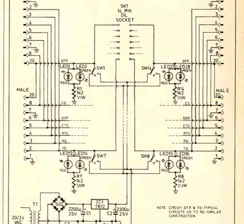
For DTE devices set all lines in centre position, set CD line on both sides to +12 V, bridge TD to RD opposite side on both sides, bridge RTS to CTS opposite side on both sides, bridge DSR to DTR opposite side on both sides.
