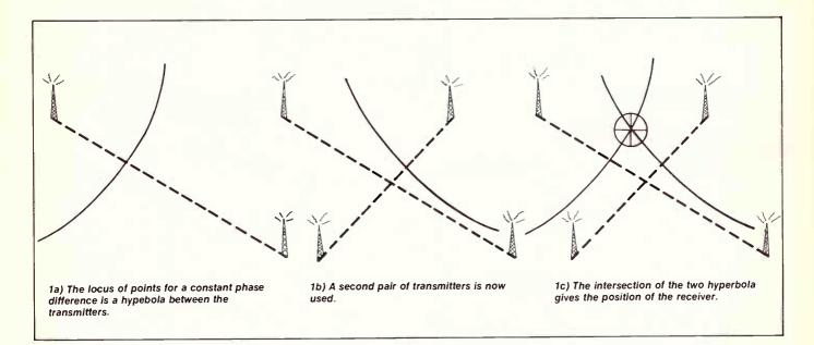
tersection of the two hyperbolae. The more transmitter pairs used the more accurate the position.
