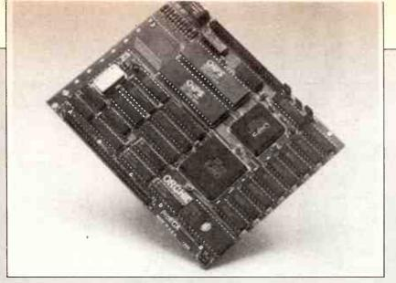
advanced processor like the 80286 or 386 running at high speed. A typical example is Orchid's Jet386 card which gives a claimed speed three times that of a standard AT.
