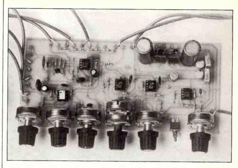
the component overlay. Do not as yet insert the IC's themselves. Insert and solder in the pc mount pots and switch, making sure that they sit firmly and parallel to the pc board. The +/- 12 V regulators (IC6 and 7) are the final components to solder in, note the orientation on the overlay.
