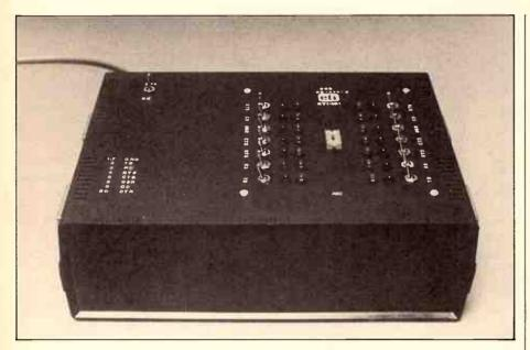
THE RS-232-C STANDARD greatly simplifies the interconnection of digital devices. When something goes wrong at an RS-232-C interface, the 25 signal lines and two equipment configurations — Data Terminal Equipment (DTE) and Datacircuit Terminating Equipment (DCE) — can easily confuse the trouble shooter. The RS-232-C BreakOut Box (BOB) is a piece of test equipment used to simplify RS-232-C trouble shooting.
