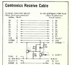
\*1 — The IBM-PC Strobe pin (and Autofeed, Init, and Select) are bidirectional because they have an open collector driver. In the read mode the "write" (see below) must be +5v thus STROBE is pulled high by the 4.7 k resistor. Any other device connected to STROBE may write a +5v at no current drain or a OV if it can sink 1 mA through the 4.7 k resistor. The STROBE pin is used for reading AND writing to the flipflop formed from Q1 & Q2.
