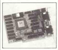
The picture shows a highly integrated multifunction card from NEC. It has three video modes, extra memory and a printer port.
