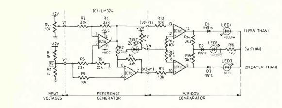
Figure 6: A window comparator with a reference generator
