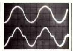
Top: Main Amp Output (VA). Bottom: Error Amp Output ( $\sqrt{B}$ ) with boot stripping.
