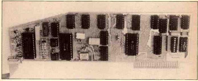
The plug-in card. The ribbon cable at left connects to the isolation box.
