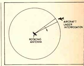
Figure 2 Transmitted pulses will only "paint" the aircraft whilst it remains in the main beam of the air traffic control radar. With a beam width of 1.5°, a rota-tional speed of 6 rpm and a PRF of 250 pps an air-craft would be intercepted by about 10 pulses. In practice, the choice of PRF is nearly always a compromise which is dictated by operational requirements and limitations of technology.
