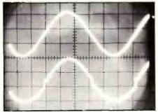
Top: Main Amp Output. Bottom: Error Amp Output, Notice that the error Amp signal at crossover is 10 times larger.
