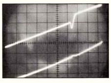
Top: Main Amp Output. Bottom: Error Amp Output expanded to see Crossover Region. The kink in the main output is clearly seen, whilst the "anti-kink" is seen to be 10 times larger.
