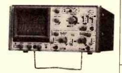
Geoff chose the Goodwill GOS522 as outstanding value in a 20MHz scope. It offers dual channel operation with a big 150mm screen and a 20nS max sweep for high precision. Alternate triggering greatly simplifies the knob-tiddling to get a stable display on both channels. Ask Geoff for a demo, you'll be delighted with the performance!
