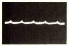
Distortion Waveform with Feed Forward 0.025% (1 kHz) (Output of Distortion Analyser).
