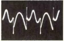
Distortion Waveform with no Feed Forward 0.6% (1kHz) (Output of Distortion Analyser).
