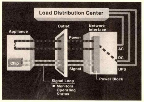
Once an appliance identifies itself and signals for energy, it is supplied and its use is continually monitored. AC or DC may be called up by the appliance. A low-voltage uninterruptable power supply (UPS) maintains signalling operations should main power fail. In the case of gas interface monitors pressure and flow.
