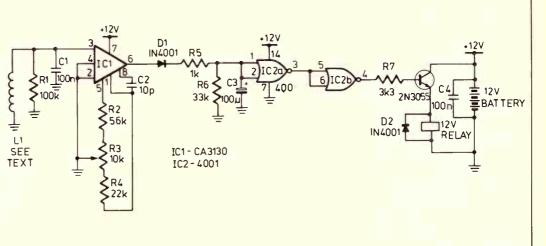
on for a suitable time. IC2 acts as a buffer to prevent C3 discharging through the transistor. R3 is a sensitivity control. adjusting the offset voltage of IC1 so that the small input voltage will trigger the circuit.
