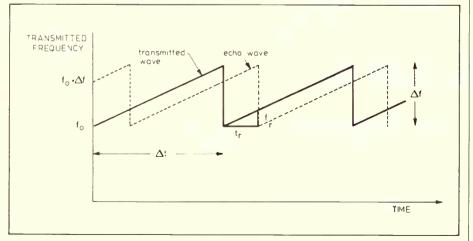
Figure 1 The sawtooth frequency modulation of a CW of fundamental frequency  $f_{c}$  by 2.4 in time  $\Delta t$  provides range information from a fixed target. The echo signal received will lag the transmitter signal by  $t_{c}$  and so it the frequency difference  $t_{c}$  is measured at this point the range may be determined and displayed.
