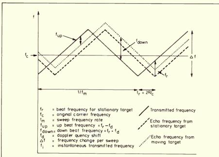
**Figure 3** FM-CW may be used to determine the range of a moving target. The CW of frequency f is modulated in frequency over a period  $1/f_m$ . On the up-sweep the echo signal range frequency f, will be reduced by the Doppler shift  $f_d$  whilst on the down-swing the echo frequency will be increased by  $f_d$ . The range may then be dedweed.
