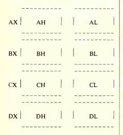
Any of these registers can be altered by a wide variety of instructions to do things like move data to and from registers into memory, move data from one register to another, add the contents of one to the contents of another, and so on. In a sense, these registers are like variables in BASIC — each of them will have a particular meaning in terms of the section of program you are writing.
