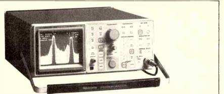
Computer control allows sophisticated ergonomics. Primary functions are accessed via dedicated keys on the front panel, and less important ones via menu driven displays. If the unit needs to be customised further, the operator can use the control programme that allows one to reduce oft repeated sequences to single key stroke functions. *R.I. No. 133*
