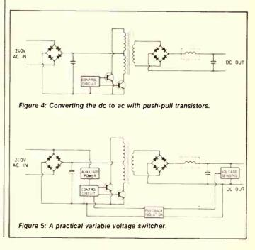
with the primary (or secondary for that matter). At the same time as output current is flowing in S1 energy is being stored in the main transformer inductance (referred to as the magnetising inductance). When the main transistor turns off the voltage its collector rises to some hundreds of volts above the 340 volt supply and at the same time the voltage at the output of S1 reverses.
