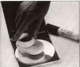
Trackmate, whose products are distributed by Amaray of Sydney, has reached an agreement with Eastman Kodak to supply a special cleaning solution for CDs. This Kodak solution is packaged in the open, and applied to the disc via a patented brush.
