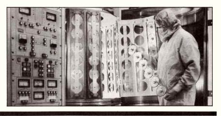
The vacuum metalising process which deposits a film of aluminium on the disc substrate.
