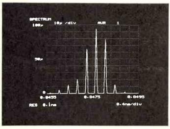
Figure 1. 0.85 µm LD spectrum.
