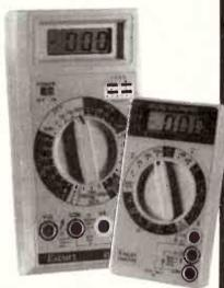
Measures only 126mm x 70mm x 24mm yet incorporates full 31/4 digit multimeter including a continuity buzzer. Single rotary switch for fast convenient operation. Checks diodes too. Measures Vdc from 200mV to 1000V, Vac 200 and 750V, Adc from 200uA to 2A. Ohms from 200ohm to 2Meg. Special 1.5V battery test range with 1mV resolution and a continuity range which beeps when resistance is below 100ohm. Bright yellow case so you can't mislay it!! EDM-70B \$64.40 inc. tax (\$55.52 ex tax).
