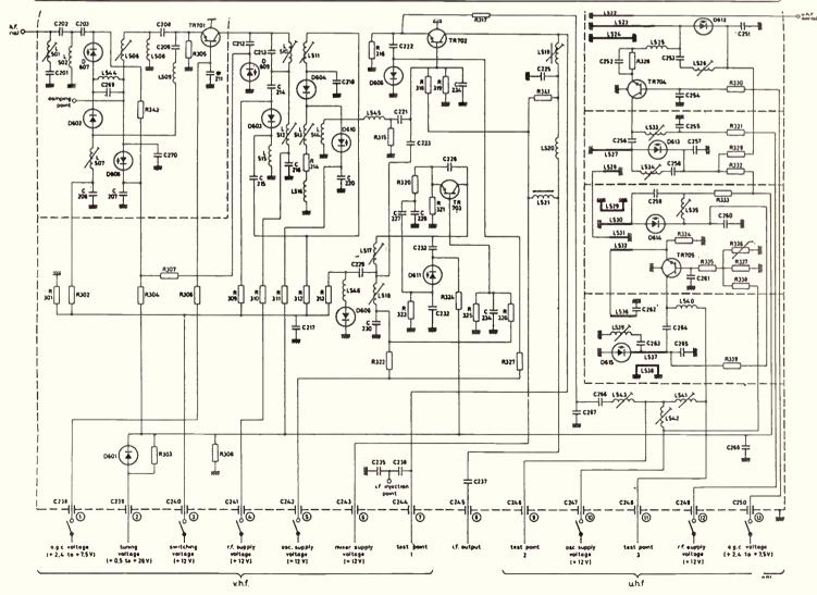
Figure 1. ELC2060 schematic.
