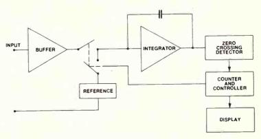
Figure 2. Block diagram of multislope approximation architecture.
