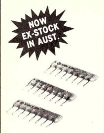
PRAGUE ECONOLINE thick-film resistor networks include multiple isolated resistors, pull-up/pull-down and interface networks in low-profile-6-pin, 8-pin or 10-pin conforma-coated single in-line packages (SIPs). Pins are set on 0.100-in. centers. Packages are 0.200-in. high.
