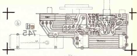
check with a multimeter will indicate the difference. The main coil (largest winding) will measure in the vicinity of 7 to 15 ohms. The secondary will be something like 0.5 to 2 ohms.
