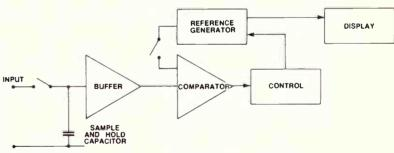
Figure 1. Block diagram of successive approximation architecture.
