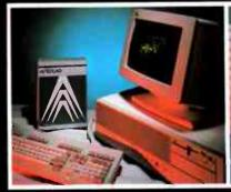
The NCR PC8 Advanced Technology (AT) PC is an ideal CAD workstation with its 8 MHz 80286 processor and native 640 by 400 colour graphics capability
