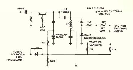
Figure 2. Tuning and band switching methods.
