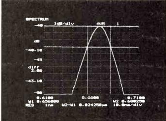
Figure 2. 0.66 µm LED spectrum.
