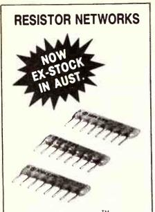
SPRAGUE ECONOLINE<sup>TM</sup> thick-film resistor networks include multiple isolated resistors, pull-up/pull-down and interface networks in low- profile-6-pin, 8-pin or 10-pin conforma-coated single in-line packages (SIPs). Pins are set on 0.100-in. centers. Packages are 0.200-in. high.
