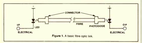
n a communications sense, fibre optics is the transmission of information by means of optical energy confined and guided by optical waveguides.
