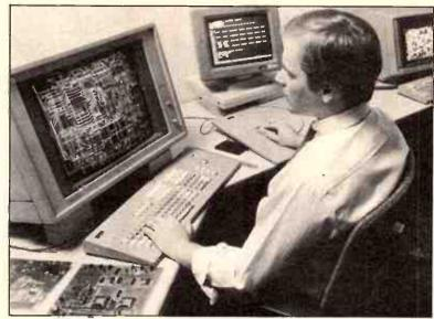
simulation programs on the engineering workstation itself. Any problems can be rectified by altering the schematics and testing the logic again until the desired results are obtained.
