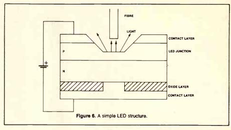
As with most simple things there are problems, foremost of which is that the light has difficulty getting out of the junction area. Reabsorption of the light by the overlaying material makes it necessary to use a heterojunction configuration (see Figure 7).
