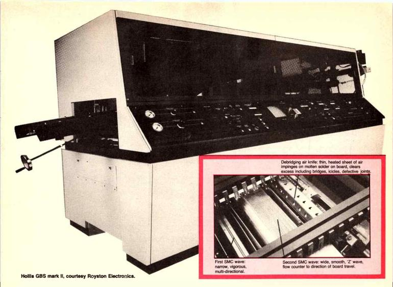
per 1000 joints at the test facility. The boards manufactured there had no solder mask and component leads were left long and straight. Large ground plane areas with no solder drain capability, plus the absence of protective solder masking, created another defect: icicles. Taken altogether, the number of defects averaged 4.9/1000 joints.
