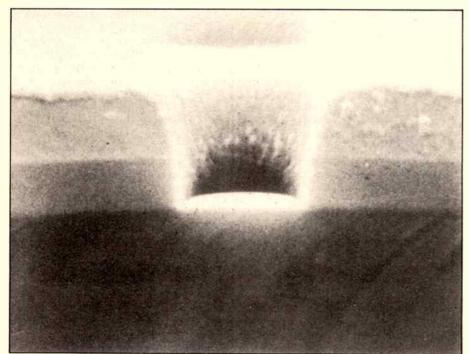
Contact hole in SiO<sub>2</sub> showing sloped walls using controlled photoresist erosion (Plasma Technology).
