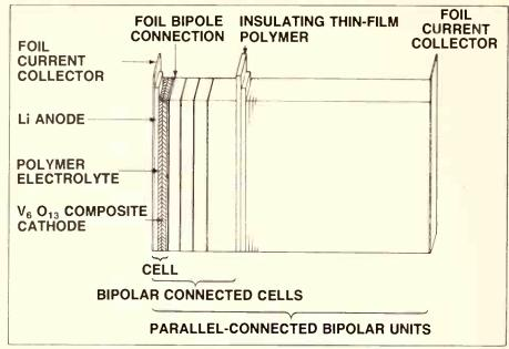
solid-state polymer electrolyte perhaps using various materials and construction technologies for different applications, holds out one of the most versatile and exciting prospects for battery development this century.
