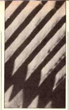
One hundred nanometre optical structures in semi-insulating gallium arsenide with gold/platinum mask using silicon tetrachloride chemistry (Plasma Technology).
