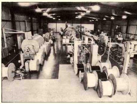
The manufacture of fibre optic cable at Olex, Melbourne.
