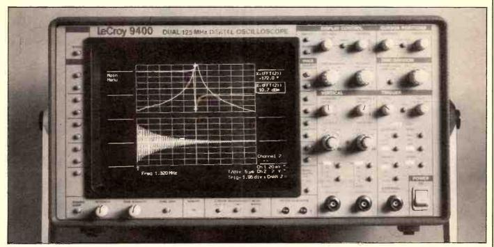
ETP Oxford has just released an FFT spectrum analysis package for the LeCroy 9400 digital oscilloscope. The screen shows a logarithmic amplitude against phase transform of the bottom trace, a 50 μs damped sine wave.
