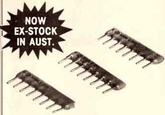
SPRAGUE ECONOLINE<sup>™</sup> thick-film resistor networks include multiple isolated resistors, pull-up/pull-down and interface networks in low-profile-6-pin, 8-pin or 10-pin conforma-coated single in-line packages (SIPs). Pins are set on 0.100-in. centers. Packages are 0.200-in. high.
