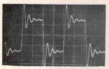
(b) 8 ohm and 2 uF parallel load
