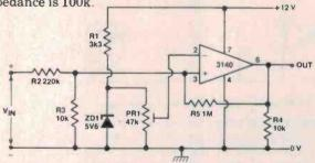
Figure 6. High value (0 — 130 V) regenerative over-voltage switch.
