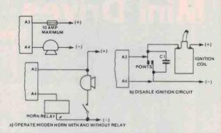
Figure 6. A3 and A4 alarm relay contact; giving extra protection.
