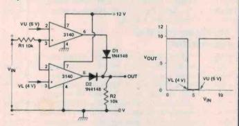
Figure 8. A voltage window comparator or discriminator. The output goes high when VIn goes outside of the VL or VU limits.
