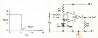
Figure 1. Basic op-amp comparator that functions as an under-voltage switch: the output is high when Vin is below Vref.
