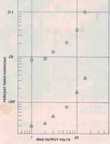
Figure 13. 1 kHz third harmonic distortion 0 — Figure 2 (conventional amplifier);
