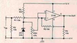
Figure 4. Variable over-voltage switch with regenerative feedback.
