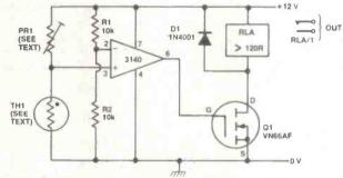
Figure 13. Precision under-temperature switch with VFET/relay output.
