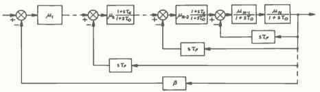
Figure 5. Block diagram of an NDFL amplifier.
