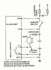
Figure 2. Basic alarm system, positive ground.
