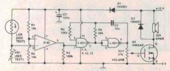
Figure 14. Light-operated switch with monotone alarm output.
