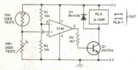
Figure 12. Precision over-temperature switch with transistor/relay output.
