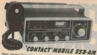
New stocks have just arrived of our beefed up version. Now puts 6.5 watts AM into aerial. Fully synthesized. 23 Ch AM plus upper and lower sideband. Dual conversion AM power and S meter. P.A. facility, xtal lattice filter. For Novice or Ham use. 12 volt operation.
