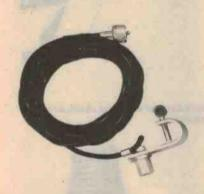
Fig. 12. A luggage rack or ski-bar mount. These are inexpensive, simple and quick to install. They are also suitable for wing-mirror mounts.
