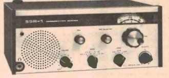
The SSR-1 Receiver provides precision tuning over the short wave spectrum of 0.5 to 30 MHz with capability of reception of a-m (amplitude modulated), cw (continuous wave) and ssb (upper and lower single side band) signals.
