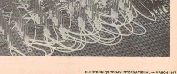
The disadvantage with wire wrapping is the need for special IC sockets. They are twice as expensive as ordinary sockets and increase the volume occupied by assembly. Not evident in this photo is the squareness of the socket's pins or their sharp corners. The pins come gold plated or tin plated, with the gold type more expensive.
