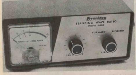
A typical SWR bridge. Similar units are available at most retail outlets. Note on the right hand side the Forward and Reflected switch. When set on the Forward mode you adjust the sensitivity control (for different power inputs) to give full scale deflection. Then, still transmitting, switch to the Reflected position and read the Standing Wave Ratio.
