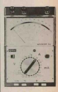
The push-button polarityreversal switch of the Unigor 3n simplifies the testing of semiconductors.
