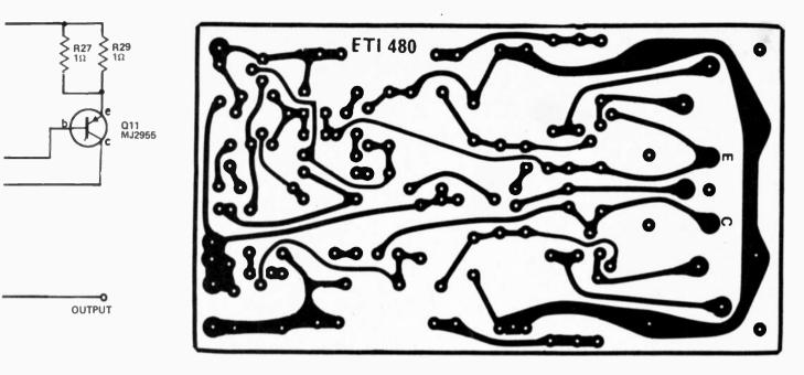
Fig. 4. Printed circuit layout of the amplifier. Full size 140mm x 76mm.
