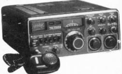
KYOKUTO 2M FM 15 W output transceivers with digital read-out and crystal synthesized PLL circuitry now with 800 transmit and 1000 receive channels 5 KHz apart, covers all of 144-148 MHz, receive to 149 MHz. No more crystals to buy. Includes simplex, repeater and anti-repeater operation
