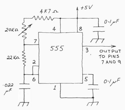
Fig. 2. Circuit diagram of the external oscillator.
