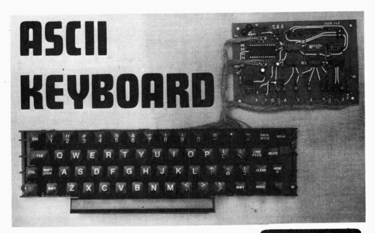
This simple and inexpensive keyboard encoder gives full ASCII output, has keyrollover facility and can be used with almost any keyboard.
