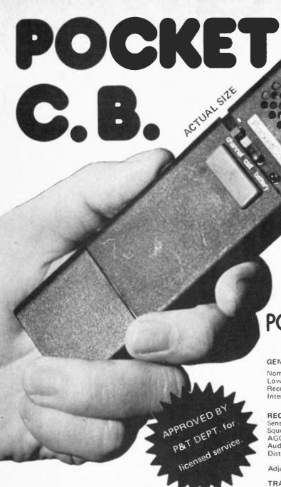
THE POCKETCOM is a 27240 kHz battery-operated transceiver suitable for two-way communication over a few kilometres (on a line-of-sight link with a clear channel). If a second channel is permitted you can plug in a crystal and switch to channel B.
