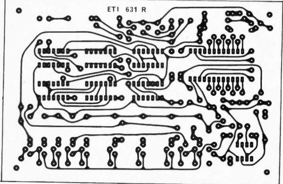
Fig.4. Printed circuit layout(both sides) Full size 150 x 100 mm.
