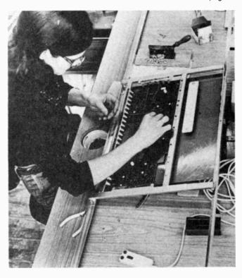
The slide projector is synchronised with a system of small component trays which run below the assembly desk.
