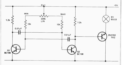
A simple and inexpensive unit for reducing the brilliance of a lamp and at the same time reducing the current drain, thus increasing battery life considerably. A power saving does not happen by merely inserting a resistor in series with the bulb, hence the reason for the above circuit.
