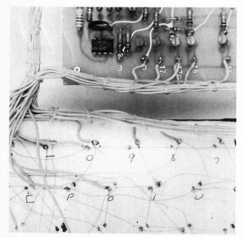
Rear of the keyboard showing how the inter conections are made.
