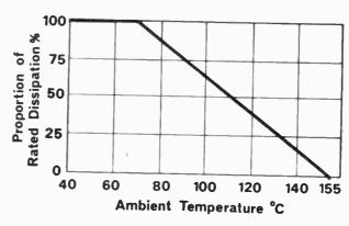
Fig. 2. Derating curve for common metal film resistors. It also applies to metal oxide film resdistors up to 1 W rating.
