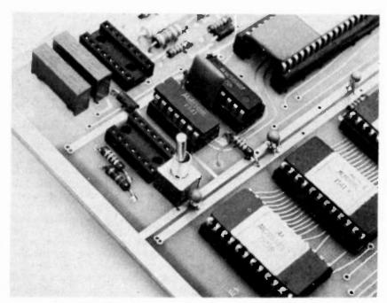
How the double pole switch is mounted on the MEK board.
