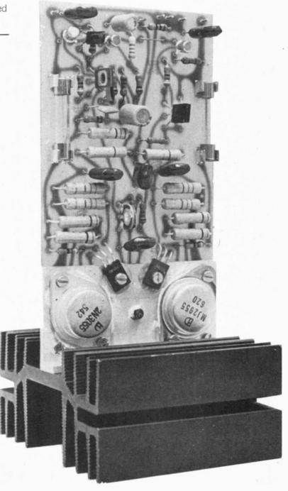
The screws holding the 2N3055/MJ 2955 should also be insulated where they pass through the heatsink bracket. The BD 139 and BD 140 do not need any insulation other than the mica, provided 6 BA (or 3 mm) screws are used. In the 100 W version the addition transistors are mounted on the heatsink bracket outside the pc board area.
