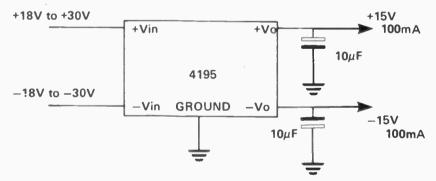
When experimenting with operational amplifiers and other circuits, one often requires balanced positive and negative power supplies of about ±15 V. One can, of course, employ two separate stabiliser circuits employing an integrated circuit voltage regulator.
