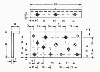
Fig. 9. Heatsink bracket for the 50 W module.
