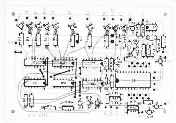
Fig.2. Component overlay of the encoder.
