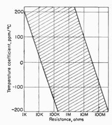
Fig. 1. Hange of temperature coefficients available for various values of metal film resistors having controlled TC characteristics.
