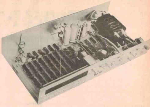
pulses or level changes, into the respective sockets. A voltage change from 0V to 3V (or +3V to 0V) is all that is necessary although up to  $\mp$  100V can be used. For accurate timing the pulse should have a rise time of less than 1  $\mu$ s. For measuring single pulses, both inputs can be paralleled and starting and finishing on opposite edges. If it is a repetitive pulse chain the unit will time the first pulse after the release of the reset button.
