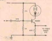
FIGURE 8. Current Limiting and Short Protection
