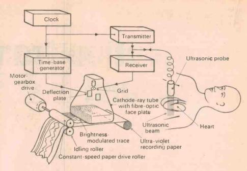
Time-position recording system based on the B-scope display, shown in use for echocardiography. The fibre-optic face plate of the cathode-ray tube collects enough light to produce a self-developing trace on ultra-violet recording paper.
