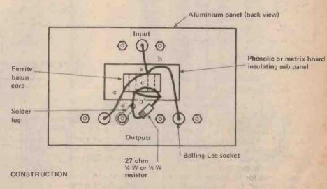
Fig. 9. a) Circuit of transformer-type splitter.
