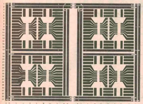
Fig. 2. Above: This is the track pattern for the ZB-B-IC used in this series. Note the wire links which need to be made in order more easily facilitate application.
