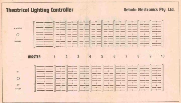
Fig. 1. The front panel artwork for the 10 way control desk. Full size is 440 mm x 250 mm.
