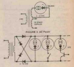
FIGURE 4. Unfiltered DC Power
