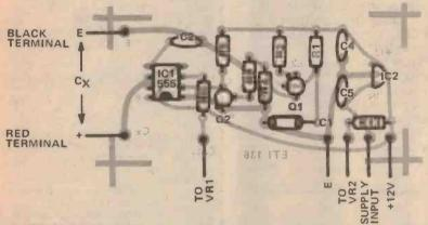
R7-R12 and C3 are mounted on the rear of the range switch
