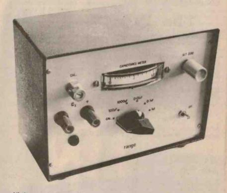
All the range resistors, R7 to R11, and R12 are high tolerance 1% or 2% resistors accurately measured to be within the tolerance required. If only 5% or 10% accuracy of capacitance
