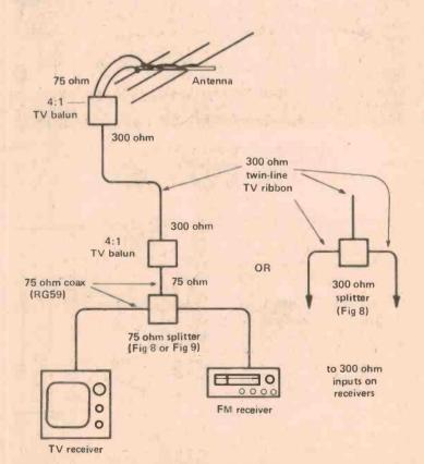
Fig. 10. Feedline and splitter systems installation.
