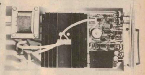
If the dimmer is connected up to a reasonably heavy load and adjusted for about 1/3 level it will probably be found that with RV3 at one end the light level is not stable and tends to flash. This is caused by the sync pulse occuring after the end of the half cycle and the trigger pulses from the previous half cycle triggering the next. The trim potentiometer RV3 should be turned back about ¼ turn from the position at which this effect stops.
