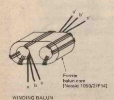
Fig. 7. Construction of 1:1 balun transformer.
