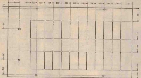
Fig. 2. The mechanical dimensions for the front panel.
