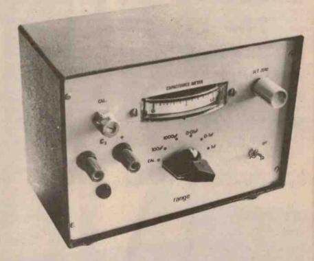
All the range resistors, R7 to R11, and R12 are high tolerance 1% or 2% resistors accurately measured to be within the tolerance required. If only 5% or 10% accuracy of capacitance
