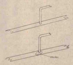
Fig.1. The method of attaching components to the Blob Boards. The 'leg' can be simply bent to one side and then soldered 'blobed' over the lead to hold it. Since the boards are tinned, and the leg ought to be, a sound joint is usually obtained.
