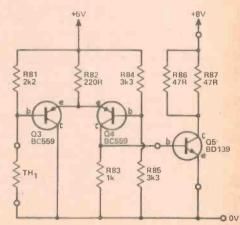
Fig. 1. The circuit diagram of the oven circuit
