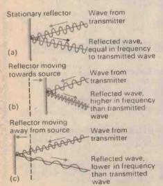
The Doppler effect occurs when a wave is reflected from a moving surface, giving an upward or downward 'shift' in frequency as in (b) and (c).
