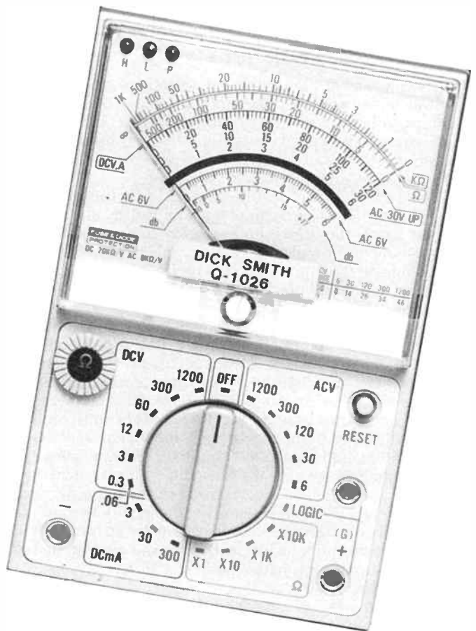
Today's equivalent of the "five bob" multimeter. Dick Smith's Q-1026 is a low-cost analogue meter with mirror scale for improved reading accuracy. It features 20 ranges and overload protection.
