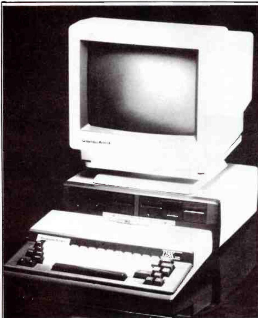
The Microbee Premium Series is available in the same formats as the 'standard' series. For review, we obtained a 64K system with twin 3.5" disk drives, the latter being housed side by side in the twin-drive box that take 5.25" drives, as shown here. Both colour and monochrome monitors are available to team with the computer.
