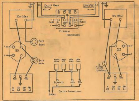
Wiring diagram of the power supply, showing A.C. switch connections.
