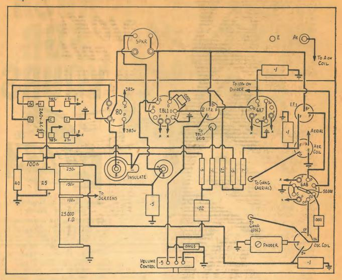
The wiring diagram shows the simplicity of the set's construction. The five resistors near the centre may be mounted on an insulated panel.
