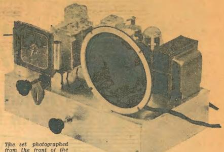
The set photographed from the front of the chassis. The speaker plugs into the rear of the chassis.
