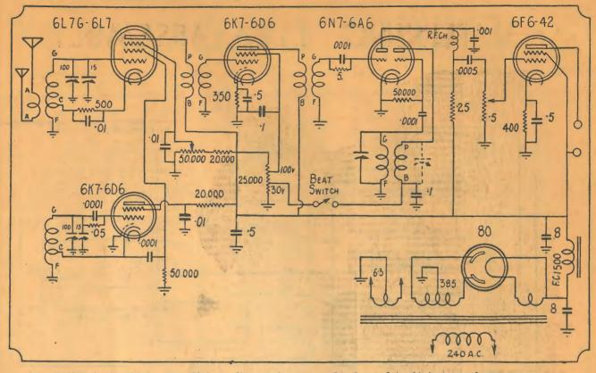
Here is the circuit. The .0005 coupling condenser may be changed to .01 for normal response.
