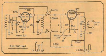
Circuit of the exciter unit. Note the shield position and switch connections.
