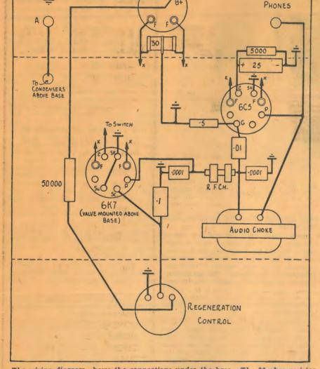
The wiring diagram shows the connections under the base. The 30 ohm resistor is omitted in the battery version, connection to the chassis being made from one of the filament terminals of the 6K7.
