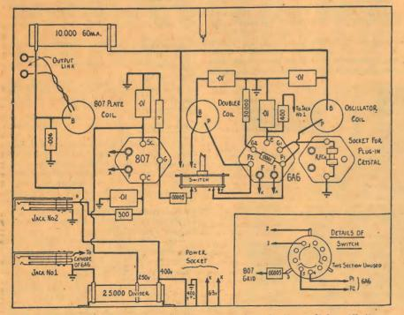
Wiring diagram of the exciter. Note connections to the switch. All these wiring diagrams are to scale.
