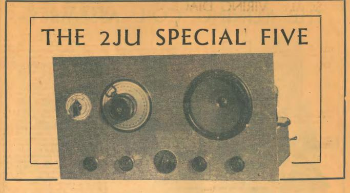
A front view of the set. The small pointer and scale in the centre is the oscillator band-setter. Any good panelmounting dial may be used.
