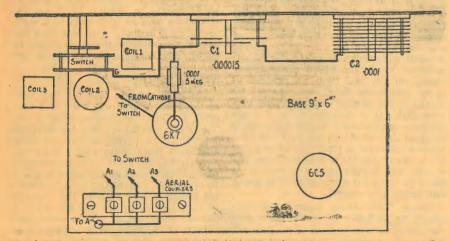
Here is a scale drawing of the components above the base. Connections are also shown in this diagram.
