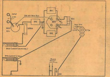
Wiring diagram of the final amplifier.
