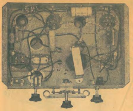
This picture shows the wiring beneath the chassis. Note the audio transformer.
