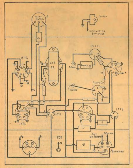
The wiring diagram gives a complete picture of the connections. The bias battery stands above the chassis. The positive terminal connects to the chassis through a solder lug bolted to the frame of the gang condenser.
