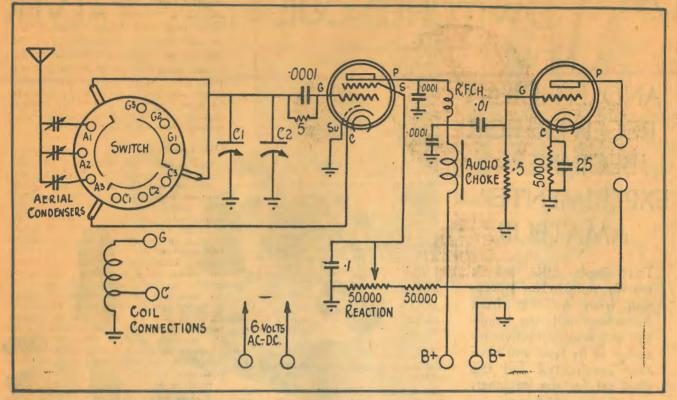
The circuit. A switch should be included between B minus and the chassis, or a lead to the B battery removed when the set is not being used.
