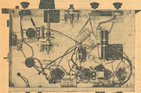
Under the chassis. Aerial connections may be seen running through the chassis at the bottom left-hand corner.
