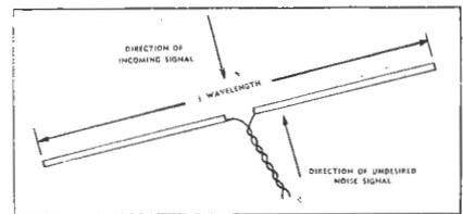
Fig. 5.—Signal response of a half-wave dipole.
