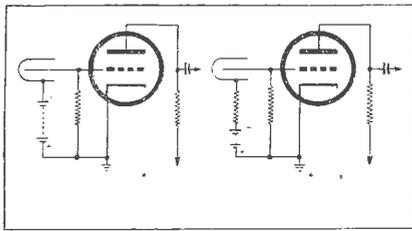
Fig. 4.—Two types of quenching circuits—on the left the Neher-Pickering circuit and on the right the Neher-Harper circuit.
