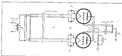
Fig. 5.—The tuned-grid tuned-cathode push pull oscillator.
