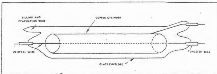
Fig. 2.—The Geiger counter tube as developed by Geiger and Rutherford.
