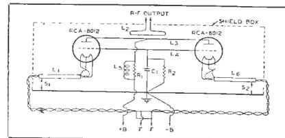
Fig. 6.—A parallel-plate oscillator using two 8012's.
