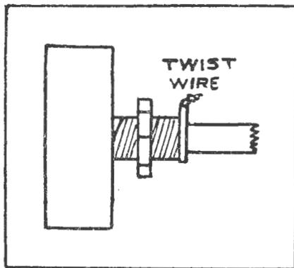
Twisting a piece of wire around the volume control shaft will often cure a "noisy" control.
