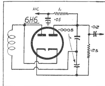
This voltage doubler detector circuit give increased signal and AVC voltages.
