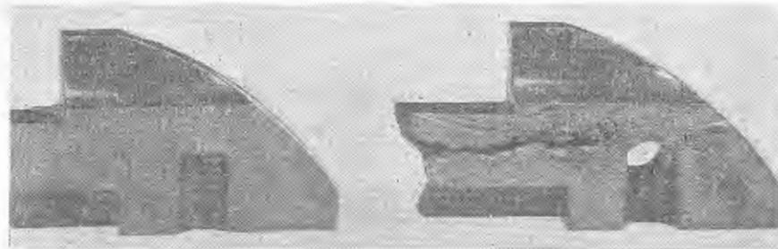
This photograph of bakelite moulding samples with and without H.F. preheat, clearly illustrates the effectiveness of this method of heating.
