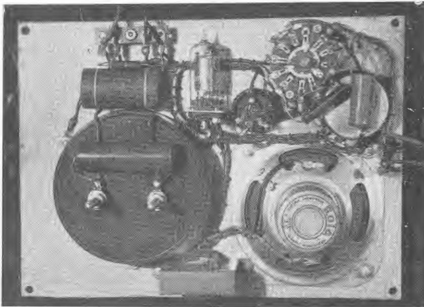
A close-up of the completed wiring. The various leads are tied together for neatness, and are made as short and direct as possible.
