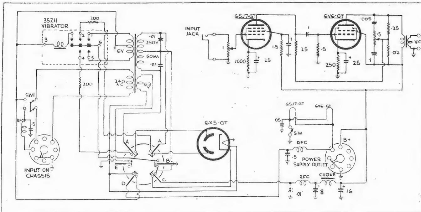
This is the circuit for mains or vibrator operation. Although the switch connections may appear complicated, they are simple enough if traced out in a logical order.
