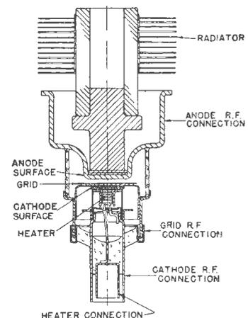
Fig. 3.—A sectional drawing of the 2C39.
