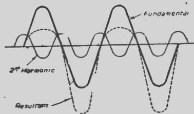
Fig. 8.—When anode current flows it can produce an inverse form of second harmonic distortion.
