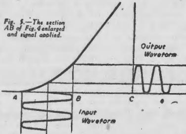
Fig. 5.—The section AB of Fig. 4 enlarged and signal applied.
