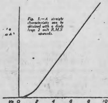
Fig. 3.—A straight characteristic can be obtained with a diode from 2 volt R.M.S upwards.
