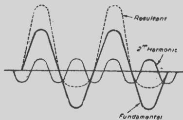
Fig. 7.—Combining a fundamental with its second harmonic produces the broken curve.
