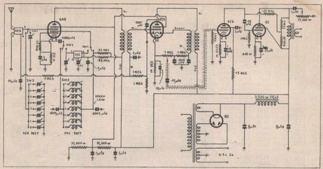
Circuit of a modern 4/5 dual-wave superhet with push-button tuning, designed around the Crown FK/8 Foundation Kit. Though shown separately above, the padder is incorporated in the D-2 unit. The grid lead of the first i.f., labelled "B" above, is black.
