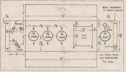
Dimensions for stamping and drilling the sprayed steel chassis are given in this sketch.
