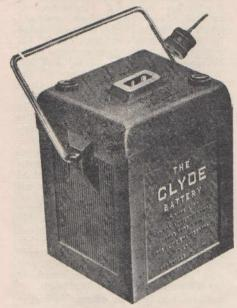
two-pin, non-reversible socket. Connection to the positive and negative terminals is made by means of leadcoated brass straps, moulded into the cover, with lugs at each end to fit over the battery terminals.
