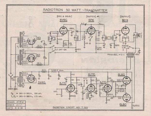
for receiving purposes, so that a pair of Radiotron 866 mercury vapour rectifiers would normally be necessary. However, as will be seen from the circuit diagram, by combining in series the outputs from two standard power packs, the required voltage is obtainable at a lower cost.
