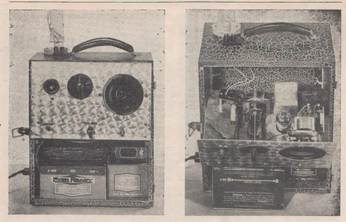
These close-up views provide all the detail necessary for the layout and assembly of the transceiver. Note the method of mounting the 76 horizontally to ensure short leads, and the tuning condenser extension shaft employed for the same purpose.
