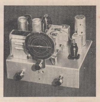
and triode audio amplifier, driving a 42 power pentode, with an 80 as rectifier.
