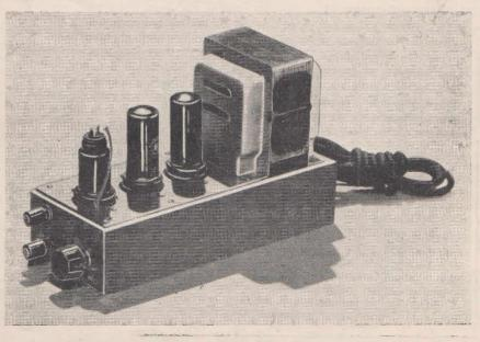
A view of the completed amplifier, with cover removed.
