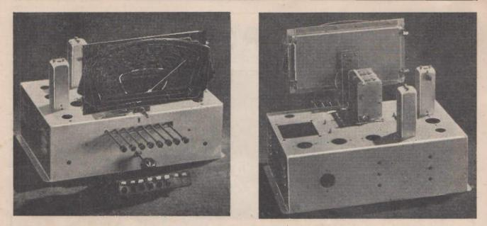
Front and rear views of the Foundation Kit mounted on the special 4/5 superhet chassis that is available from Crown distributors.
