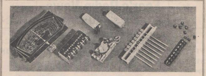
The Crown FK/8 Foundation Kit incorporates (left to right) station-calibrated full-vision dial, type PB/8 push-button unit, D-2 dual-wave unit (with permeability-tuned i.f. transformers above), push-button switch, and escutcheon with knobs.
