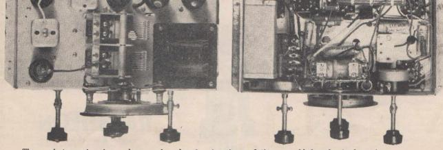
These photographs show above and under-chassis views of the assembled and wired receiver.
