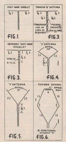
sure that the quarter-wave sections are exactly the required length. A convenient formula for calculating the length of any half-wave aerial is—  $L = M \times 1.56$ Where L equals Length in feet
