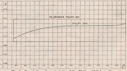
Fig. 1-Regulation characteristic of the Philips 1941 barretter.
