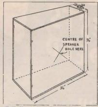
Full dimensions for making the infinite speaker baffle described in the accompanying article are given in this sketch.
