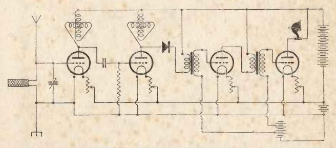
20. This combined crystal and four-valve receiver is capable of operating a loud speaker at a distance of a couple of hundred miles or more from a broadcast station. It is comparatively simple to operate, the two high-frequency valves being tuned by variometers.
