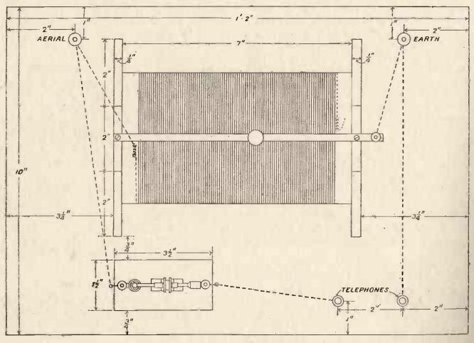
FIG. 4.—Showing lay-out and connections of crystal receiver, Model A.
