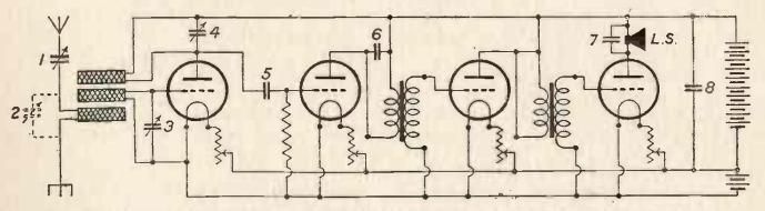
This diagram shows eight different positions in which condensers can be used with advantage in a multi-valve receiver.
