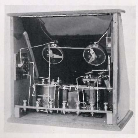
Rear view of the Two-Valve Amplifier.
