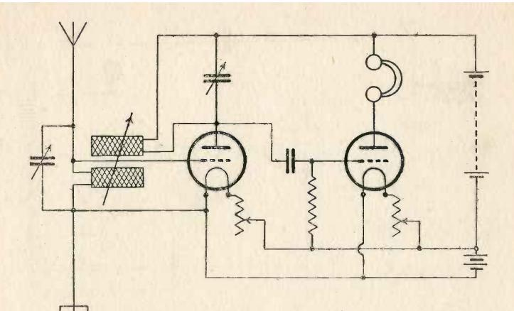
10.—This circuit is similar to the preceding one in every respect except that the anode of the high-frequency valve is here tuned by means of a plug-in coil and variable condenser. This permits of reactive coupling between the aerial and anode circuits and thus increases the sensitivity of the receiver.
