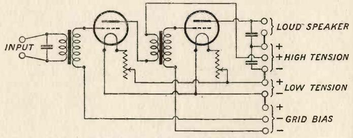
FIG. 2.—Showing the positions of the twelve terminals.
