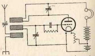
4.—A very sensitive and selective one-valve receiver with inductive coupling between aerial, grid and anode circuits.
