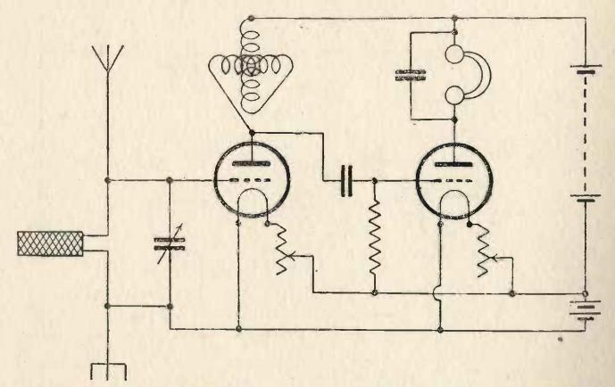
9.—A two-valve receiver in which the first valve is used as a high-frequency amplifier, and the second as a detector, the anode circuit of the former being tuned by a variometer. This receiver can bring in good broadcast signals at a distance of 100 miles.
