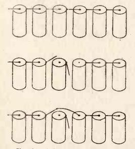
FIG. 1.—Showing the stages involved in excluding a dud cell from a battery.
