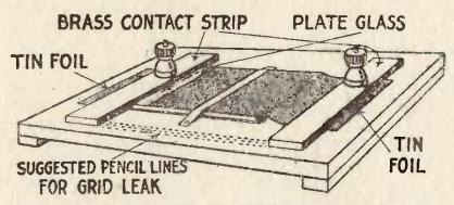
FIG. 1.—A simple type of grid condenser, with "grid leak" consisting of graphite or lead pencil lines.
