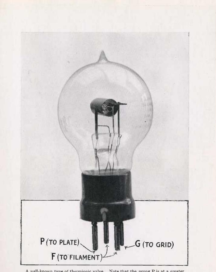
A well-known type of thermionic valve. Note that the prong P is at a greater distance than the prong G from either of the prongs which connect up the filament. This prevents the valve from being inserted wrongly in its socket.
