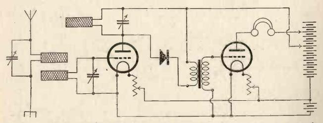
13. A crystal and two-valve receiver, in which a high degree of selectivity is obtained by coupling the aerial inductivity to the high-frequency valve. There are thus three tuned circuits, each being tuned by means of a plug-in coil and variable condenser. This receiver is particularly recommended for use in areas where bad "interference" is experienced.
