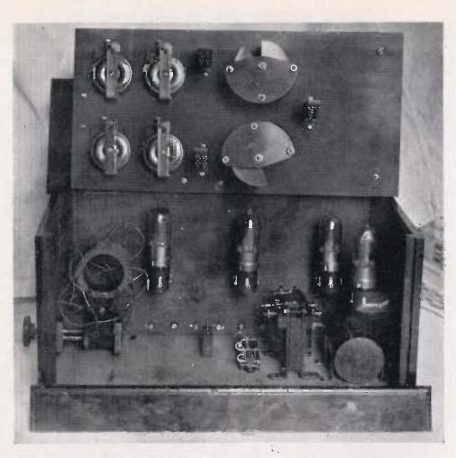
Showing positions of various components in Four-Valve Receiver before wiring up. The ebonite panel (back view) is balanced on top of cabinet. Note the battery terminals in back wall of cabinet.
