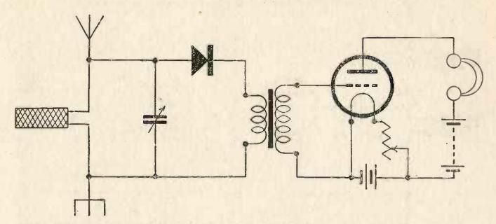
6.—A combined crystal-valve set. The valve functions as a low-frequency amplifier. Very loud signals can be obtained with this receiver at a distance of 25 to 30 miles from a broadcast station.
