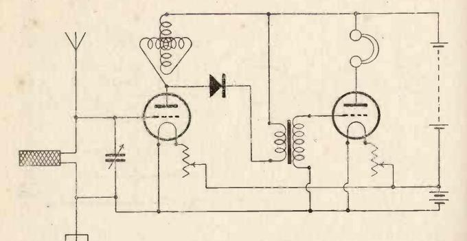
12. This circuit differs from the preceding one in that the aerial is here tuned by means of a plug-in coil and variable condenser. The same modification may, of course, be introduced in the anode circuit, as shown in next diagram.
