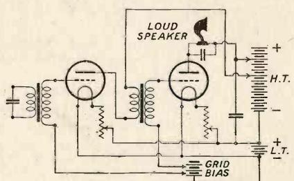
FIG. 1.—Diagram of connections of the amplifier.
