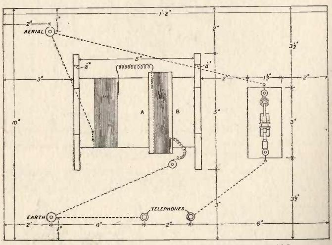
FIG. 10.-Showing lay-out and complete connections of crystal receiver, Model C.
