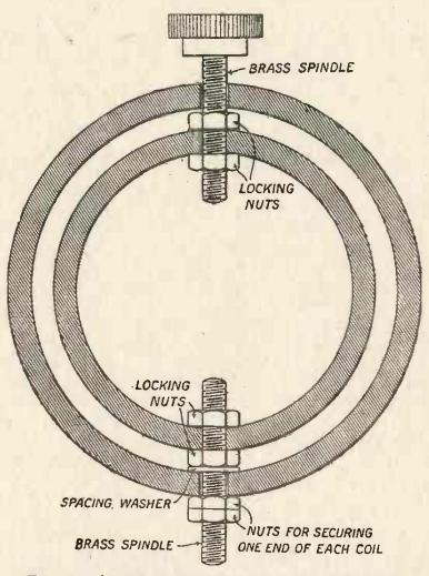
FIG. 11.—Arrangement of tubes for rotary variometer.
