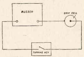
FIG. 1.—Showing connections of buzzer circuit.
