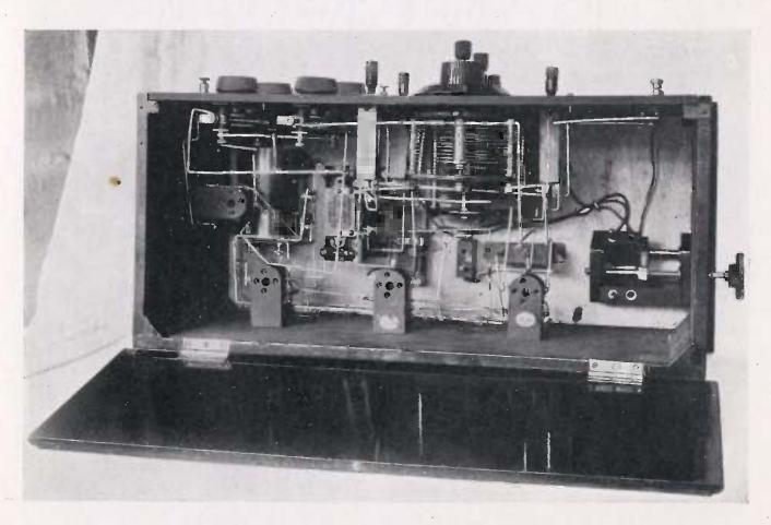
Interior view of Four-Valve All-station Receiver.
