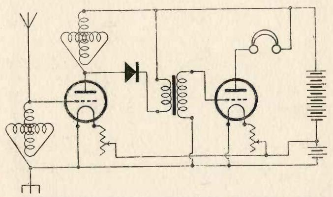
11.—A combined crystal and two-valve receiver, in which the first valve acts as a high-frequency, and the second as a low-frequency, amplifier. This is an extremely simple circuit to operate, both aerial and anode circuits being tuned by variometers.
