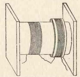
FIG. 9.—Illustrating the principle of the sliding variometer.
