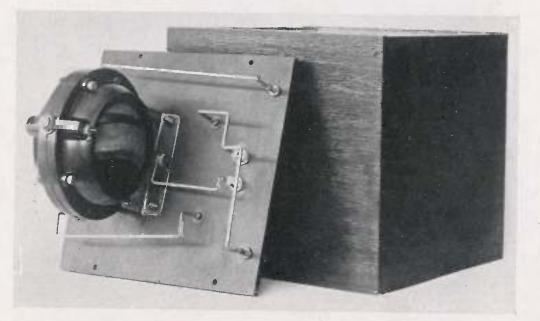
Showing internal wiring of Variometer Crystal Set.
