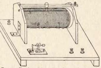
FIG. 5.—Showing slider coil and crystal mounted ready for reception. All connections are made underneath the base board.
