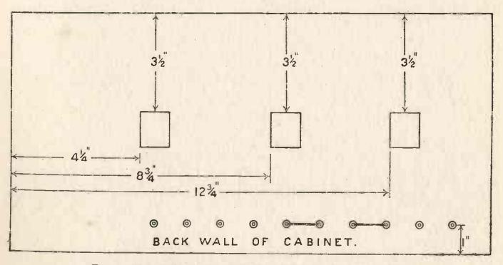
FIG. 4.—The small squares indicate the position of the valve holders.
