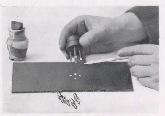
In order to ensure that the holes in the ebonite are drilled at the correct distances apart, the prongs of the holder, or of the valve itself, may be marked with white paint or chalk, and an impression of the latter reproduced on the ebonite, by contact. All traces of paint or chalk should afterwards be removed.
