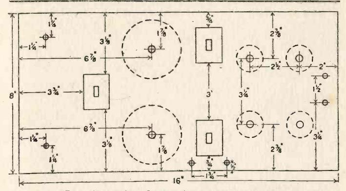
FIG. 3.-Diagram showing positions of various components on panel.
