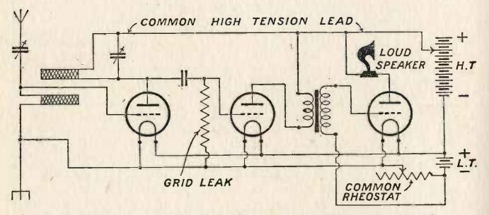
FIG. 1.—A three-valve receiver in which all filaments are controlled by the same rheostat.
