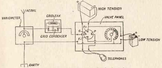
FIG. 3.-Showing lay-out and connections of single-valve receiver.
