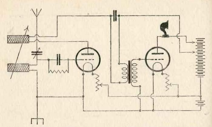
8.—A two-valve receiver in which the first valve acts as a detector, and the second as a low-frequency amplifier, reaction on the aerial being introduced from the plate of the first valve. This circuit can operate a small loud speaker within about ten miles of a broadcast station.
