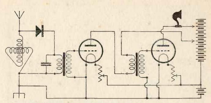
14. A very simple and reliable circuit, capable of operating a loud speaker at a distance of 25 miles from a broadcast station. The aerial is tuned by a variometer, and both valves function as low-frequency amplifiers.
