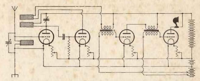
18. A four-valve, all-station receiver, in which the first valve is a high-frequency amplifier, the second a detector, and the third and fourth low-frequency amplifiers. Each low-frequency valve is provided with a separate grid bias.
