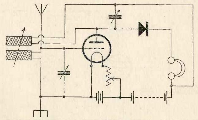
7.—A combined crystal-valve receiver, in which the valve functions as a high-frequency amplifier. The anode (*i.e.* plate) circuit of the valve is tuned by a plug-in coil and variable condenser, and maximum sensitivity is obtained by coupling the anode coil to the aerial coil. This instrument can receive broadcast signals up to 50 miles or more.
