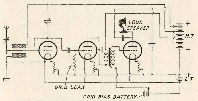
FIG. 2.—Showing how a variable grid bias can be applied to a low frequency valve.
