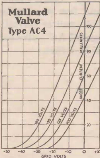
*A.C.4.* This is a dull emitter super power valve of remarkably low impedance, for use with the largest loud speakers. It is a directly heated A.C. valve for U.X. socket.
