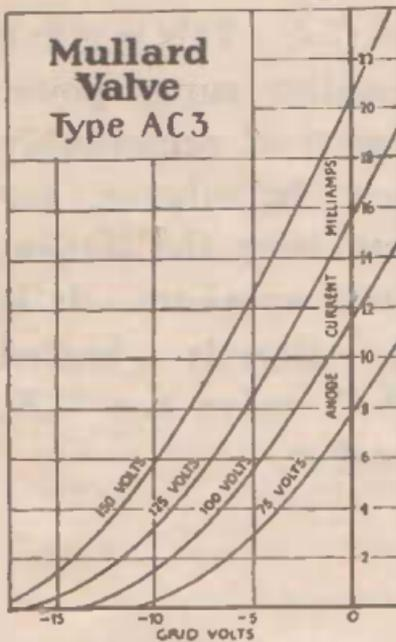
*A.C.3.* This is a radio and first stage audio dull emitter directly heated A.C. valve for U.X. socket.
