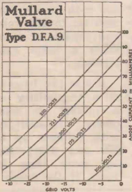
A low impedance power valve which can take its filament supply from a 6-volt accumulator or from A.C. Mains *via* a step-down transformer. It is suitable for operating a very large loud speaker.
