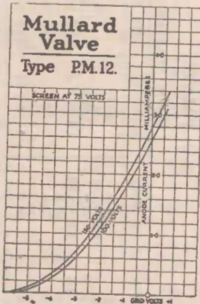
A four - electrode screened grid valve for use as a high frequency amplifier employing a high impedance anode coupling such as the tuned-anode circuit.
