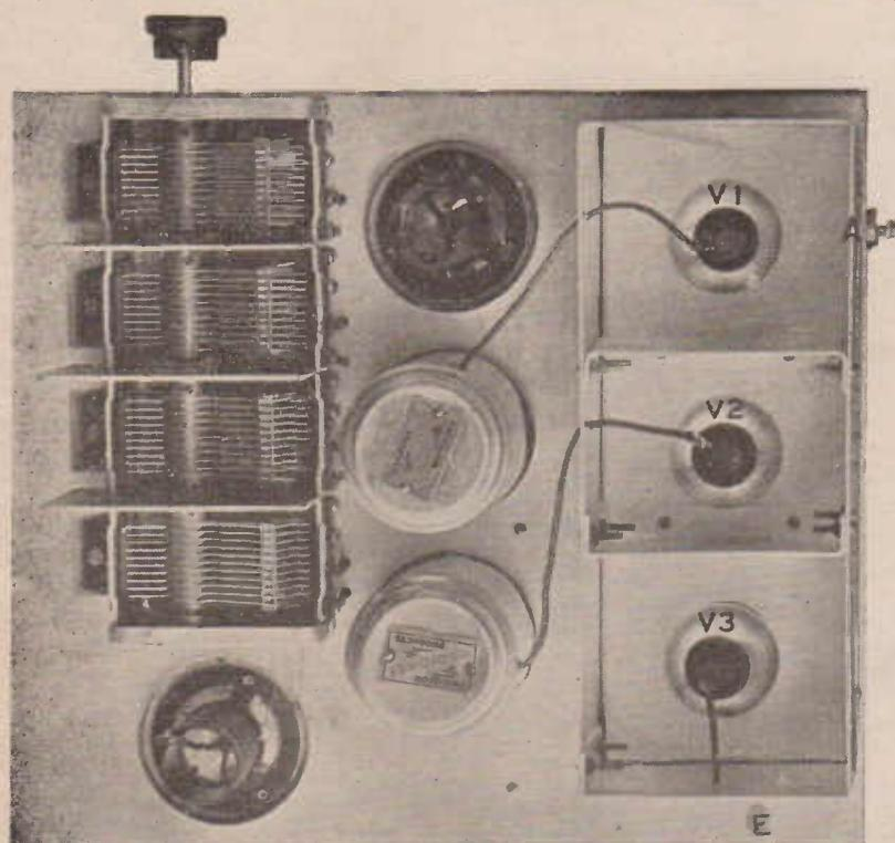
A view of a section of the receiver, showing the r.f. valves mounted in their screening boxes, and showing also two of the r.f. coils with their screens removed.
