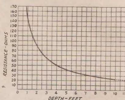
Fig. 2.—Calculated effect of depth on the resistance of a ground connection.
