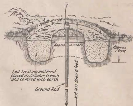
Fig. 5.—Trench method of soil treatment. Probably the most effective scheme of utilising chemicals in lower soil resistance.
