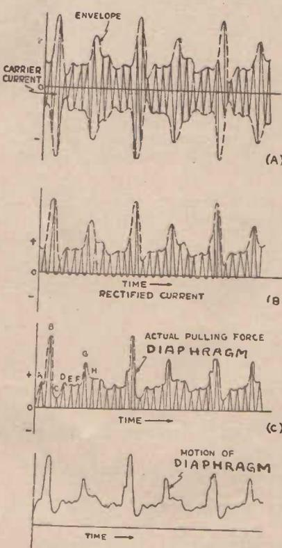
Fig. 28. The motions through which the diaphragm passes during reception of signals.
