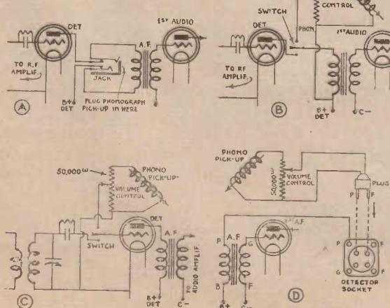
Fig. 2.—The schematic diagram showing various methods of pickup connections.
