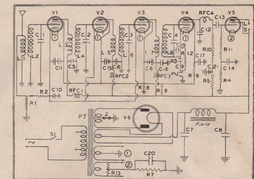
The schematic circuit diagram shows that great attention has been paid to the filtration of the r.f. and audio supply lines, so that no unwanted feedback will be present.
