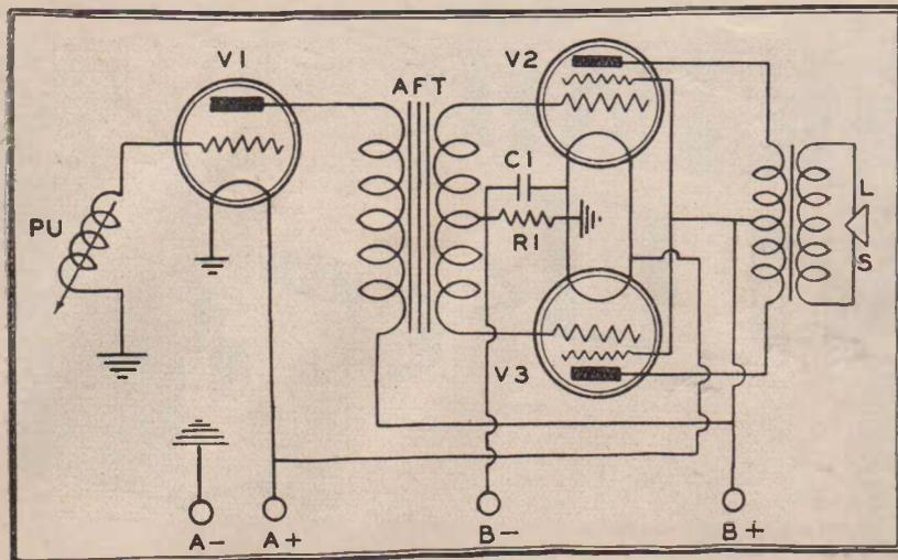
The schematic diagram of the amplifier shows that very few components are necessary for its construction.
