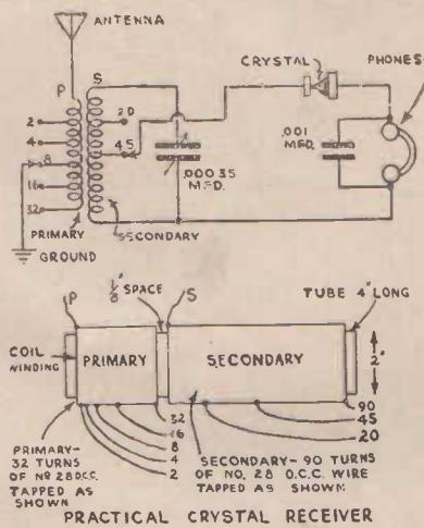
At the left, Figs. 36a and 36b show practical circuits for use with carborundum detector. The right-hand diagrams, Fig. 37, give constructional information on a cheap and simple crystal set.
