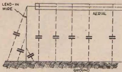
Fig. 25. The condenser effect existing between aerial and earth.
