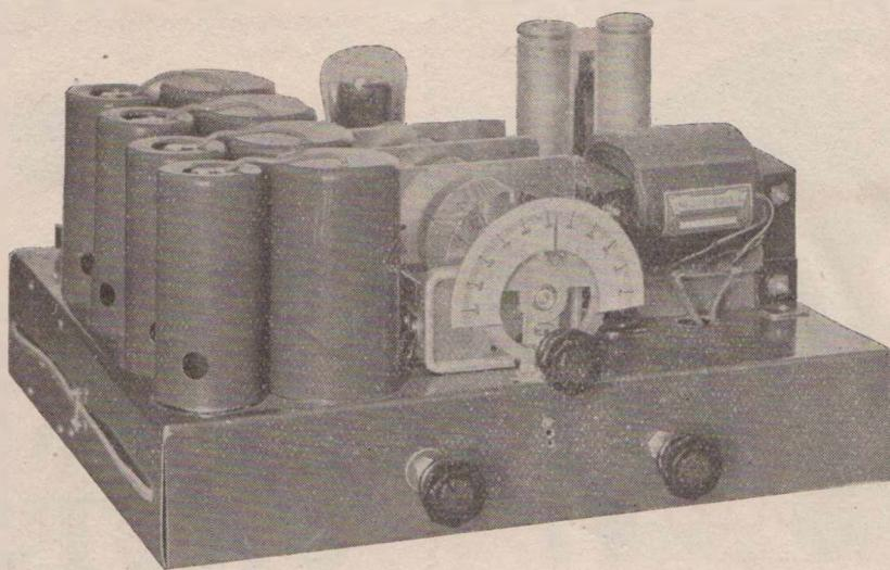
A front view of the "Compass Six" shows that despite the number of tuned circuit, the controls are kept down to three.
