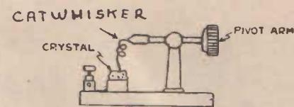
A diagrammatic view of a crystal detector. Fig. 29.
