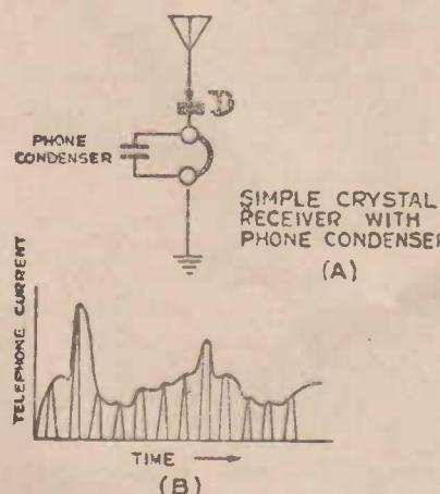
Figs. 31a and 31b illustrate the effect of connecting a condenser in parallel with the headphones.
