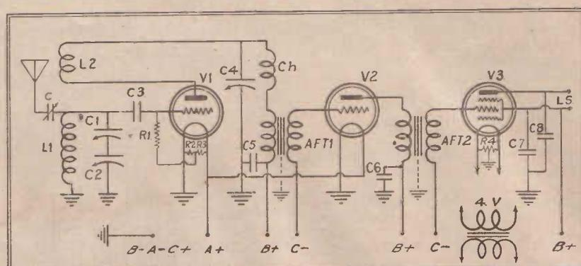
The schematic diagram of the receiver will place the experimenter in possession of full circuit details.
