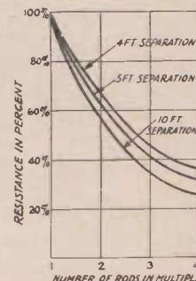
Fig. 4.—This graph shows how the resistance of a ground decreases as the number of ground rods is increased.
