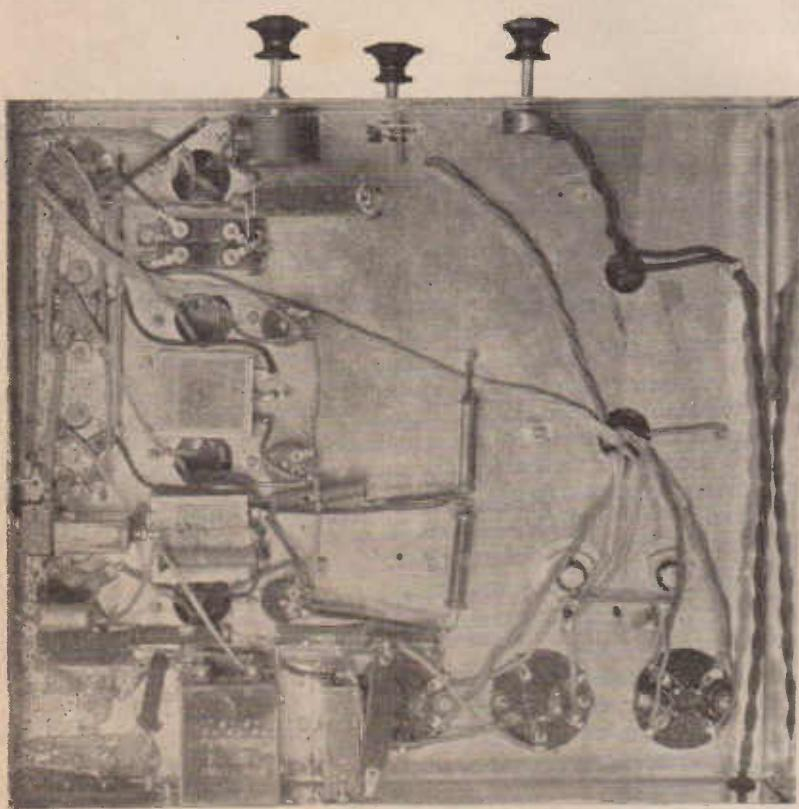
An under-chassis view gives some idea of the amount of material which is needed to build this super-receiver. Because of the necessary crowding of components at the r.f. end of the receiver it has been impossible to key-letter each part.
