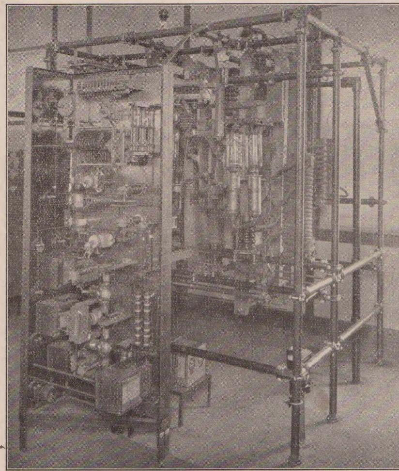
A view of the final stage of the Westinghouse Co.'s. 40 K.W. crystal controlled S. W. station W8XX.
