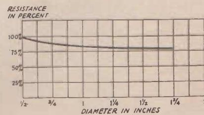
Fig. 3.—Effect of diameter of driven ground rod on ground resistance.
