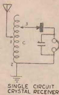
Fig. 33 illustrates one method of sharpening the tuning of a crystal set.
