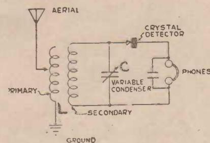
Fig. 34.—An even more selective arrangement, which is known as a "loosely coupled" circuit.
