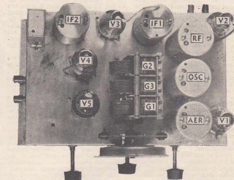
This plan view of the receiver illustrates the arrangement of parts on top of the chassis. All components are key-lettered to correspond to the written description.
