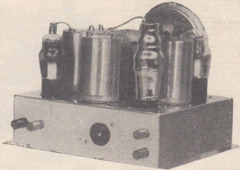
This rear view of the receiver illustrates the mounting positions of the aerial and earth terminals, the battery input socket, and the loud-speaker terminals.
