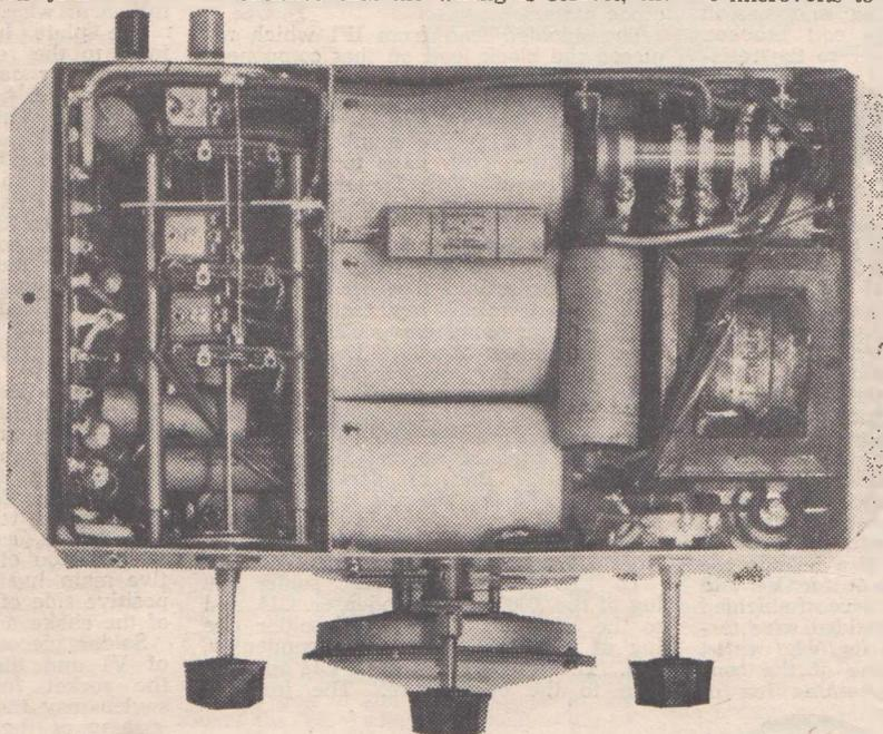
Another view of the receiver showing the wiring and arrangement of parts below the chassis.
