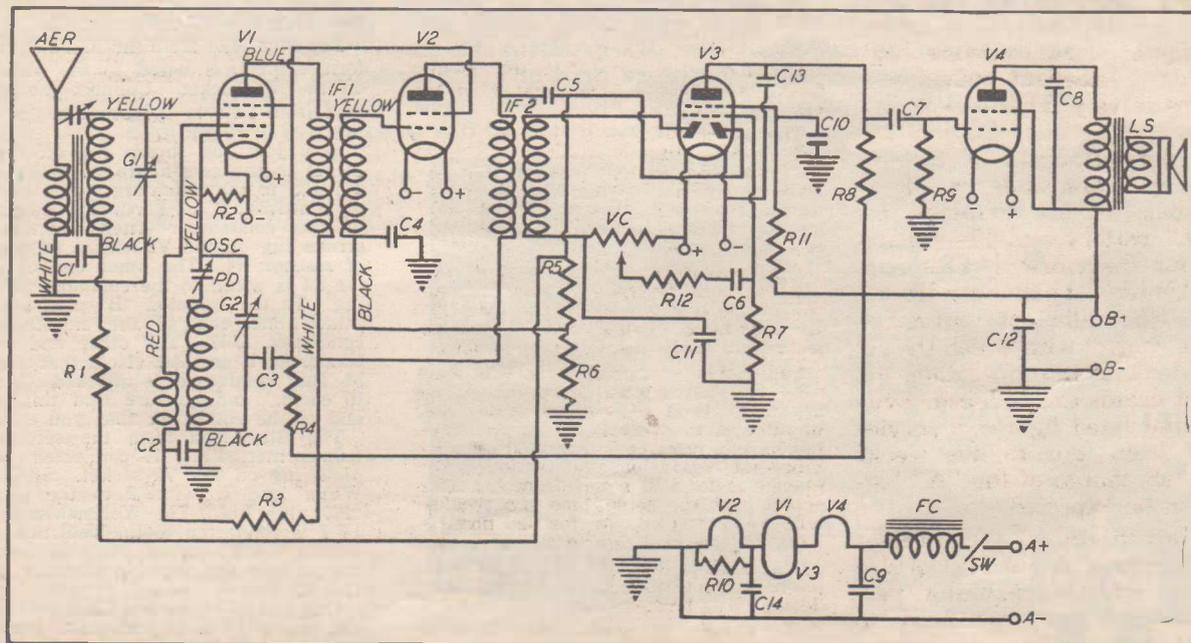
assembly. Do not earth the lugs on the bottom of the condenser, as they will not function if this is done. The filament circuits must be wired in the correct manner, or the set will be a failure. The various biases are obtained by the voltage drop across the filament circuit of the set, and if the valves are incorrectly wired, the bias will be incorrect. For this reason, too, the specified valves must be employed.
