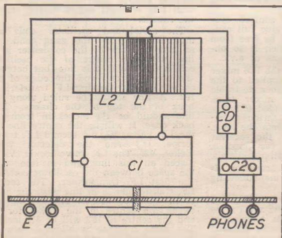
Diagrammatic plan of the crystal set showing the layout and wiring of the receiver.
