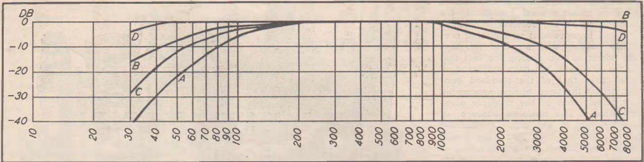
**SOME ILLUMINATING MEASUREMENTS.**—These curves of the performance of the Fidelity I.F. Super 5 show how the overall performance is affected by the design of the i.f. amplifier. Curve B shows the amplifier response and curve A the overall response when measured at the primary of the speaker transformer. Curve C (overall) and curve D (amplifier) result when the output is fed to a purely resistive load.
