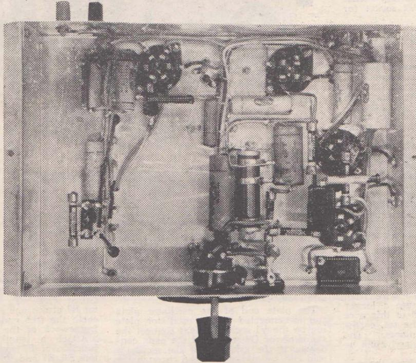
Another photograph of the receiver showing the placement and wiring of parts below the chassis. This illustration should be closely studied before the construction of the set is commenced.
