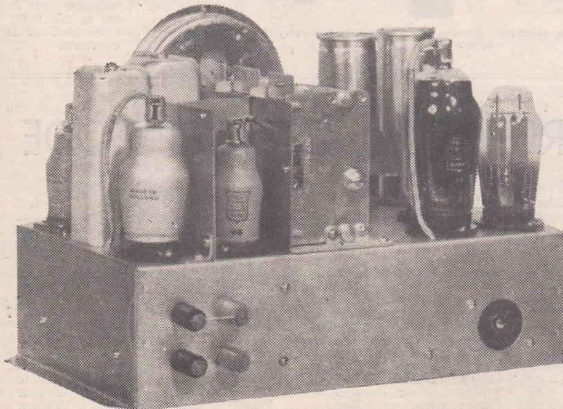
This photograph of the receiver shows the aerial and earth terminals and the loud speaker input socket arranged along the rear side of the chassis.
