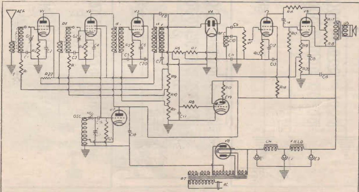
noticed, however, that extreme care, as evidenced by the inclusion of a doubly by-passed radio frequency choke, has been taken to ensure that no r.f. shall enter the audio system.
