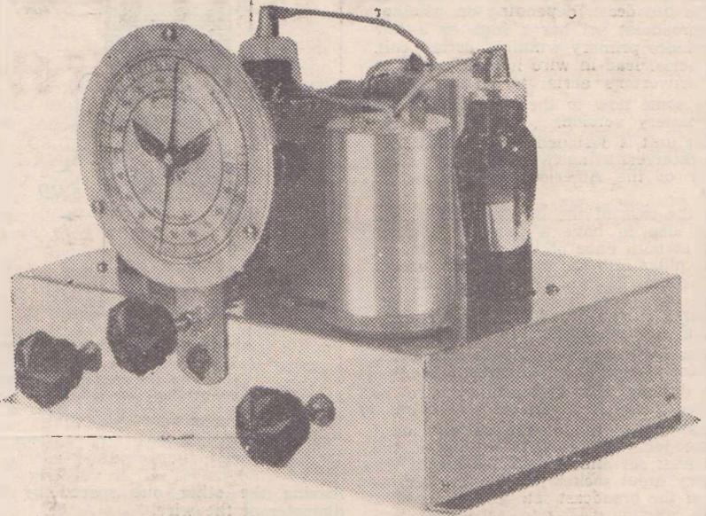
A front view of the completed assembly showing the arrangement of the operating controls. They are (from left to right) the combined volume control and battery switch, the main tuning control and the reaction condenser.
