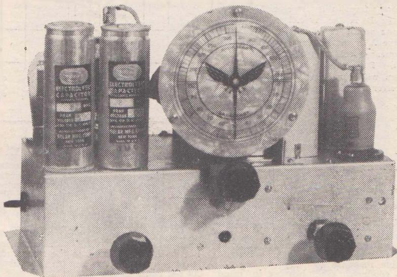
A front view of the finished receiver. The controls required to operate this set are (from left to right) the volume control, the main tuning control and the band switching control.
