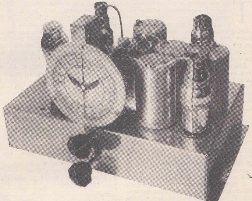
A front view of the Symphony Vibrator Four showing the mounting positions of the controls. They are (upper) the main tuning control and (lower) the volume and battery switch control.
