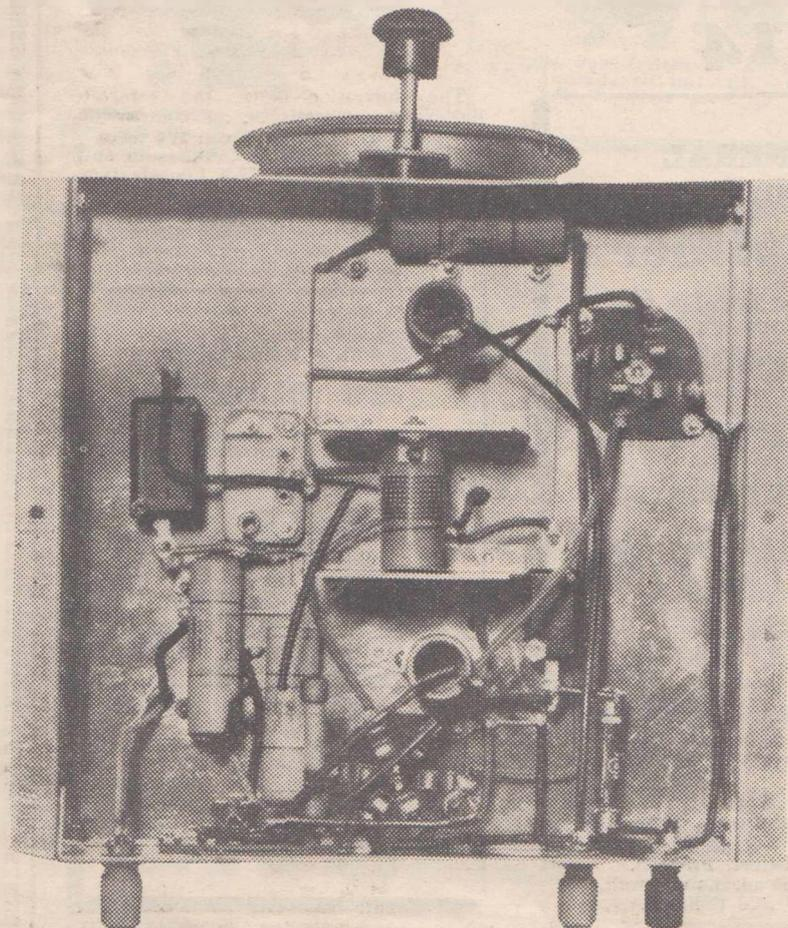
This illustration shows the layout and wiring of the parts below the chassis of the battery version of The Globe Girdler Two.
