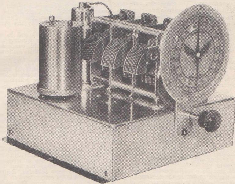
The front view of the completed short-wave converter. The special high gain intermediate frequency transformer is seen mounted at the rear left-hand corner of the chassis.
