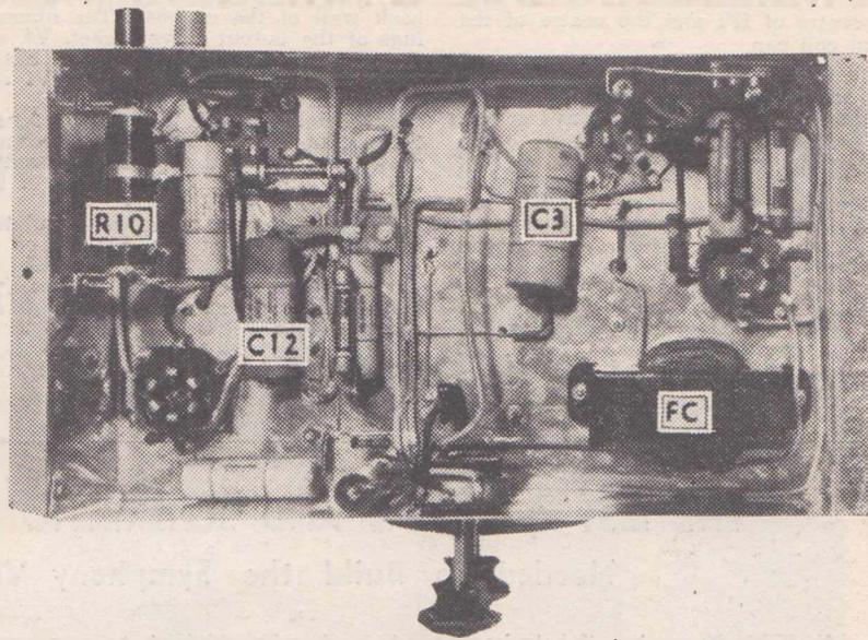
Another photograph of the receiver illustrating the placement and wiring of parts below the chassis.
