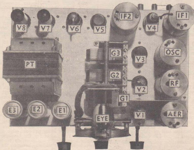
This plan view of the receiver illustrates the arrangement of parts on top of the chassis. All components are keyed to correspond to the written description of the receiver.
