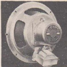
Due to a large magnet of new ALNI steel, the 8in. Rola 8-20 permanent magnet speaker shown above has remarkable sensitivity; incorporates patented Rola dustproof assembly and transformer is sealed against moisture and battery fumes. 42/6.
