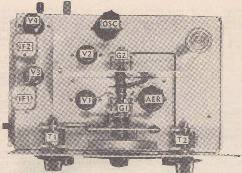
Looking down on top of the chassis gives the builder an excellent idea of the layout required. All parts are keyed to correspond to the written description of the receiver.
