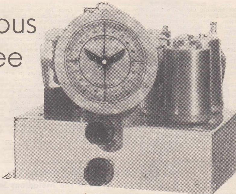
The front view of the Melodious Super Three. The two controls are for tuning and volume.
