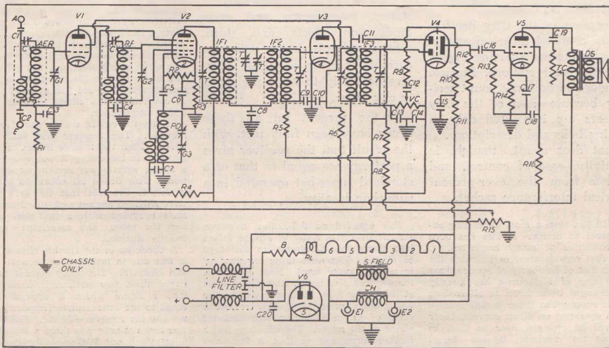
planned to have a slight delay voltage, so that control did not start until half the available audio output was fed to the speaker. It was found, however, that when this delay was eliminated the set's effective noise-level was reduced greatly.
