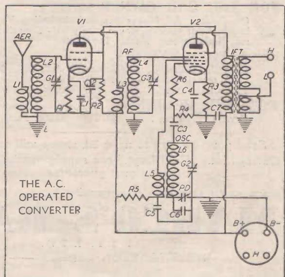
V2 and connect them to the filament lugs of the power input socket. All of this wiring must be carried out by means of twisted leads. Solder lugs should be placed under the bolts holding the coil shields, and these should be connected together with tinned wire and joined to the earth terminal.
