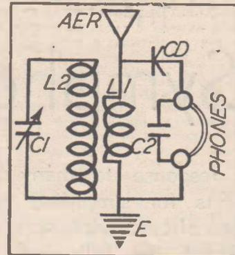
Circuit diagram of the trap-tuned crystal receiver.
