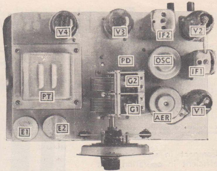
This key-lettered top-chassis illustration should be studied in conjunction with the circuit diagram, the parts list, and the wiring descriptions.
