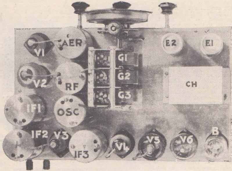
This plan view of the receiver illustrates the layout of parts on top of the chassis. All components are keyed to correspond with the written description of the receiver.
