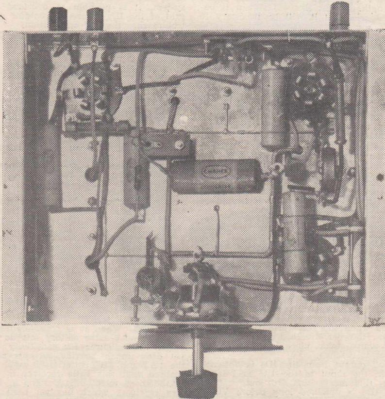
An under-chassis view showing the wiring and placement of component parts.
