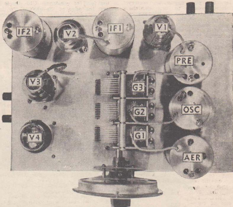
This plan view of the receiver illustrates the arrangement of parts on top of the chassis. All components are key-lettered to correspond to the written description of the set.
