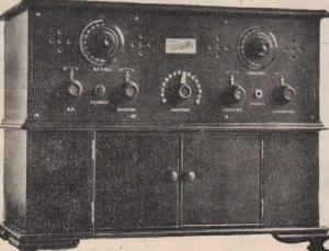
The "Tunola" is controlled by means of only two dials and one of the comparatively few sets that can be accurately and easily calibrated.
