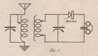
Crystal is Midite, with number 36 copper wire cat whisker. I do not use a buzzer to find sensitive spot on crystal, but carefully manipulate the cat whisker until signals are heard.
