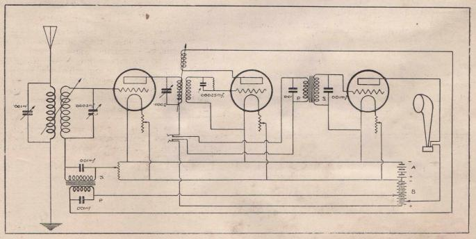
The wires used to make connections from the storage battery to the receiving set should not be insulated with a cotton covering, as the acid in the battery is apt to attack the insulation and cause a short circuit of the battery. Heavy rubber-covered wire is best suited for this purpose.
