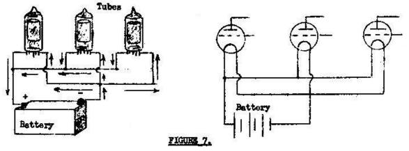
diagram than in the picture kind. The diagram with symbols is often called a "schematic" diagram because it shows the "scheme" of things.
