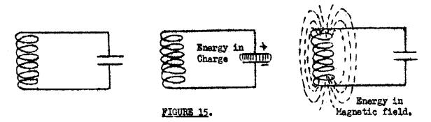
flowing it must pass through the coil.. Whenever current commences to flow through a coil, it rises to the highest value and then falls to zero, there is a rising, and falling magnetic field or a moving field produced around the coil. This field contains energy, low of current from the condenser through the coil will naturally commence at zero, then will quickly rise and will commence to fall again to zero as the voltage difference or electrical pressure between the plates disappears.
