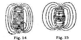
The coils "A" and "B" may be placed end to end on a single piece of tubing as in Figure 14. Then nearly all the lines of force from one of the coils will pass through the conductors or turns of the other one. The amount of mutual inductance depends on the number of lines which link through both coils, consequently we have much more mutual inductance in Figure 14 than in Figure 13.
