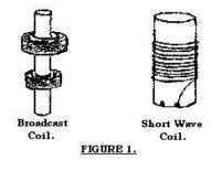
The coils we use in radio are given the job of forcing the alternating currents to give up part of the energy being carried through the circuit. As those currents flow through the coil we have voltages produced or differences of potential produced across the coil from one end to the other. It is the coil's reactance to alternating current which makes the current work for us.
