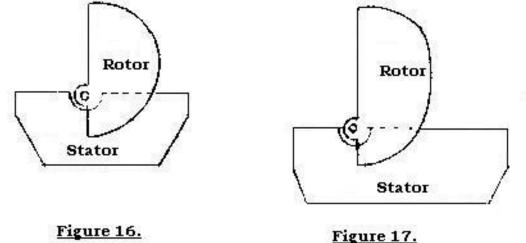
A straight line wavelength condenser changes its capacity according to the "square" of the amount you turn it, and is sometimes called a "square-law" condenser. For example, the difference in capacity between "20" and "40" on a dial would be in proportion to the difference between 400 (square of 20) and 1600 (square of 40). Doubling the dial reading will give four times the capacity.
