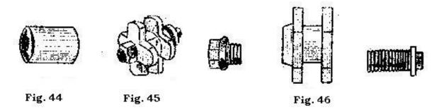
The bobbin type of core is illustrated in Figure 45 and the parts forming it in Figure 46. The screw at the left of Figure 46 is used for holding the core to the holding strip. In the centre of the bobbin itself and at the right is a screw made of the same material as the bobbin which can be screwed inside the bobbin to vary the amount of iron in the core and consequently adjust the coils inductance.
