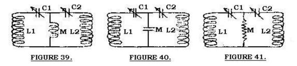
In Figure 41 we have the resistor "M" common or mutual to the two circuits and this makes what we call "resistance coupling". This particular arrangement would not be used in practise because we do not wish to add resistance to tuned circuits. A least, we don't want to add the amount of resistance which would be required to give us a good degree of coupling.
