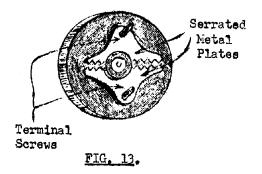
Are enclosed in a moisture proof compartment so that moisture or dust cannot bridge the gap between the plates and allow radio signals to leak away to earth instead of passing into the receiver.
