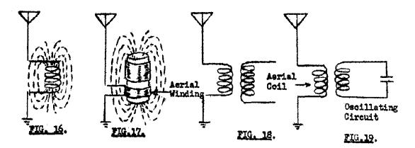
In Fig. 17 we have placed the aerial winding from Fig.16 on the bottom of a piece of tubing and on this same tubing have placed a second winding. Now the lines of force produced by the changing current in the aerial wining will pass not only through the aerial winding itself, but also through the other winding as indicated by the line of Fig 17.
