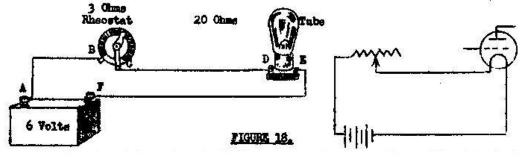
that the rheostat arm is not all the way around. The arm's position lets 3 ohms resistance remain in the circuit. The wires too have some resistance, just for illustration say the wire between "A" and "B" has  $\frac{1}{4}$  ohm resistance, the wire from "C" to "D" has  $\frac{1}{4}$  ohm resistance, and the wire from "E" to "F" has  $\frac{1}{2}$  ohm resistance. Let us add up the resistances.
