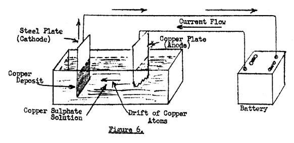
The fact that the metal connected to the positive terminal dissolves away and is carried across through the liquid to build up on the negative plate suggests that the metal is carried by a current of electricity which appears, consequently, to move from the positive terminal of the battery, to the positive plate, through the liquid from positive to negative, to the negative plate and back, to the negative terminal at the battery.
