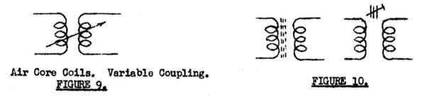
At one time all transformers for use at radio frequencies were of the air-cored type. This does not mean that the transformers had nothing but air inside their windings, it means that no magnetic substance, such as iron or steel, was used inside the coils. Most air-cored coils were wound around a circular former made of some insulating material such as bakelite or specially treated cardboard.
