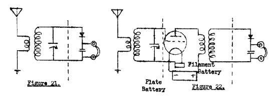
There is no end to the things such a tube can be made to do and we can use the same identical tube as either as an amplifier or as a detector.
