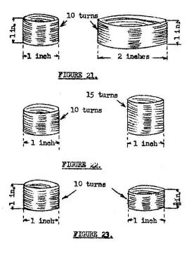
The two coils in Figure 21 have the same number of turns of wire and are of the same length. But the one at the right is twice the diameter of the other one, therefore the right hand coil has much more inductance than the one at the left.
