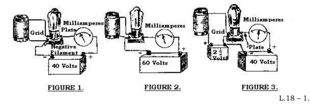
by  $2\frac{1}{2}$  volts grid change equals 8, or 8 times  $2\frac{1}{2}$  equals 20. So we say that the amplification factor of this tube is 8.
