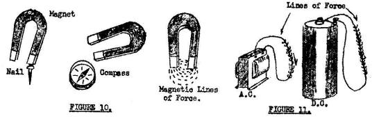
Between the magnet poles there are invisible "lines of force". The nail tries to come close to the magnet so that it can carry more of these lines. The Compass needle turns so that the lines pass through it from end to end. These lines of force make up what we call the "magnetic field".
