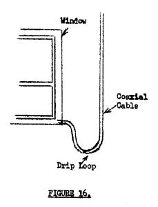
The lead-in may enter the house through a ventilator or through a hole in the <u>lower</u> section of a window frame. In either case a loop should be left in the cable as shown by Figure 16 to allow rainwater to drip outside the house rather than be conveyed inside along the lead-in cable.
