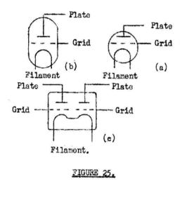
standard symbols for the diode and triode valve, no difficulty will result in figuring out the function, in a circuit, of the multiple electrode types such as tetrodes, pentodes, octodes etc., whether they exist singly or in combination.
