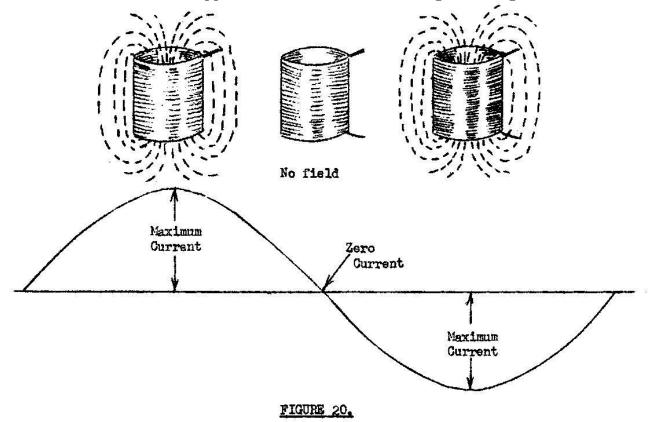
As the frequency of the alternating current increases, the number of times the field rises out of and falls back into the; coil in one second will increase. Consequently the greater the frequency, the greater will be the counter e.m.f. and the more opposition there will be to the original voltage. So you see that increase of frequency increases the reactance of the coil since the opposition to the original voltage is what constitutes reactance.
