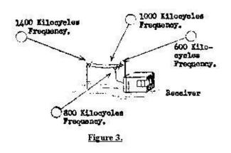
The different stations send out "carrier waves" of different frequencies. Broadcasting stations use the frequencies between about 500 kilocycles and 1600 kilocycles.
