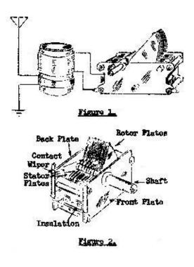
tuned circuit. With no reactance remaining, any signal at this resonant frequency will produce very great currents in the condenser-coil circuit and high voltages will be generated.
