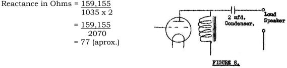
Notice that at a frequency of 50 cycles the 2-mfd, condenser has a reactance of more than 1500 ohms while at a frequency of 1035 cycles the same condenser has a reactance of only 77 ohms. Here you see that the rule "more frequency – less reactance" holds good.
