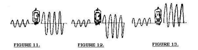
You remember from a previous lesson that so long as the grid has a negative potential with respect to the filament or cathode, no electrons are attracted to the grid and no current flows in the grid circuit. While the grid is positive, however, it attracts electrons and there is a flow of current in the grid circuit.
