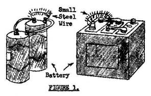
In Fig, 1 is shown an experiment which illustrates the effect of resistance. If you use two dry cells, connected together as at the left, or if you use a single cell of a storage battery such as a radio A - battery or an automobile battery, you will have
