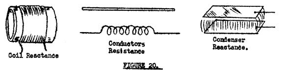
Therefore, in all the circuits we are investigating just now we want as little resistance as we can possibly get. Resistance is reduced by using short connections instead of long ones, by using large wires instead of small ones, and by using material which is a good conductor of electricity. Copper is the best conducting material that is cheap enough to use for wires and connections.
