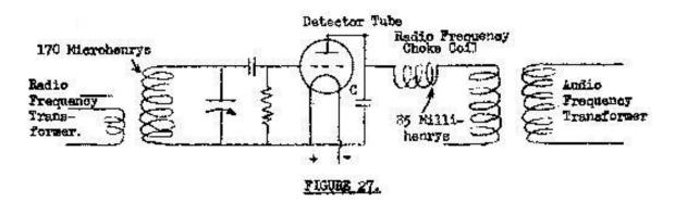
Over at the right hand side of the detector tube in Figure 27 you will se a radio frequency choke coil having an inductance of 85 millihenrys. Let's figure out the opposition or reactance of this coil to radio frequency currents having the frequency of 1000 kilocycles. Here we will use the formula (4) and fill in the values this way.
