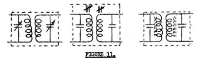
Intermediate frequency transformers, like radio frequency- transformers, are now provided with facilities for varying in their inductance over a small range. With this type the tuning condenser
