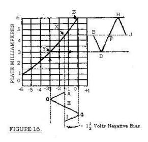
voltage becomes zero. Following upward on the zero voltage line we find it crosses the curve at 6 mils (point "z"). Consequently, the plate current increases to 6 mils.
