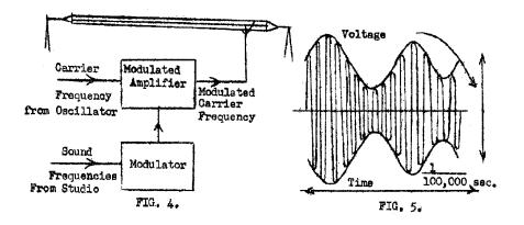
The result of combining these two frequencies is this: the rise of sound voltage are added to the voltage of the, carrier and make the carrier voltage higher at that point. The drops of sound voltage then lower the carrier voltage when the sound voltage lowered.
