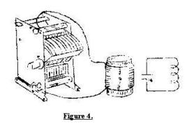
Were you to trace out the connections made to each of the tuning condensers in the receiver, you would find that each one connects to a coil as in Figure 4. The symbol for such a circuit is shown at the right hand side of this illustration. Such an arrangement of coil and condenser makes what we call an "oscillating circuit" or an "oscillatory circuit". The action that takes place In one of these circuits is as follows:-
