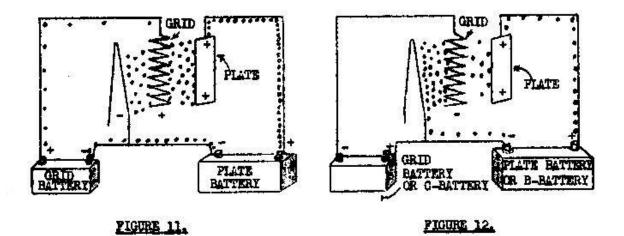
Now look at Figure 11. You see the grid is located right in the midst of the space charge. You can also see that the potential of the grid is higher than that of the filament because the grid is connected to the positive side of a small battery of which the negative side is connected to the filament. Therefore, the grid is positive and the filament negative. Whenever the grid is at a higher voltage than the filament we say the grid is positive.
