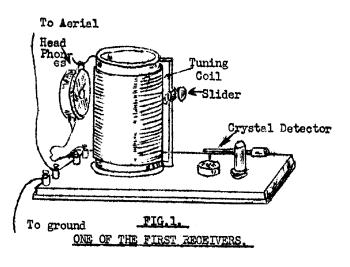
The next development put tubes ahead of The detector, between the aerial and the detector. Those were the days of "DXing" for everybody, The letters in radio mean long distance reception.
