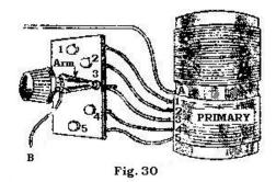
the turns between "3" and "5". If the primary consists of 25 turns, with 5 turns between each two taps, we have 15 turns working between point "A" and point "3".
