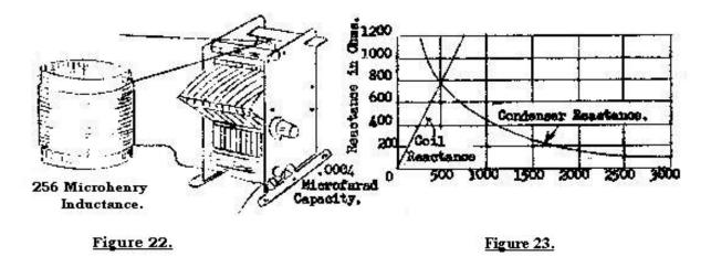
We will make a new set of reactance curves for the parts in Figure 22. These curves are shown in Figure 23. The larger coil with its greater inductance makes the coil reactance go up very
