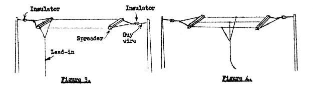
Because modern receivers require such a small amount of aerial signal for satisfactory operation, it is very seldom necessary, oven in country districts to obtain the equivalent of a single wire more than fifty feet long, but this can be done with a two-wire aerial about thirty feet long or with a three-wire aerial twenty feet long. All of the wires in the multiple aerial are connected together by the lead-in attachment.
