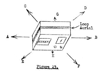
it is desired to listen to, This is done by turning the receiver until the sounds from the loudspeaker are as loud as possible.
