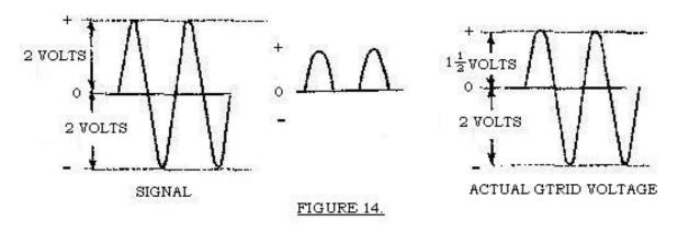
It requires an expenditure of energy to force current to flow through the high resistance between grid and filament inside the valve when the grid is positive. When the grid is negative no such energy is required. It is the previous valve's plate circuit which has to supply the lost energy. Unfortunately this valve is not capable
