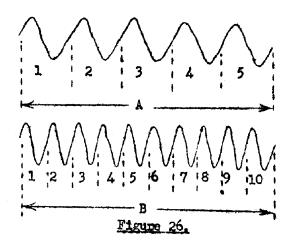
Now look at Fig. 26, Within the distance "a" there are five complete waves. Within the distance "b" (which is the same length as "a") there are ten complete waves. The length of the waves at "a" is greater than the length of the waves at "b", The waves at "b" are coming from the transmitter more frequently than those at "a", consequently the frequency at "b" is greater than the frequency at "a".
