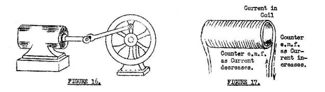
the turning and acts against the steam pressure. Then, as the steam pressure decreases, the weight of the flywheel tends to keep the wheel revolving. A similar action takes place in the coil. While the current in the coil is increasing, or while the lines of force are rising out of the conductors and spreading out, the counter e.m.f. acts against the original voltage. This is shown in Figure 17.
