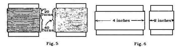
hand coil gives (lx1) l. The left hand coil will have four times the inductance of the right hand one, yet has only twice the diameter or radius.
