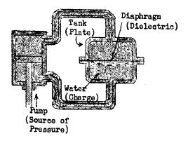
will see a water pump connected to a tank which is divided into two parts by а diaphragm or partition across it. The pump, the pipes, and the tank are filled with water. The diaphragm is thin, made of flexible rubber.
