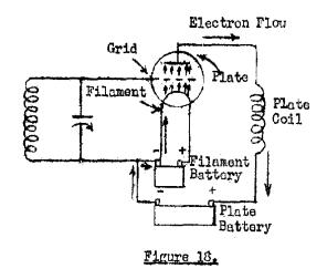
across the space inside the valve to the plate and then they move on around the circuit from atom to atom through the plate wire, the wire comprising the plate coil, the wire leading to the battery, and they are pumped internally through the plate battery and pushed out at the negative terminal to replace those electrons which were "emitted" from the filament.
