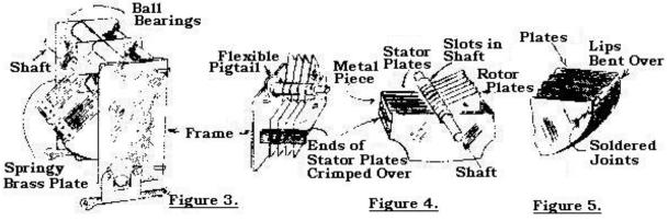
To provide a dependable contact, the condenser of Figure 2 has a contact spring or wiper to which the connection is soldered and bearing with considerable pressure against the shaft.
