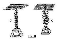
at the left in Figure 8, you have a heavy weight (large inductance) with a comparatively small spring (small capacity) a pull on the weight will set it into oscillation which will be powerful and
