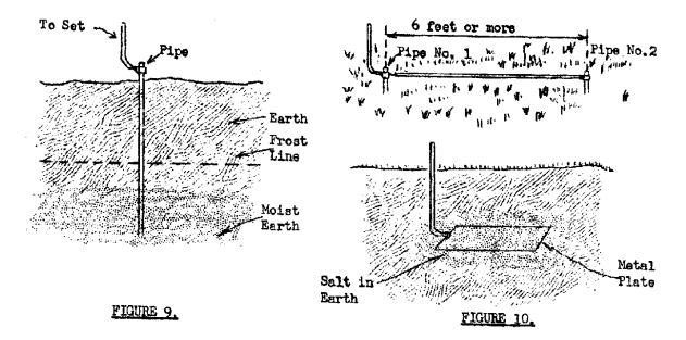
it will go. Any *size* pipe is good enough as an electrical conductor. Nothing will be gained by running a copper wire down inside the pipe.
