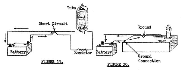
In Figure 20.the negative terminal of the battery is connected to the metal base. The wire between the positive side of the battery and the tube is touching the metal or is "grounded" where marked. Then the battery current flows through the wire to the metal chassis, then returns through the ground to the battery without ever reaching the tube.
