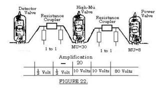
Another power valve has an amplification factor of 8 and will handle signals up to  $13\frac{1}{2}$  volts with 180 volts on its plate. This is the valve to use. It handles the 10 volt signal without distortion and delivers 80 volts into the speaker circuit instead of the 30 volts we would have secured with the previous power valve.
