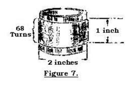
Dividing 83,730 by 43 (microhenrys) gives approximately 345 micro-microfarads. One of the standard tuning condenser capacities is 350 micro-microfarads or 0.00035 microfarads -- so of course that is the tuning condenser to go with this coil of Figure 7.
