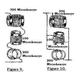
The three inductance coils of Figure 9 are connected together in series. That is all current flowing through any one of them must also flow through the others. We will assume that the three cols have inductances of 300 microhenrys, 100 microhenrys and microhenrys. 200 The total inductance of the three, connected in series is 300 plus 100 plus 200, or 600 Inductances in series microhenrys. add together just as resistances in series add together.
