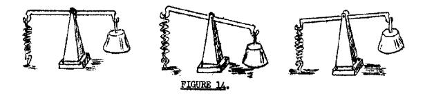
Then the weight would tend to drop and in dropping would spring again. So the action would go on, the spring stretching and compressing the weight rising and falling.
