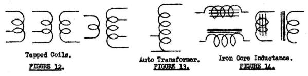
In most transformers we have two separate windings but there is one kind of transformer with one continuous winding which is called an "auto-transformer". Its symbol is shown in Figure 13. Once in a while you will find aerial couplers or radio frequency couplers using auto-transformers.
