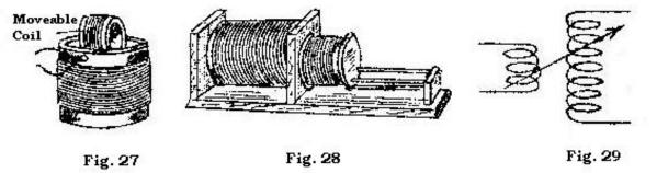
coupling as was done in Figures 21 to 24. We can vary the amount of coupling and so we call such a device a "variable coupler". The name "vario-coupler" was once used to mean the same thing as variable coupler.
