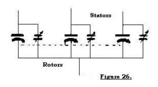
actually shown connected to the condenser gang, but are completely omitted, it being understood that all modern sets use trimmer condensers either on the gang itself or connected to the coils.
