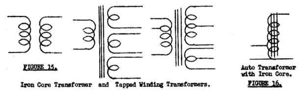
A transformer with two windings and an iron core is shown by the left hand symbol in Figure 15. This is generally the sign for an audio frequency transformer, but it also may indicate any other simple transformer such as one for furnishing filament or heater current to tubes. The other two symbols in Figure 15 indicate transformers with one
