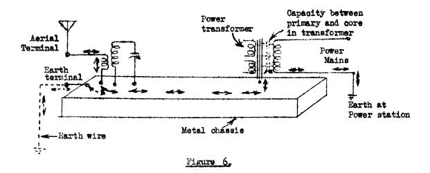
Over the top of the primary winding is another layer of insulating material and then, in turn, come additional windings to supply power to the various valves in the receiver although the primary winding is insulated from the iron laminations, both the primary winding of copper wire and the laminations are conductors and because they are separated by an insulating material they form a small condenser effect which allows radio frequency current to pass through.
