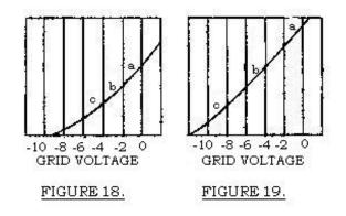
To handle this stronger signal, the one of 3 volts, we must do two things, we must increase the plate voltage on the tube and we must also increase the negative grid bias. If you will look back at Fig. 15 you will see a curve drawn for 135 volts on the
