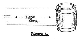
the reactance of the coil is exactly the same as the reactance of the condenser and as we saw earlier, would tend to cancel the other.
