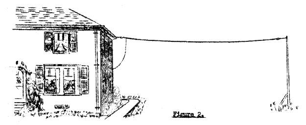
An aerial or this kind is really a large condenser and between the two plates of a condenser you can't have anything better than air from the standpoint of saving every bit of energy from loss.
