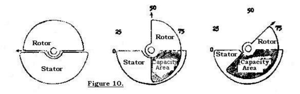
In the centre drawing of Figure 10 the rotor has been turned half way through its total movement from "0" to "50" on the dial readings. Then half of the surface or area of the rotor plate is in mesh with the stator plates. The capacity of a condenser is in proportion to the plate area in mesh, so with the rotor turned half way in we have one-half the total capacity.
