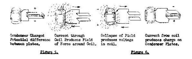
The energy of the falling lines of force now having been expended in charging the condenser, the charge of the condenser again exerts itself in causing electrons to flow back again from the top plate to the bottom. The lines of force are again set up and again keep the current going when the condenser's charge has been expended. This charges the condenser again, positive at the top and negative at the bottom, just as it was at the start.
