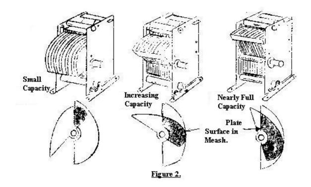
The three pictures in the lower part of Figure 2 show what is happening, You recall that a condenser consists of plates separated from one another by a dielectric. Air is the dielectric of the tuning condenser. The only part of the plate surface which is effective in producing capacity is the part opposite another plate. The only part of the air dielectric which can be placed under an electrical strain is the part between the plates.
