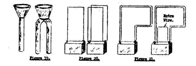
or two, will the battery current flow more easily ? Through the two wires, of course, because just as much current will flow through the second wire as through the first, and the two will take twice as much current as one. The resistance of two wires in parallel is less than the resistance of either or one alone.
