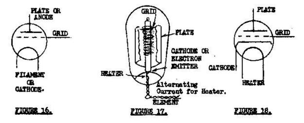
Around the outside of the heater is the cathode, a cylindrical metal surface which is heated and which then emits electrons.
