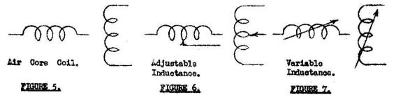
When an air-core coil is built in such a manner that its inductance is continually variable or changeable while the coil is working in the set we call it a variable inductance and the symbols for this arrangement are those of Figure 7. This long arrow drawn right through a symbol always means that the part may have its value changed while the receiver or other radio device is in operation.
