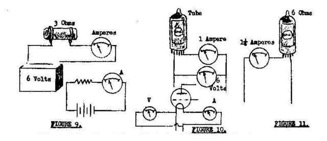
resistance of the filament is really 6 ohms. Now, knowing the filament resistance of this tube, 6 ohms, how many volts must you apply to the filament to make  $1\frac{1}{4}$  amperes flow through it? This 50 tube may be worked with six volts on its filament and a currant of one ampere, but to got the full power it is capable of delivering we have to send  $1\frac{1}{4}$  amperes through the filament.
