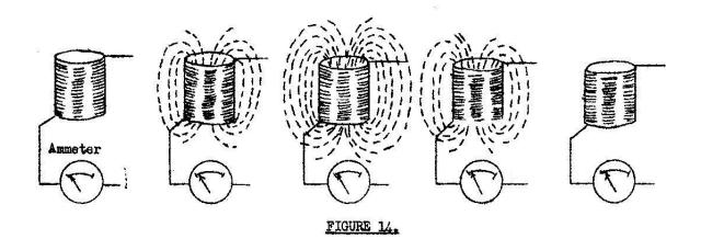
With the action shown in Figure 14, the lines seem to rise out of the coil to spread out as their number increases, and then to drop back into the coil, finally to disappear altogether.
