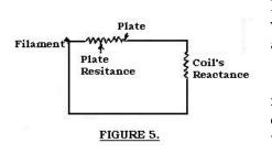
this circuit of Figure 5, it will have to overcome these two resistances just as in Figure 4. Current flowing in the plate circuit would have to overcomes the plate resistance and the coil reactance.
