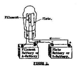
You will also find that a large proportion of our present rectifier tubes are of the two element type. A rectifier changes alternating current to direct current.
