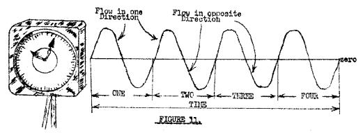
Any "wave" is a disturbance in some substance during a period of time, the disturbance, moving away from the source of the thing which started it.
