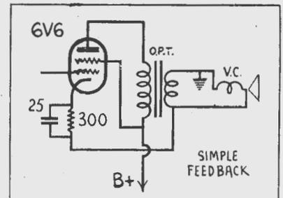
Two minor points have to be watched. One side of the voice coil must be earthed. Which side is to be earthed can be found by experiment, incorrect connection giving increased gain and distortion, even to a point of setting up a squeal. With correct connection the gain is cut back a bit, but the tone improved quite noticeably.
