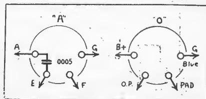
Coil connections for the "Aegis" coils as supplied in the kit by Magrath's
