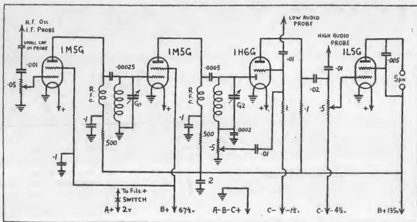
Circuit for an improved Signal Tracer for battery operation.
