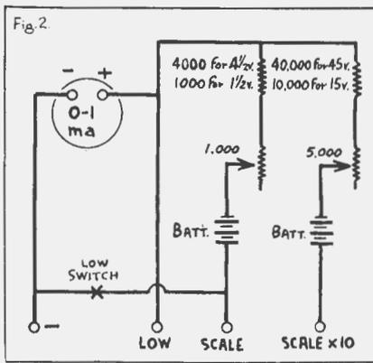
Diagram for a three-range Ohmmeter of infinite value to the serviceman.
