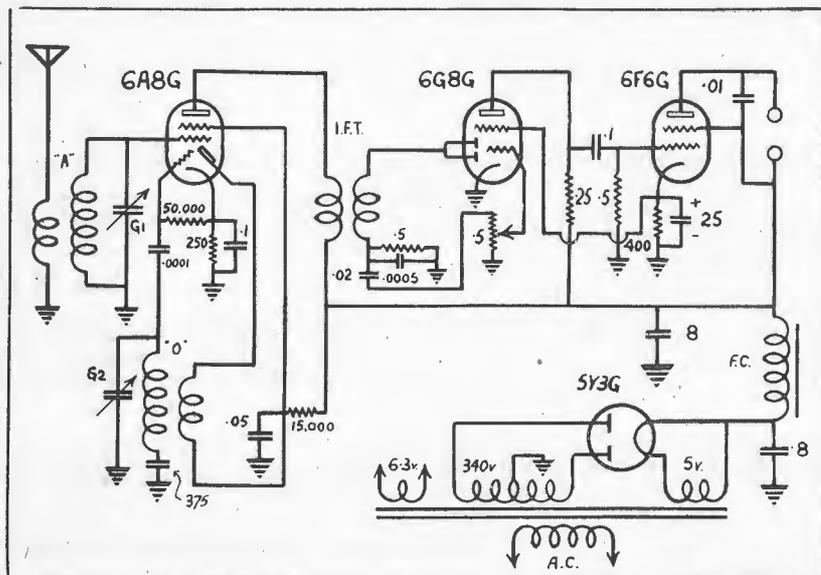
The circuit diagram, which shows the unique screen feed scheme for the detector.
