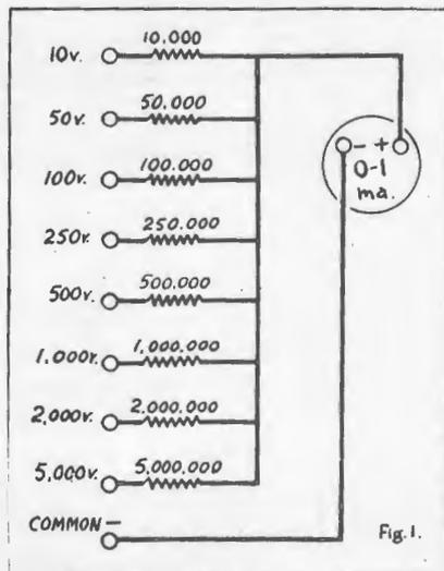
Schematic arrangement for wide-range voltmeter.
