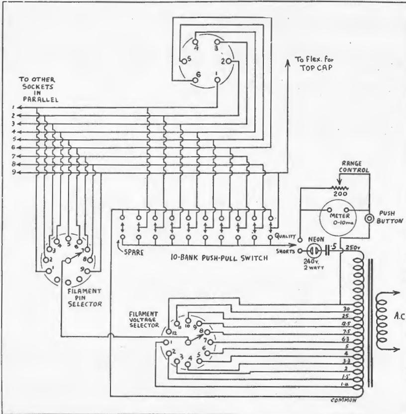
Circuit of the versatile valve tester
