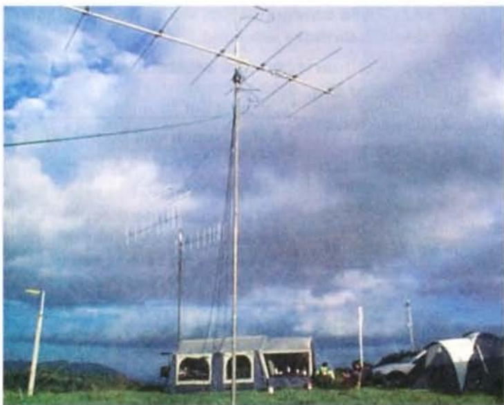
SARC's set up for JMFDC. Foreground 6 m, 23 cm, 2 m vert, behind 2 m, 70 cm.
