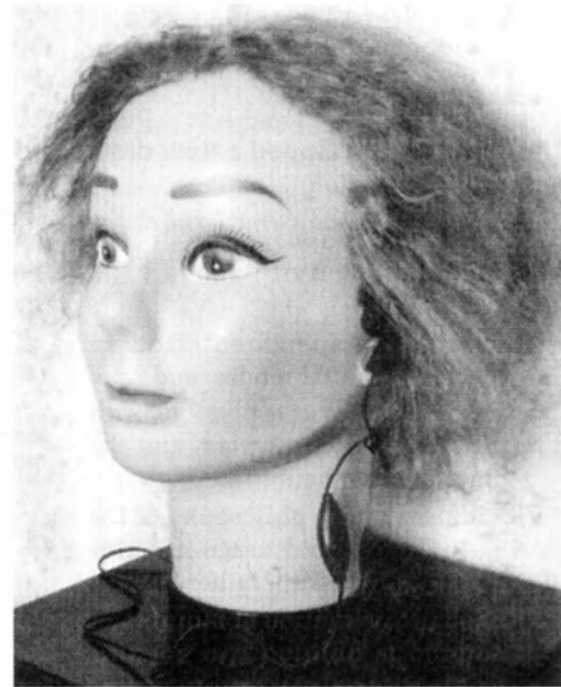
Photo 1 - A mobile phone earpiece and microphone with shirt clip. It has a PTT control box.
