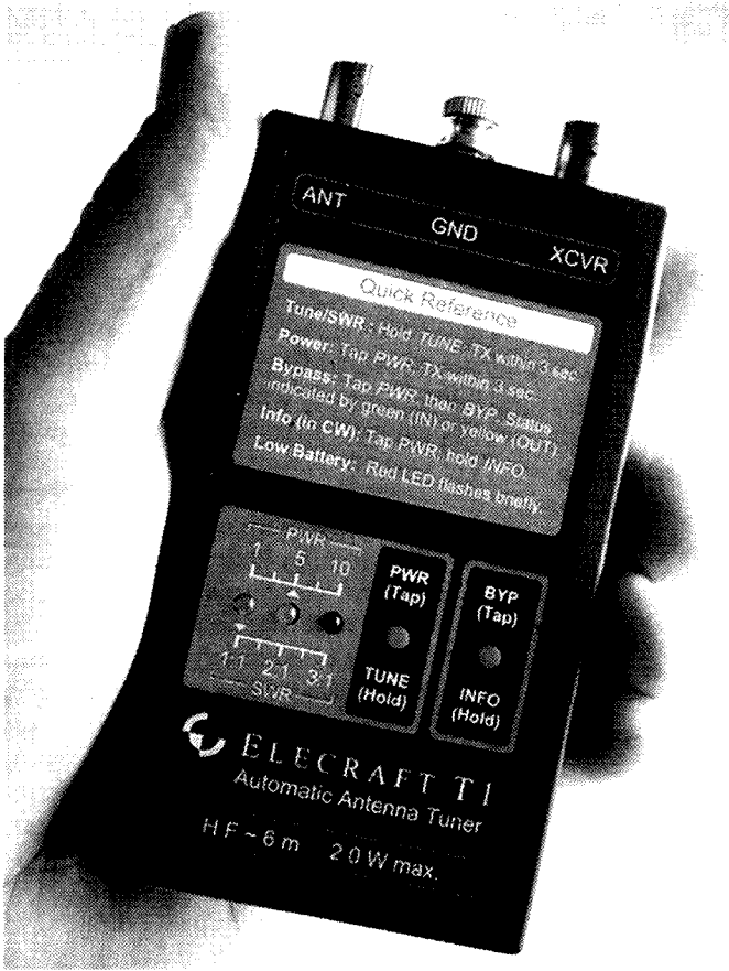
Photo 2 - The completed T1 installed in its case. The battery fits into a compartment in the back.
