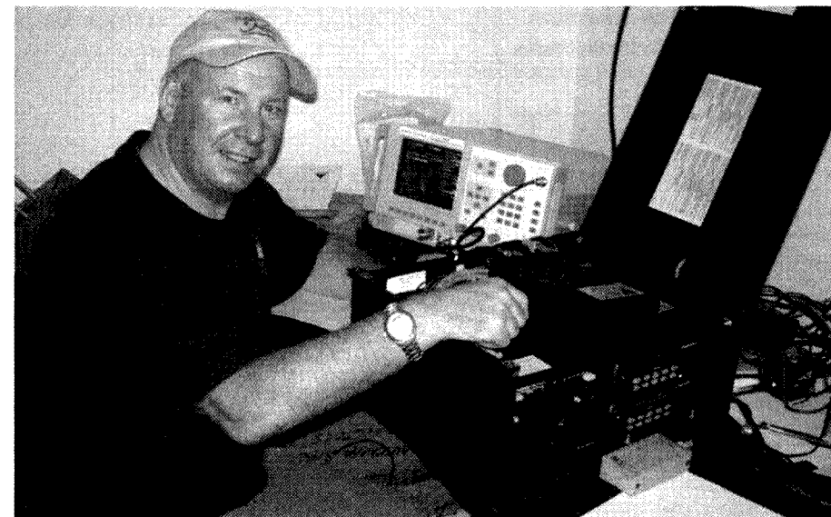
Mark Tell, a RedR Australia register member, aligning a duplexer for a VHF repeater, Middle East
