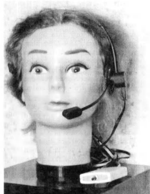
Photo 3 - A disposals ex-telephone single earpiece headset and microphone. It has a similar PTT control box to the Y2 headset combination.
