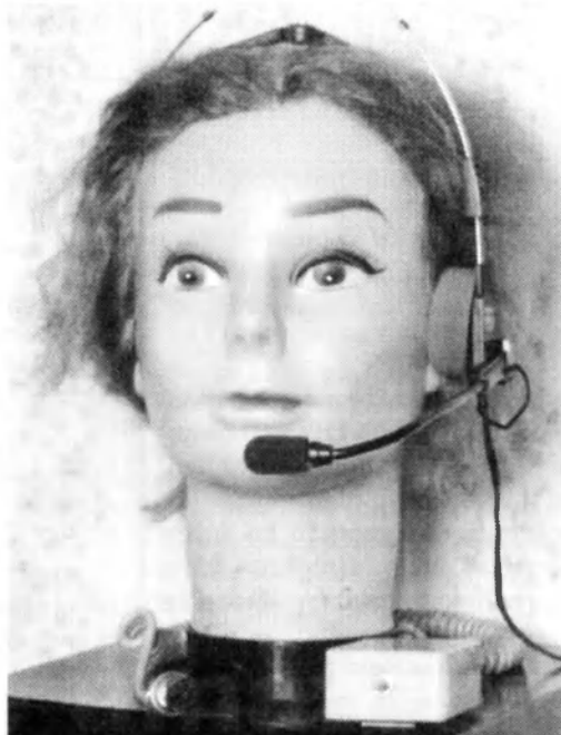
Photo 2 - The Yaesu Y2 headset and microphone with a home-brew PTT control Box. A clip holds it onto the seat belt. The PTT switch is locking one way and spring loaded the other.
