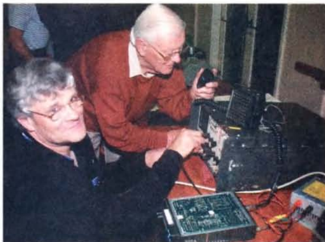
Phil VK5NN checking his radio's deviation with Greg VK5ZBD's test rig
