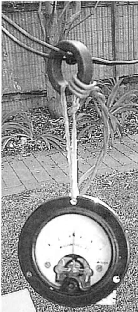
Photo 2 Measuring of common mode current on open wire line to the X3 antenna.
