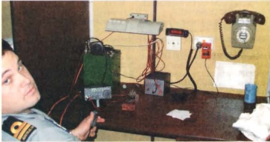
The "shack" was set up in my stateroom (cabin/office). The SG2020 is just above my left hand, with the metal box housing the 18 Ah GelCell and the body of the FT-7800 behind it. The remote head of the FT-7800 can be seen between the desk lamp and the phone. The GelCell battery is charged by a 1 amp Arlec charger. The efficiency of this charge seemed to be affected by the ship's 60 Hz supply.
