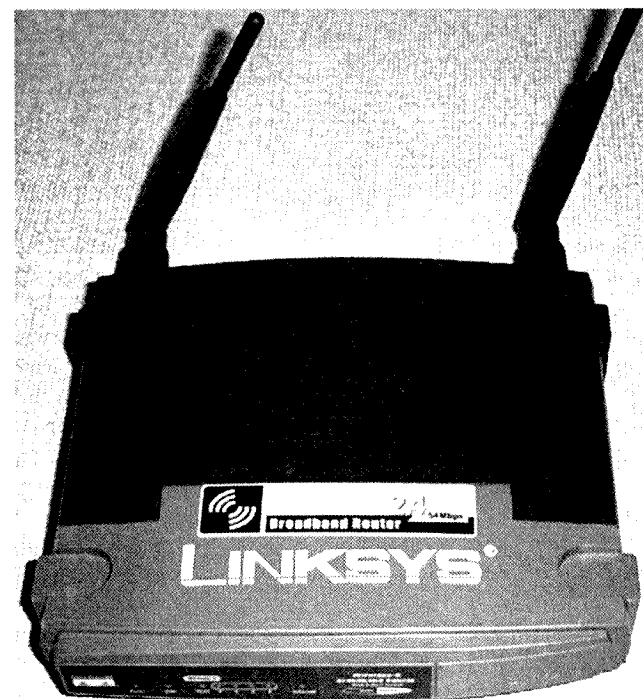
Photo 1 – A Linksys "data transceiver" with removable antennas which are replaced by an external antenna for wireless LAN use.
