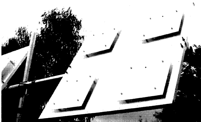
Photo 1. Final dual patch array
