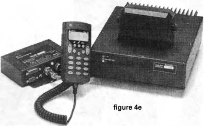
Figure 4. Models showing changes in transceiver styles. Types a) 6801, b) 7727-TB having separate control head, c) 8525 with separate control head, d) the X-2 or 9105 and e) 2010 (NGT) mobile version with junction box
