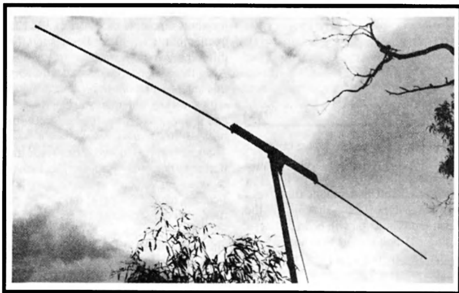
The compact HF directional antenna up in the air and working.
