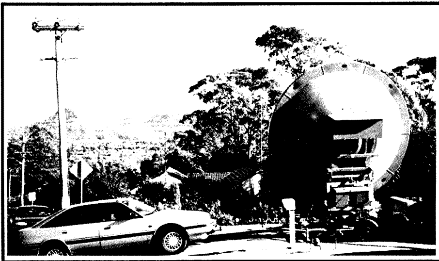
VK2ALU's 3.7 metre 10 GHz EME dish in its operating position at the front of VK2ALU's GTH during a 10 GHz EME test with G3WDG. The dish is looking towards the western horizon window with G3WDG.
