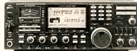
IC970H: Deluxe 2m/70cm multi-mode base station with power supply, can have 23cm, 13cm and 25-950MHz receiver added. Satellite features built-in.
