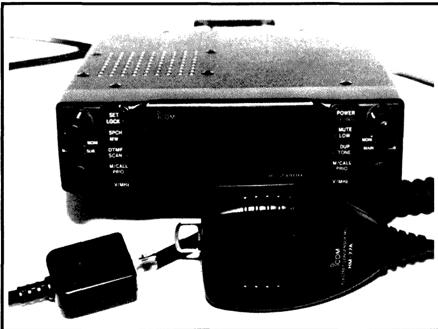
The IC-2340H. Note the small size in relation to the handheld microphone, and the modular mic socket which is on a lead coming from the back of the transceiver.
