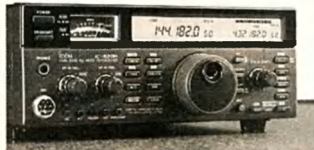
IC820H: Superb performance in a dual band (2m/70cm) all-mode transceiver for voice, satellite or packet.
