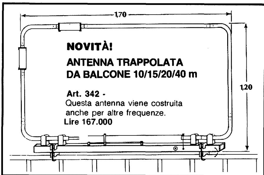
Fig 1 — The line drawing of the compact loop antenna as advertised in Radio Rivista .
