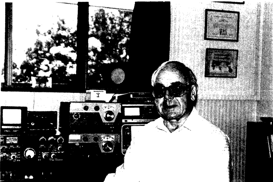
Robin at his rig. The Kenwood TS830 S is to the left, with a Ham M rotator on top. To the right are the Drake twins, the R-4C and a T-4XC.
