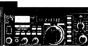
IC-730 HF Transceiver 80-10 meter Ham bands compact mobile 100W SSB CW AM
