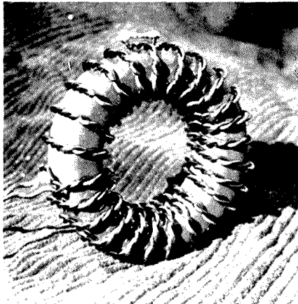
Photo 5 Matching transformer showing tapping method.
