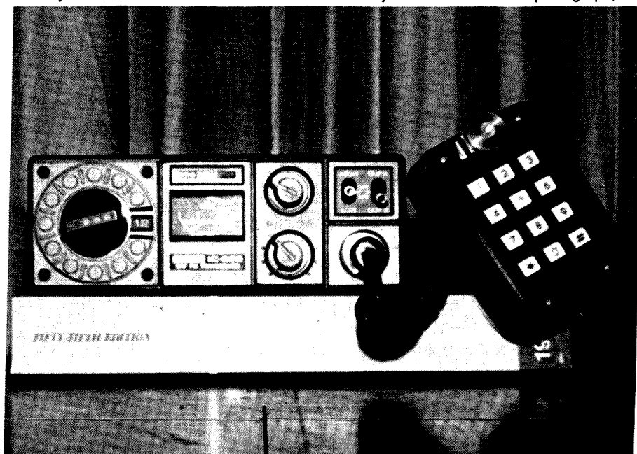
Touchtone Pad on rear of Microphone gives access to Repeater “Auto-Patch” and Public Telephone Network. Tone IC in Mic. gets power from rig via simple modification to Mic. Socket.
