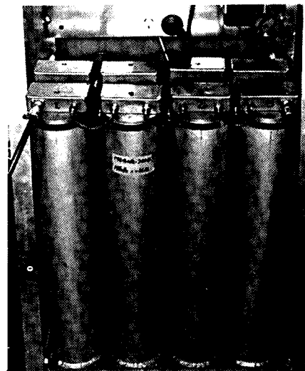
The repeater is unique in its design using eight home constructed aluminium cavities. The design is based on the ARRL repeater handbook.
