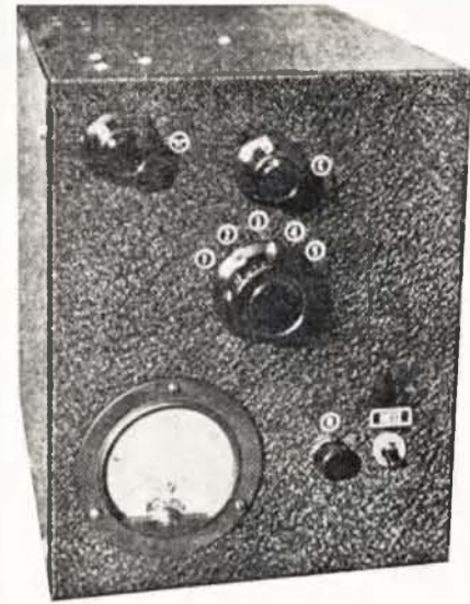
Front view of the Shoebox II. Linear. Although similar in concept to the earlier Shoebox Linear, the Mark II. features more flexibility of operation and ease of construction. Inexpensive 6HF5 tubes are used in parallel to deliver as much power as the builder desires.
