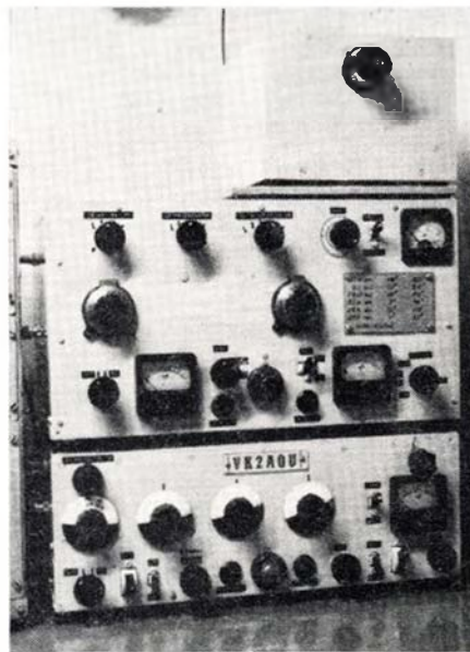
The Transmitter and Exciter on the desk with the Linear on top. The VFO stands again on top of the p.a. with heat shield underneath. Transmitter is switched to six bands, each 500 Kc. wide.
