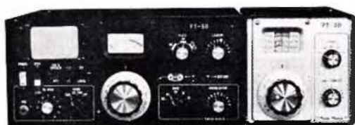
FT-50 Transceiver FV-50 V.F.O. 80-10 mx, peak inp. 100w.
