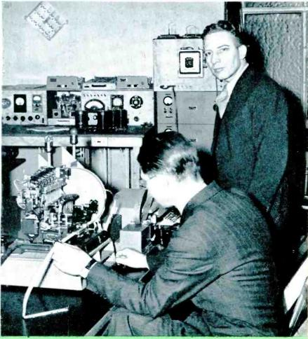
The error-proof radio printer developed by RCA Laboratories for use on the high-speed communication circuits.
