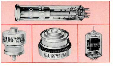
and oscillator. It can be operated with full ratings at frequencies up to 500 Mc.
