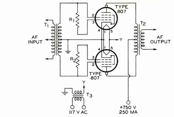
$R_1 R_2 = 20000$  ohms, 1 watt, carbon  $T_1 = Driver$  transformer, turns ratio of total primary to one-half secondary 1:1.25; Stancor A4761 or equivalent
