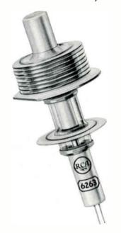
designed for use in low-power mobile transmitters and in aircraft transmitters at altitudes up to 60,000 feet without pressurized chambers. They have a maximum plate-dissipation rating of 13 watts (ICAS) and can be operated with full ratings at frequencies as high as 1700 Mc. The 6263 has a mu of 27; the 6264 has a mu of 40.
