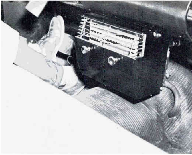
The "Auto-air" conditioner installed is a compact unit allowing fingertip control—a touch of a button sets the comfort level and this level remains constant from idling to over 100 miles per hour
