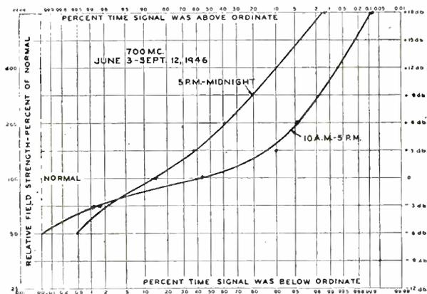
Fig. 13—Recordings on 700 megacycles—June 3 to September 12, 1946.
