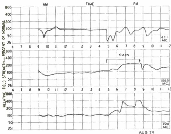
Fig. 7—Effect of rains on signal strengths—August 29, 1946.
