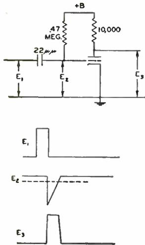
Fig. 16—Non-linear differentiator for delaying a pulse.
