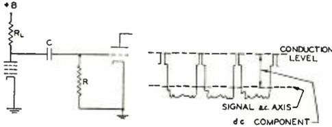
Fig. 3—The simple dc restoration circuit.
