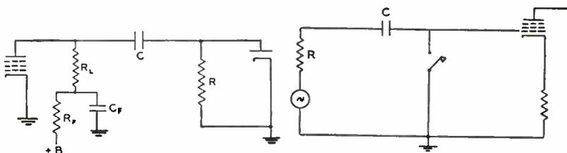
Fig. 11—Low boost circuit.
