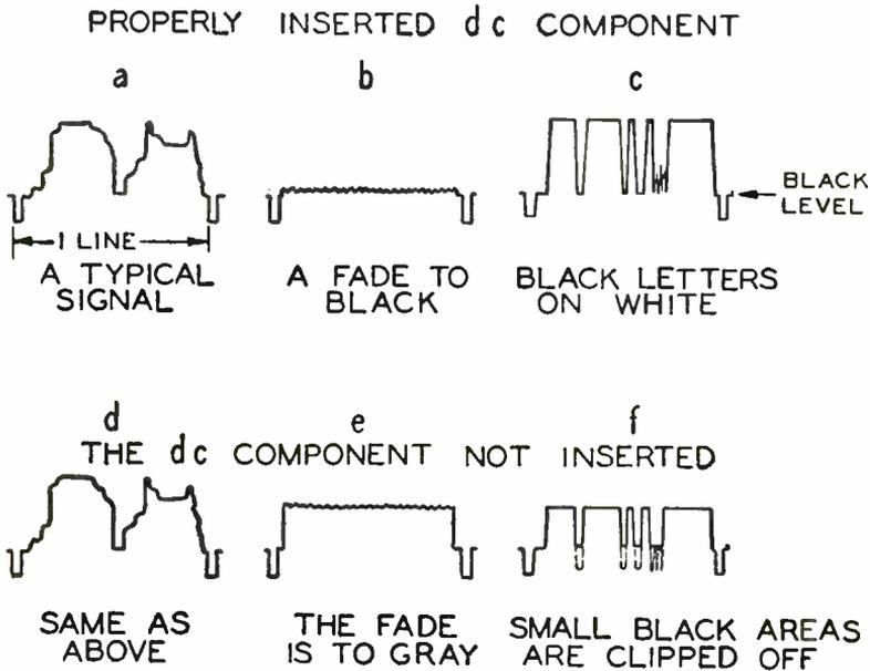
Fig. 2—Insertion of dc component.
