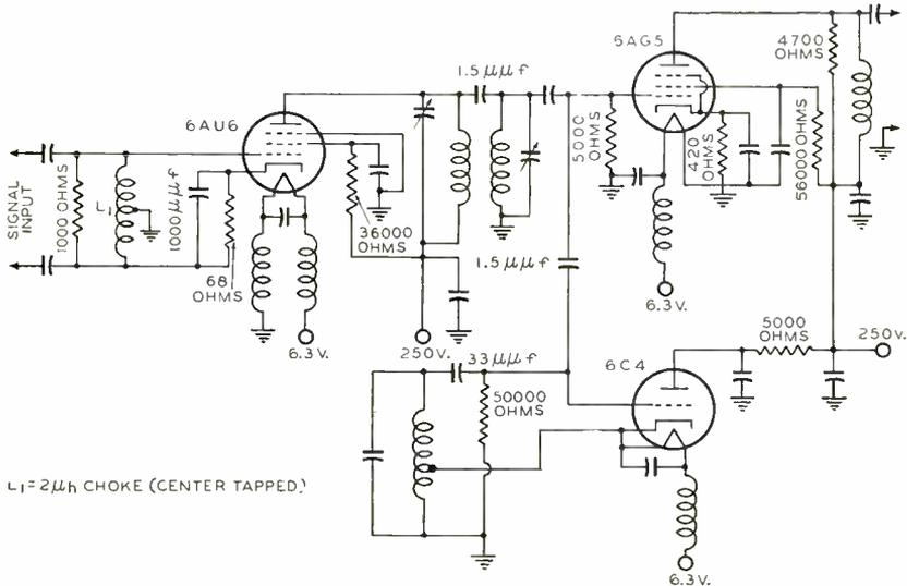
Fig. 3—Radio-frequency unit, unbalanced circuit.
