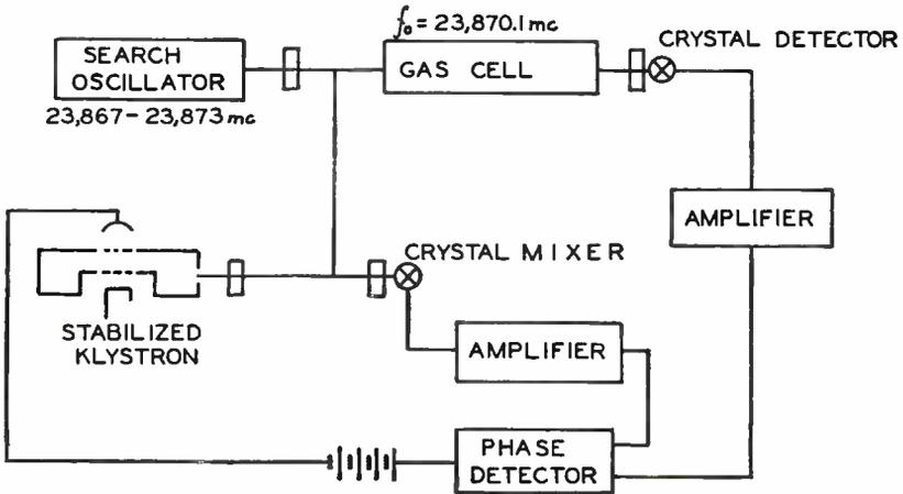
Fig. 3—Block diagram of stabilization system.
