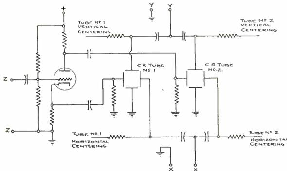
Fig. 5—Circuit for three-dimensional scan.
