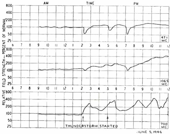
Fig. 4—Effect of thunderstorm on received signal strengths.
