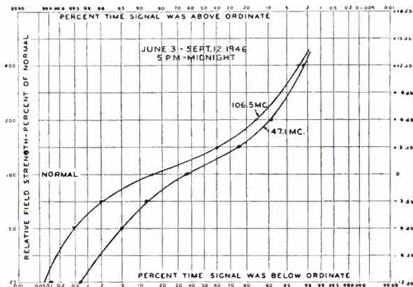
Fig. 12—Night recordings, 47.1 and 106.5 megacycles—June 3 to September 12, 1946.
