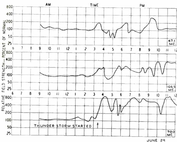
Fig. 5—Effect of thunderstorm on 700-megacycle signal—June 29, 1946.
