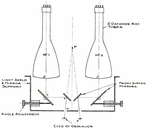
Fig. 1—Arrangement of the stereo-oscilloscope.
