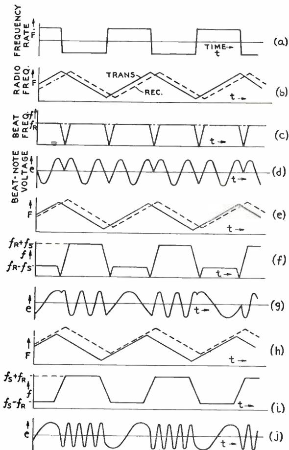
Fig. 3.—Frequency and voltage wave forms for symmetrical-sawtooth or triangular modulation.
