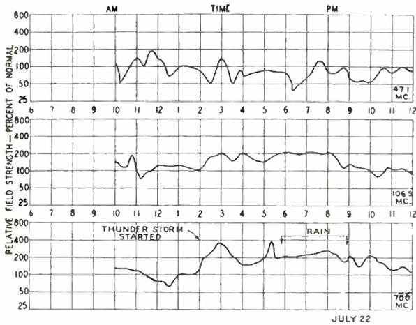
Fig. 8—Effect of rains on signal strengths—July 22, 1946.
