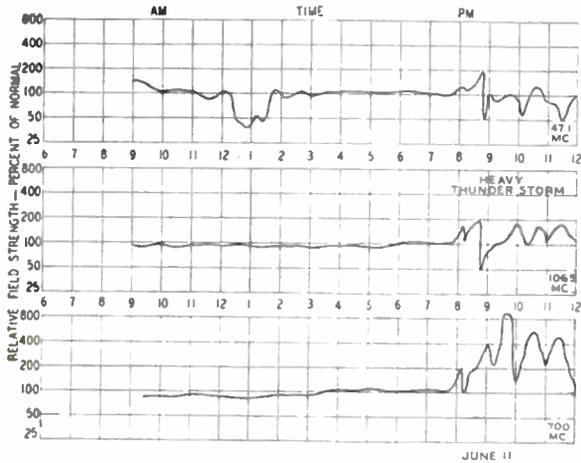
Fig. 6—Effect of thunderstorm and rains on signal strengths—June 11, 1946.
