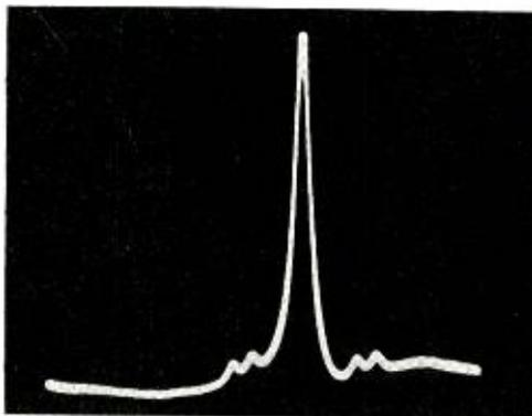
Fig. 2—The (3,3) absorption line of ammonia.
