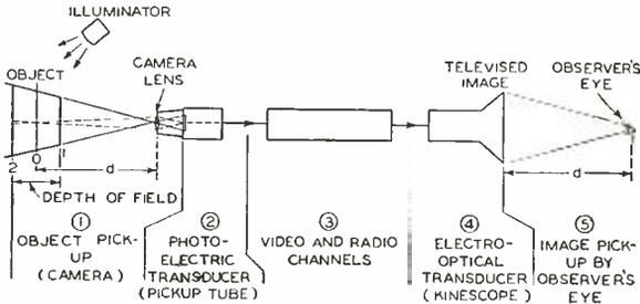
Fig. 1—Optical and electrical components of television process.
