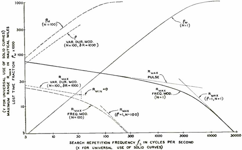
Fig. 6—Dependence of maximum radar range on search repetition frequency. For universal use of solid curves,
