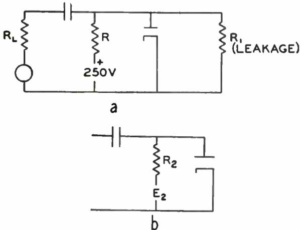
Fig. 10—The effect of leakage.
