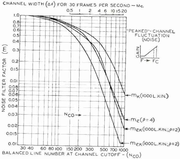
Fig. 11b—Effect of channel width on fluctuation filter factors for a peaked channel.
