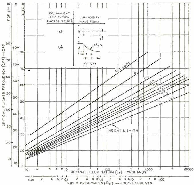
Fig. 6—Threshold flicker values for intermittent illumination.
