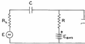
Fig. 9—Positive bias circuit.
