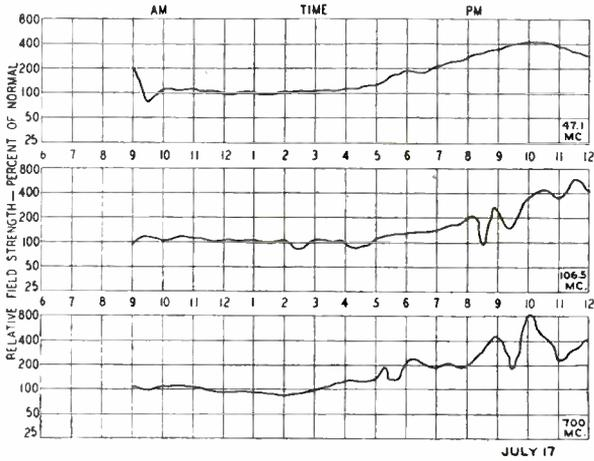
Fig. 2—Field strength recordings—July 17, 1946.
