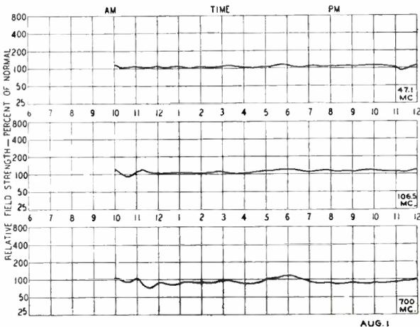
Fig. 3—Field strength recordings—August 1, 1946.
