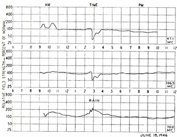
Fig. 9—Effect of rains on signal strengths—June 18, 1946.
