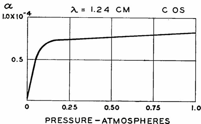
Fig. 2—Absorption of carbonyl sulphide.
