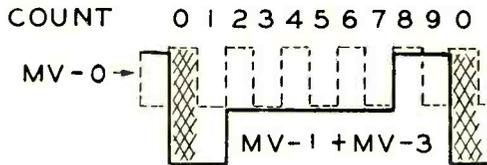
Fig. 8—Derivation of "0" indication in binary decade.
