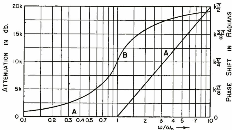
Fig. 1—Semi-infinite constant slope characteristic.
