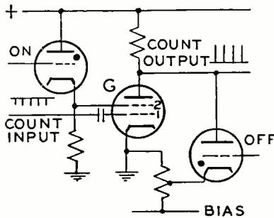
Fig. 13—Switching by gas tubes.
