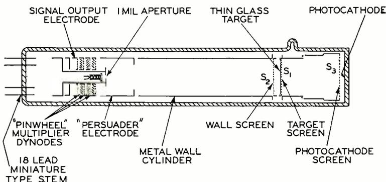
Fig. 3—Cross-sectional diagram of the Mimo tube.
