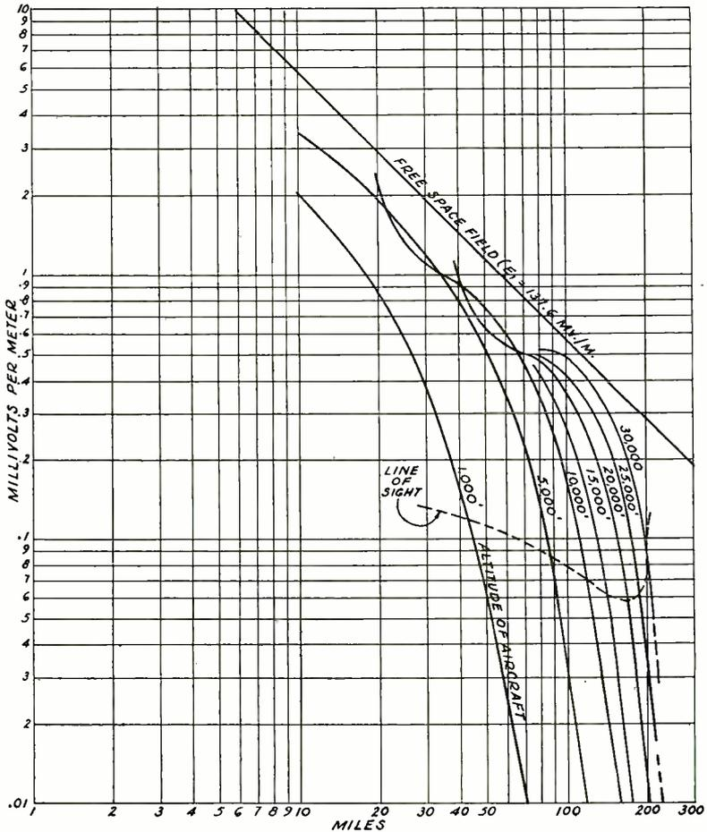
Fig. 2—Calculated field strength versus distance for the indicated altitudes of the aircraft. (Receiving antenna 30 feet high, 200 watts radiated power at 100 megacycles, for vertical polarization over sea water with a ground conductivity of 4.3 mhos/meter and a dielectric constant of 81.)
