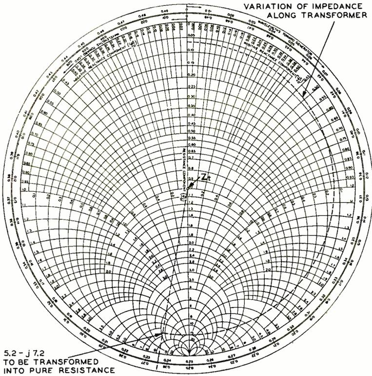
Fig. 5—Determination of correct transformer length.
