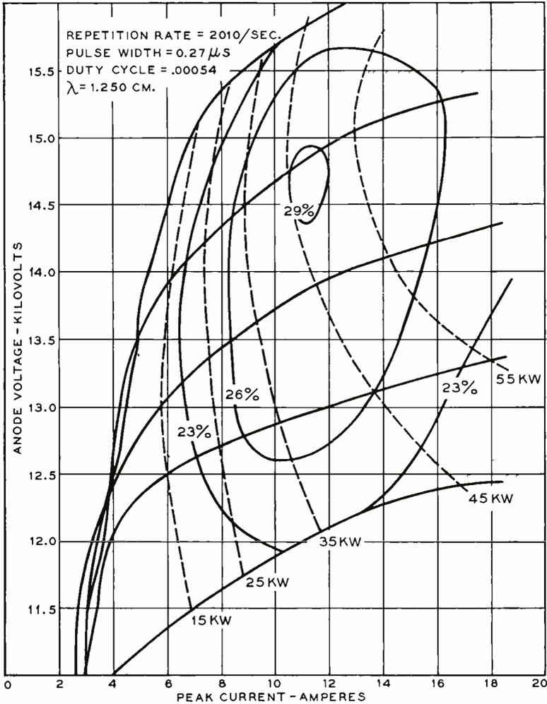
Fig. 6—Performance chart of quartz transformer magnetron.
