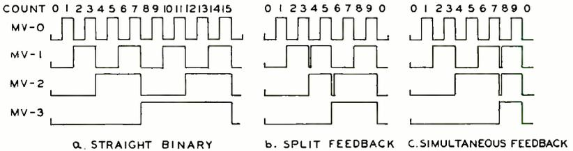
Fig. 5—Application of feedback to binary chains.
