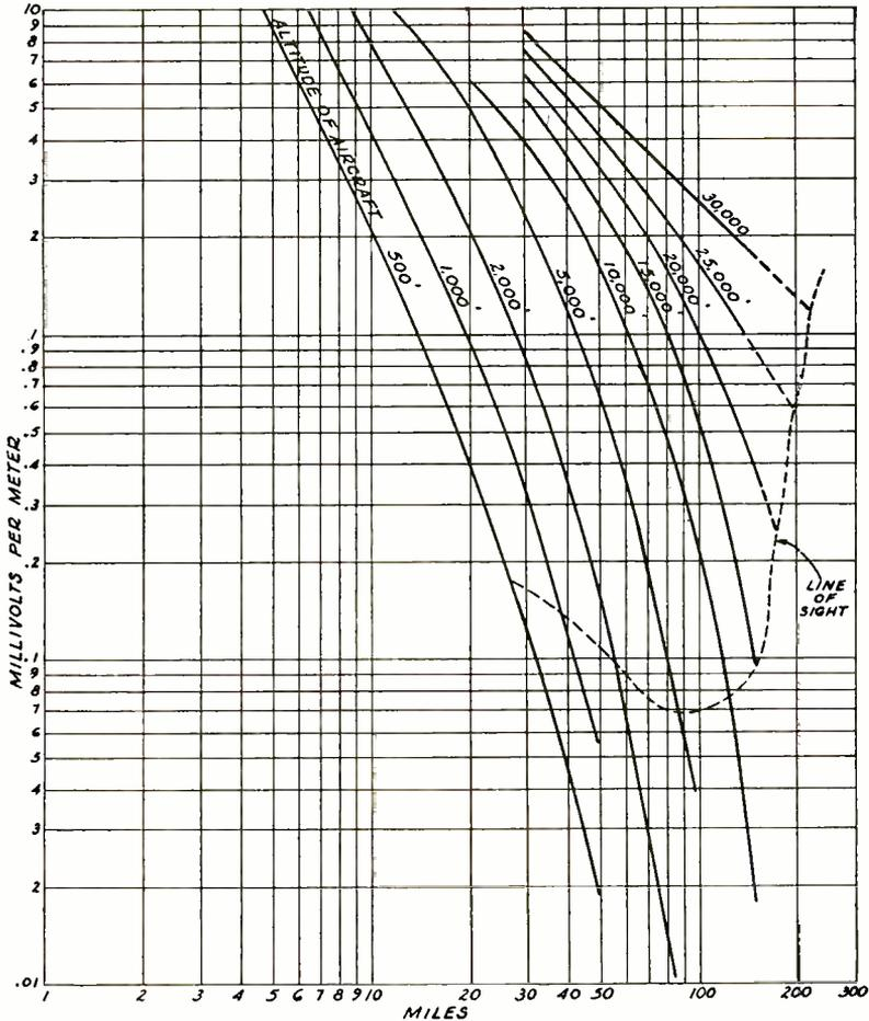
Fig. 3—Calculated field strength intensity versus distance for the indicated altitudes of the aircraft. (Receiving antenna 30 feet high, 200 watts radiated power at 105 megacycles, for horizontal polarization over land with a ground conductivity of  $5 \times 10^{-14}$  electromagnetic units and a dielectric constant of 15.
