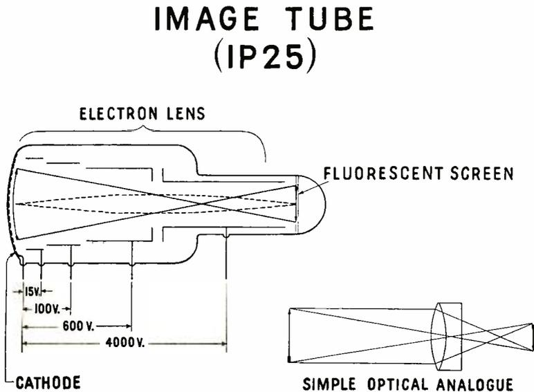
Fig. 4—Schematic diagram of 1P25 Image Tube.
