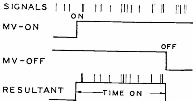
Fig. 9—Method of mixing timing and count signals.
