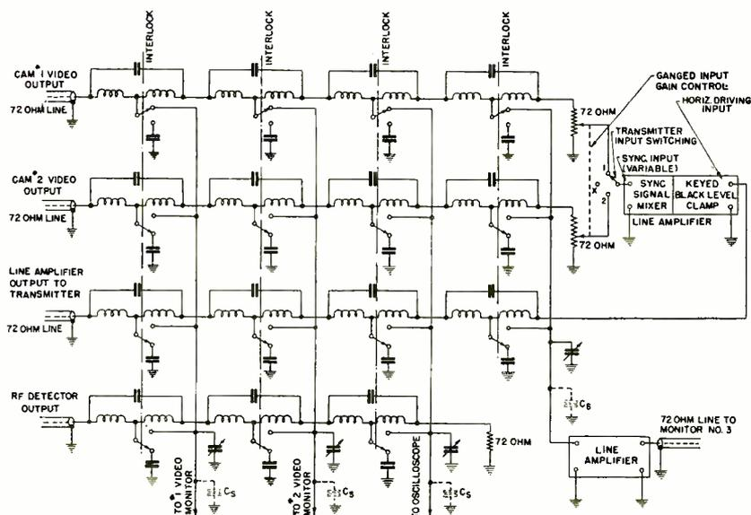
Fig. 7—Master control unit. (Simplified video block diagram.)
