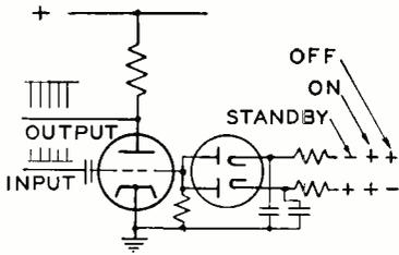
Fig. 11—Duo-diode method of switching.
