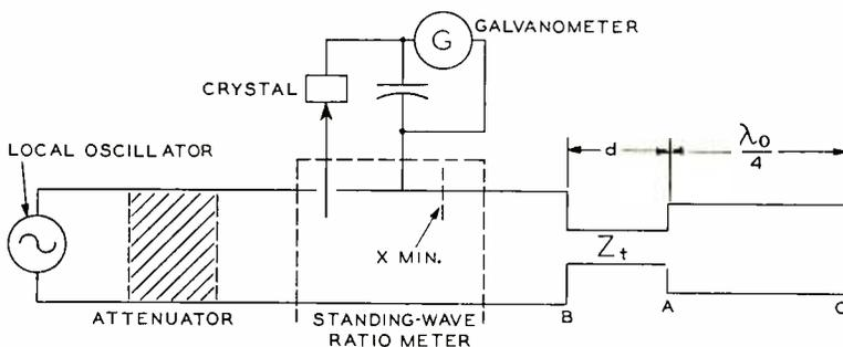
Fig. 3—Experimental setup for determining transformer "end-effects".
