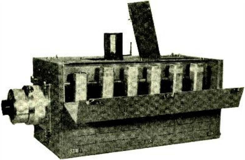
Fig. 10—Image orthicon camera with viewfinder. (Hinged cover opened to show video amplifier—top access door open.)
