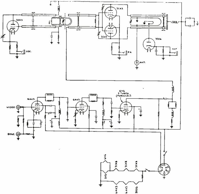
Fig. 7—Mimo transmitter diagram.
