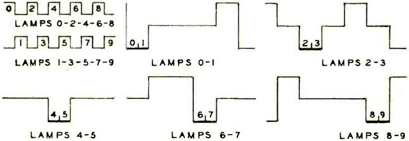
Fig. 7—Derivation of indications in binary decade.
