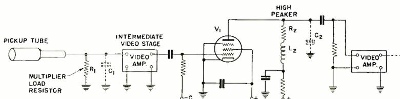
Fig. 12—Block diagram illustrating "high-peaker" correction network.
