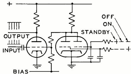
Fig. 12—Double triode method of switching.
