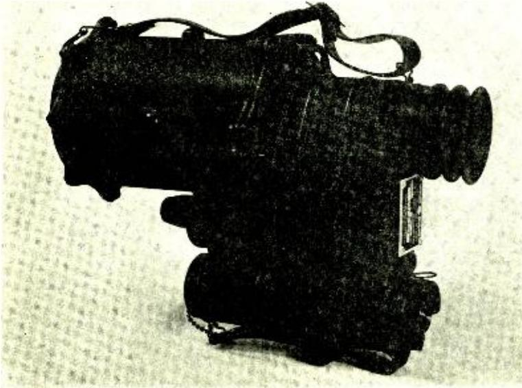
Fig. 1—Infrared telescope.
