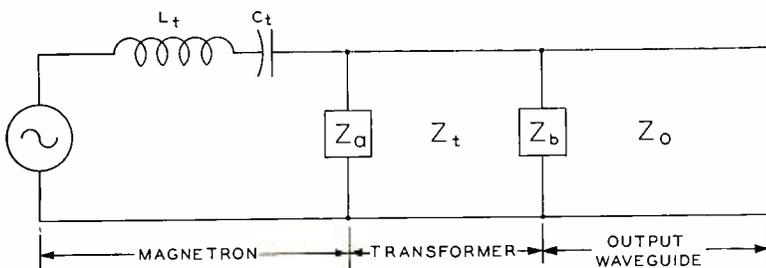
Fig. 2—Schematic diagram of waveguide-output magnetron.
