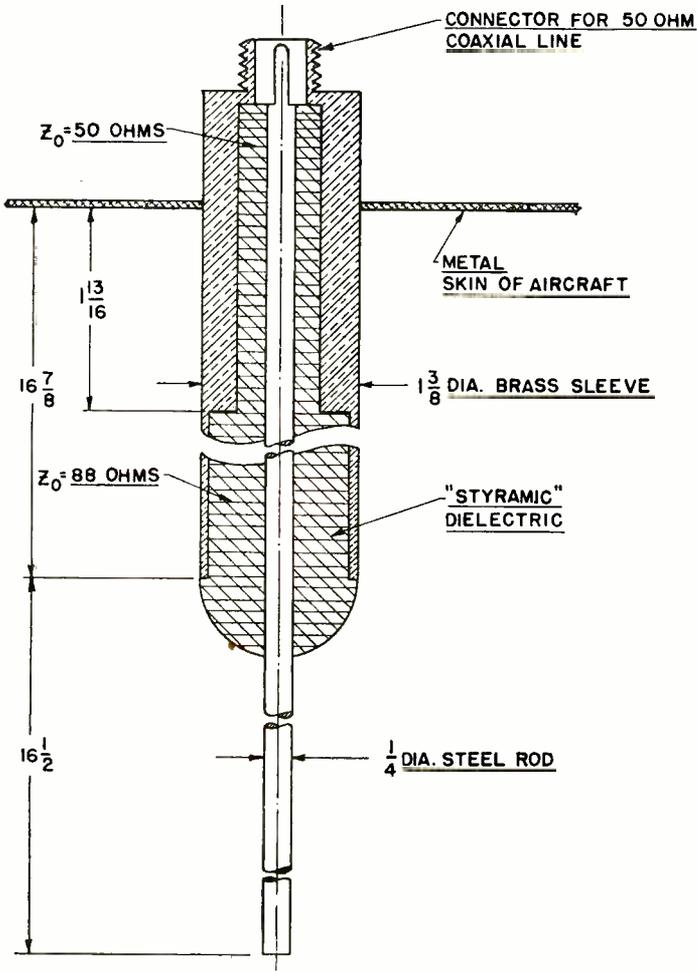
Fig. 15—Transmitting antenna.
