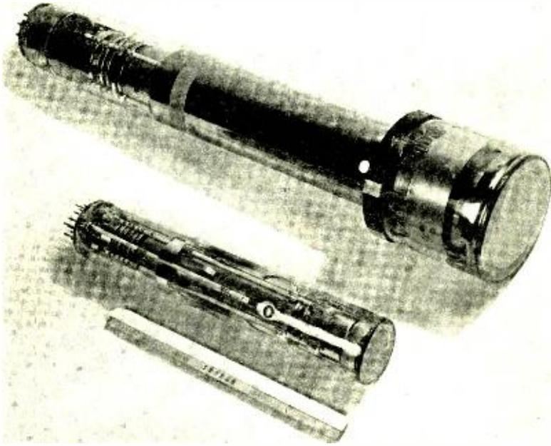
Fig. 1—Comparison of the Mimo tube with an image orthicon.
