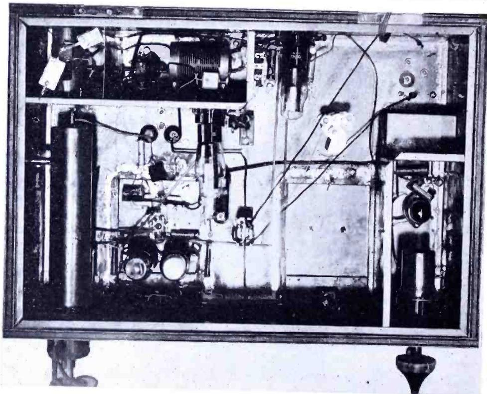
Fig. 2—Sub-chassis view of the inter-electrode capacitance meter.
