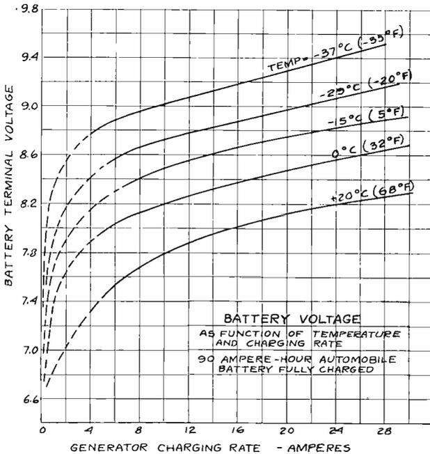
Fig. 7—Variation in battery voltage with charging rate at various battery temperatures.
