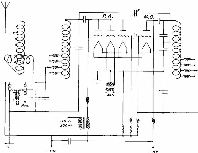
Fig. 4—Schematic circuit diagram of the transmitter.
