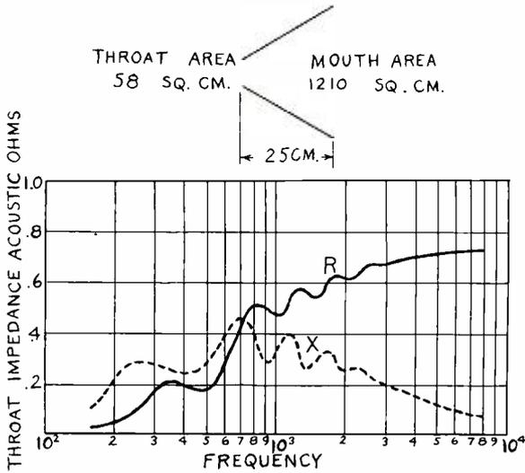
Fig. 1—Acoustic impedance characteristic, at the throat of a conical horn of the dimensions shown for comparison with the exponential horn of Fig. 2. *R*, resistive component. *X*, reactive component.
