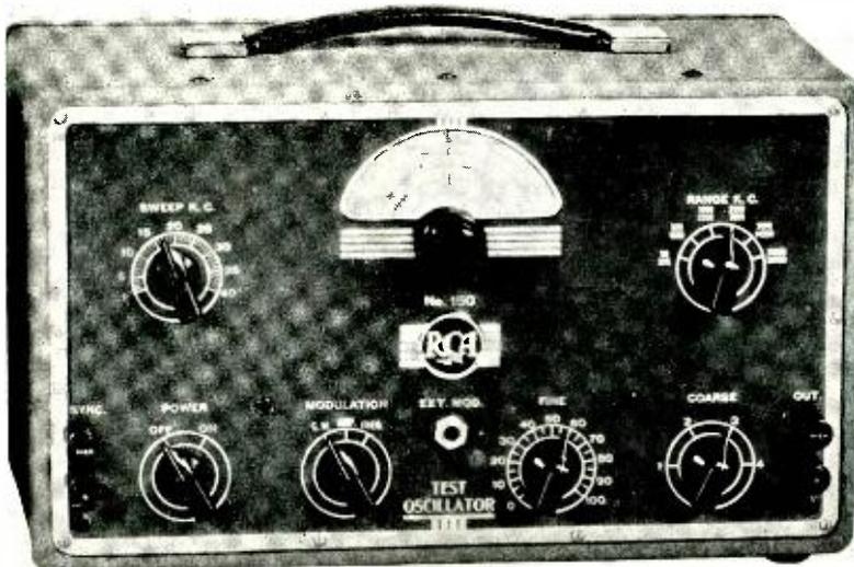
The electronic sweep test oscillator is another instrument used in servicing modern broadcast radio receivers.
