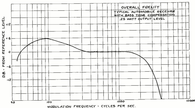
Fig. 13—Overall fidelity curve, typical automobile receiver incorporating bass compensation.
