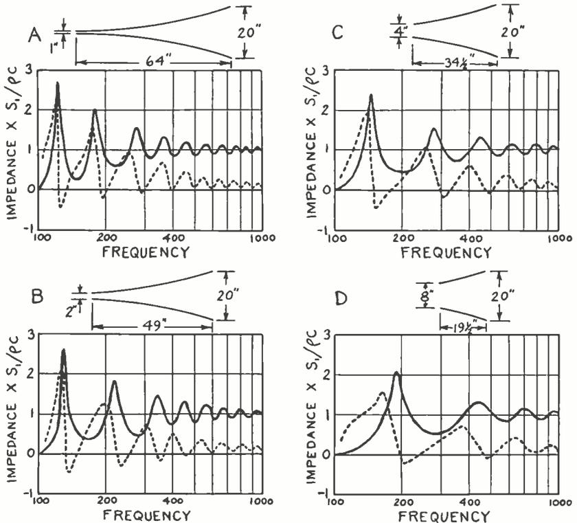
Fig. 5—The throat impedance characteristics of a group of exponential horns, with a flare cut-off of 100 cycles and a mouth diameter of 20 inches, as a function of the throat diameter.  $\rho$  density of air, grams per cubic centimeter,  $C$  velocity of sound, centimeters per second,  $S_1$  area of the throat, square centimeters.
