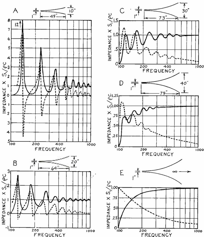
Fig. 3—The throat impedance characteristics of a group of exponential horns, with a flare cut-off of 100 cycles and a throat diameter of 1 inch, as a function of the mouth diameter,  $\rho$  density of air, grams per cubic centimeter,  $C$  velocity of sound, centimeters per second, and  $S_1$  area of the throat, square centimeters.
