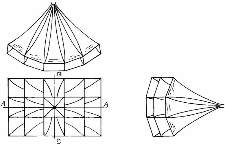
Fig. 9—Multi-horn loud speaker consisting of 15 individual exponential horns.
