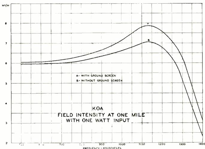
Fig. 18—Improvement obtained by use of ground screen.
