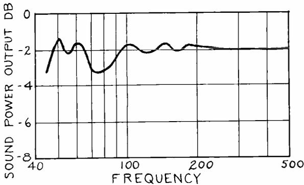
Fig. 4—Power output characteristic of a horn (horn of Fig. 5B. with all dimensions multiplied by  $2\frac{1}{2}$ ) coupled to a  $10\frac{1}{2}$  inch, 10 gram, diaphragm driven by a 5 gram aluminum voice coil in a field of 20000 gauss. Damped resistance of voice coil 20 ohms. Impedance of vacuum tube 35 ohms.
