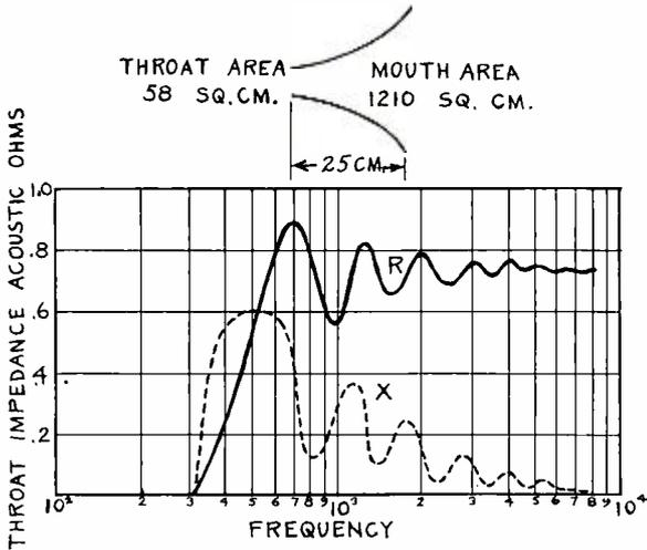
Fig. 2—Acoustic impedance characteristic, at the throat of an exponential horn of the dimensions shown and cut-off due to flare of 320 cycles, for comparison with the conical horn of Fig. 1. *R*, resistive component. *X*, reactive component.
