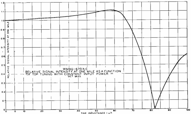
Fig. 7—Graph of one-mile signal intensity.
