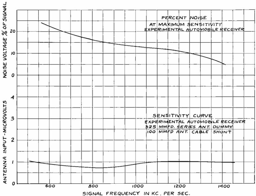
Fig. 9—Sensitivity and noise percentage curves of an experimental receiver.
