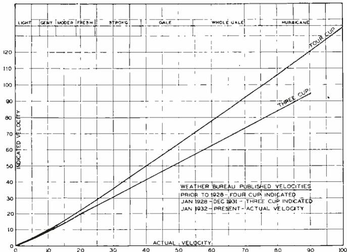
Fig. 17—Difference between actual and indicated wind velocities.
