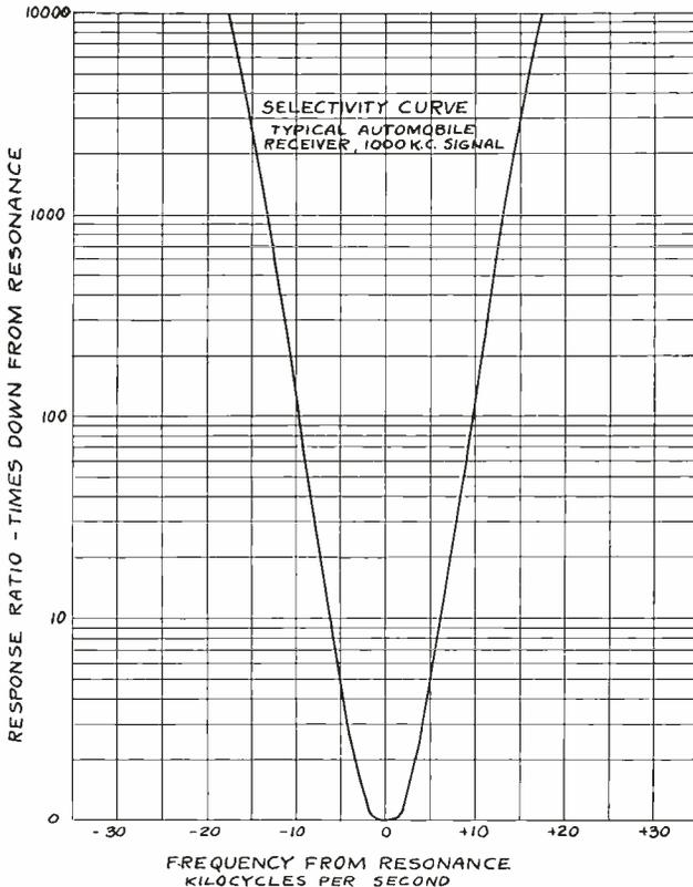
Fig. 10—Selectivity curve—modern automobile receiver.
