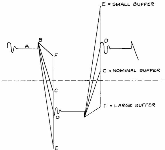
Fig. 6—Vibrator transformer primary wave form.
