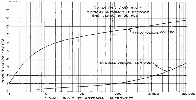
Fig. 12—Overload and automatic volume control curves of a modern automobile receiver.
