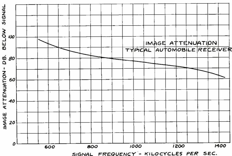
Fig. 11—Image attenuation of a typical automobile receiver.
