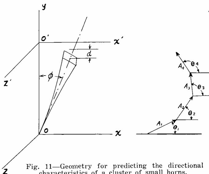
Fig. 11—Geometry for predicting the directional characteristics of a cluster of small horns.
