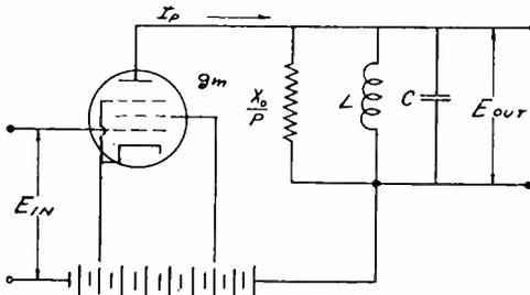
Fig. 3—Simplified schematic of a tuned amplifier.
