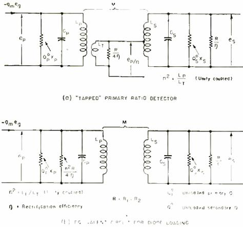
Fig. 14—The equivalent circuit for a ratio detector using a closely coupled tertiary winding (Figure 8) or a tapped primary to obtain impedance matching.
