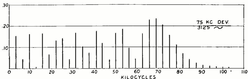
Fig. 5—Sideband amplitude.
