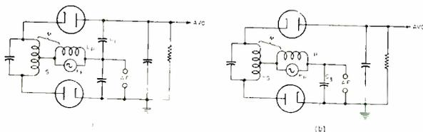
Fig. 25—Either one or two diode load condensers may be used in the ratio-detector load circuit. To obtain the same effective diode load capacitance in (b) as in (a),  $C_2$  must be equal to the sum of  $C_1$  and  $C_2$ .
