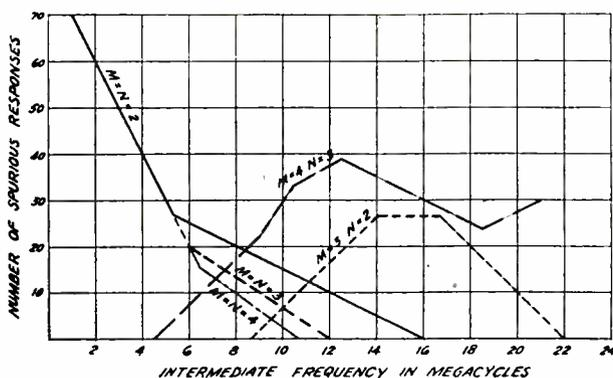
Fig. 2—Spurious responses caused by harmonic combinations of signal and oscillator versus intermediate frequency.
