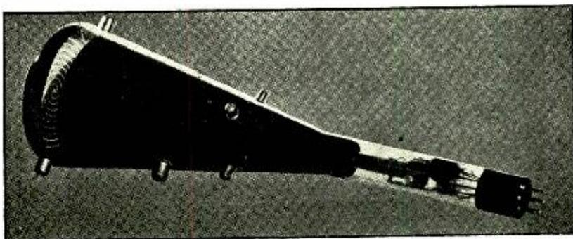
Fig. 6—Later form of the generator. The spiral anode makes five complete turns, and hence the degree of phase shift, for a given change in scanning radius, is proportionately increased.
