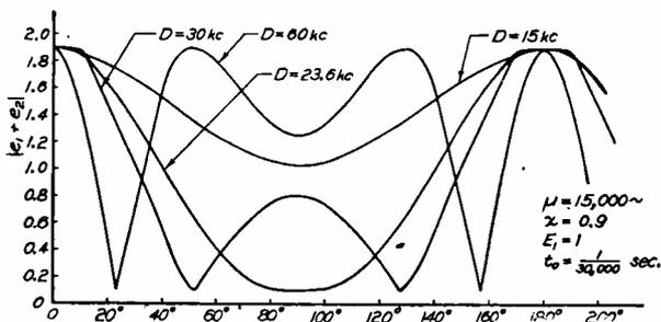
Fig. 4—Variation of carrier envelope with  $D$ .
