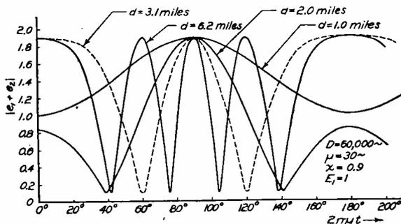
Fig. 6—Variation of carrier envelope with path difference.
