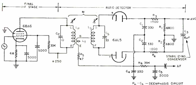
Fig. 8—A ratio-detector circuit using a balanced phase shift transformer feeding a 6AL5 double diode. The closely coupled tertiary winding  $L_T$  is wound over the  $B+$  end of the primary to provide impedance matching and improved sensitivity.
