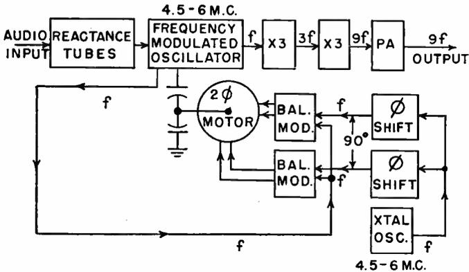
Fig. 7—Preliminary Frequency Control FM Exciter
