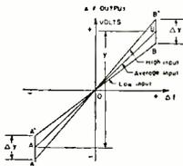
Fig. 21—Effect of amplitude modulation on the output of a balanced detector. If  $100M = \% \text{ amplitude modulation of the input signal}$ , then  $\Delta y = yM$ , and  $\Delta y/y = M$ . This is referred to as a balanced a-m component.
