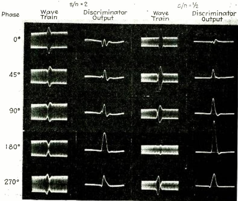
Fig. 5—Oscillograms of noise and discriminator output with carrier tuned to edge of the pass band.
