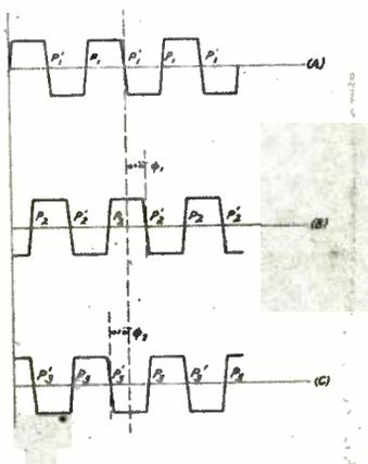
Fig. 4—Square wave outputs of the generator, lettered to correspond with the scanning circles shown in Fig. 2, opposite. The phase shift results in frequency modulated waves when the signal is passed through a frequency multiplier.
