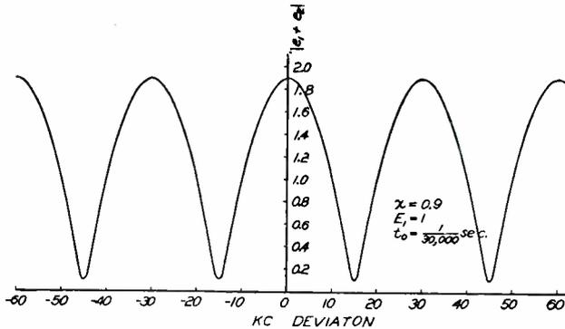
Fig. 7—Variation of amplitude with deviation.
