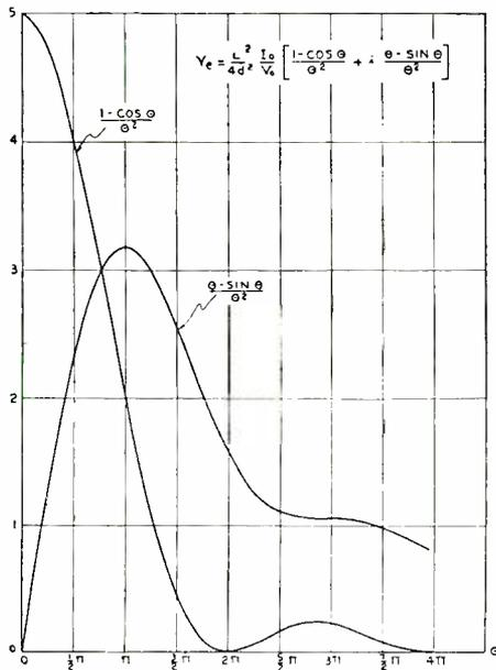
Fig. 2—Electronic admittance as a function of  $\theta$ .
