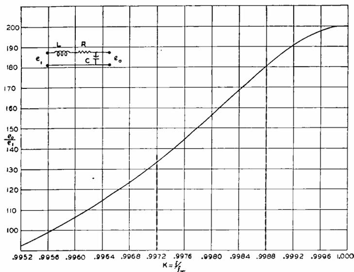
Fig. 8—One side of the discriminator resonance curve.
