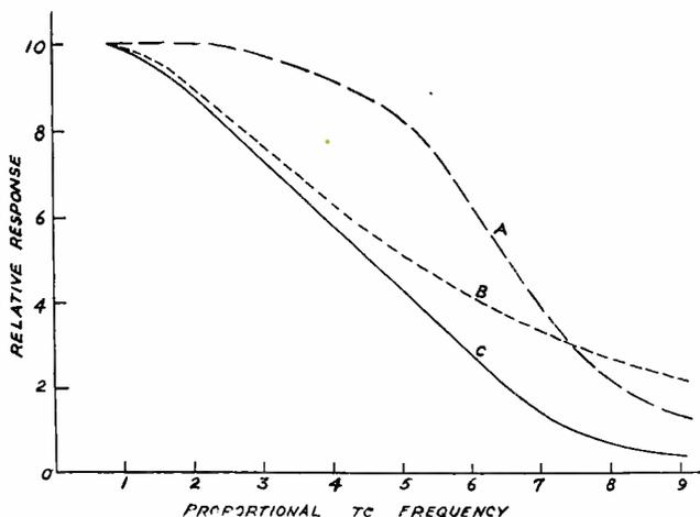
Fig. 4—Frequency-response curves of wide-range frequency discriminator.
