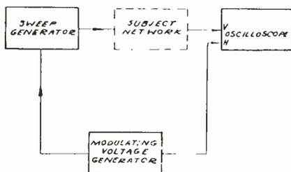
Fig. 1—Block layout of a visual network test and alignment position.
