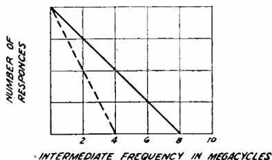
Fig. 3—Interference caused by the image response and by two stations separated by the intermediate frequency versus intermediate frequency.
