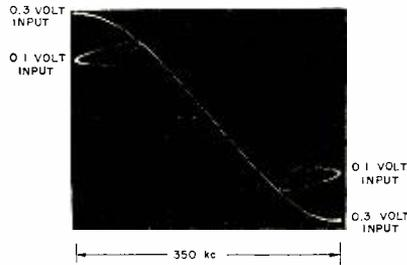
Fig. 11—Effect of reduction in the input signal. The stabilizing voltage is held constant at a level corresponding to the 0.3-volt input signal. Note the reduction in peak separation for decreasing input signal.
