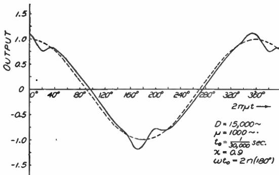
Fig. 22—Distorted audio output.
