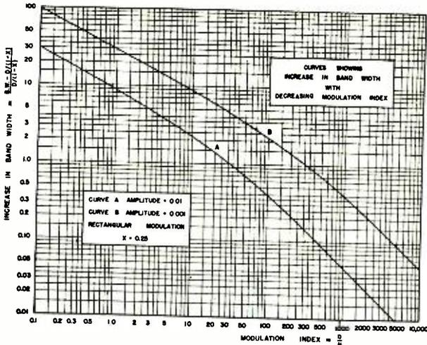
Fig. 12—Variation of bandwidth with modulation index.
