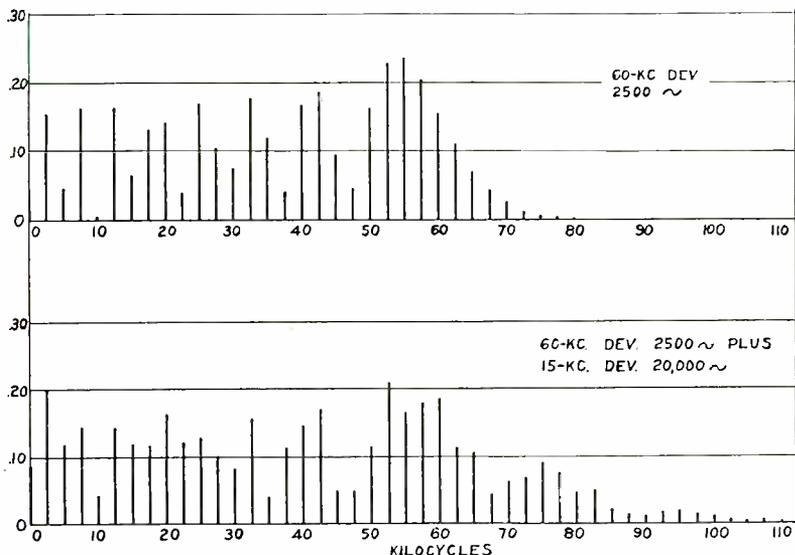
Fig. 6—Sideband amplitude.
