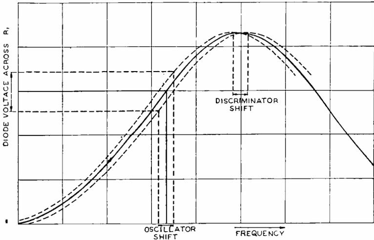
Fig. 4—Graphical representation of both oscillator and discriminator combined modulations in the push-pull FM system.
