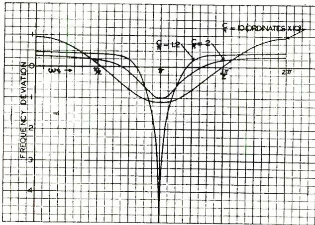
Fig. 4—Calculated wave forms showing the distortion produced on the instantaneous frequency deviation of the wave composed of the combination of the carrier and a single noise component.  $C/n$  = ratio between the peak voltage of the carrier and the peak voltage of the noise component.
