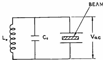
Fig. 4—Equivalent lumped circuit of resonant system.
