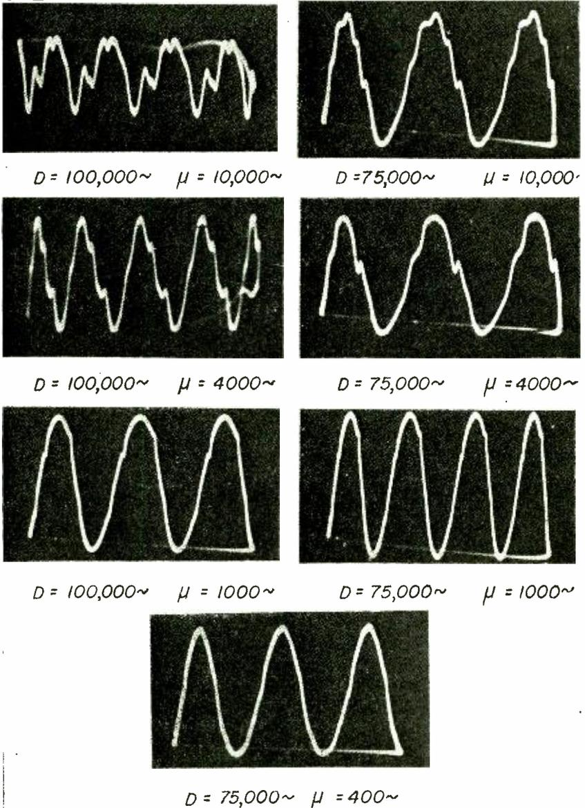
Fig. 23—Oscillograms showing distortion.
