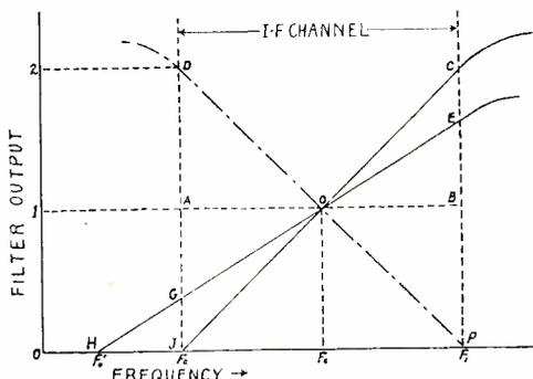
Fig. 2—Ideal sloping filter characteristics.
