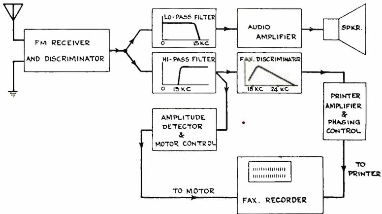
Fig. 7—Receiver block diagram for multiplex operation of aural and facsimile.
