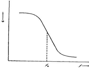
Fig. 9—Input capacitance of discriminator.
