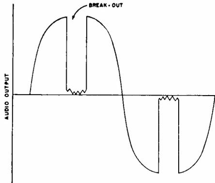
Fig. 7—Breakout characteristic.
