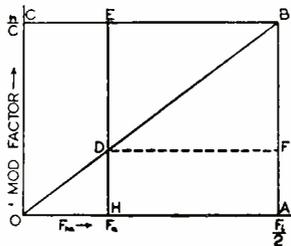
Fig. 3—Amplitude and frequency modulation receiver noise spectra. *OBA* = frequency modulation detector output. *ODH* = frequency modulation receiver output. *OCEH* = amplitude modulation receiver output.
