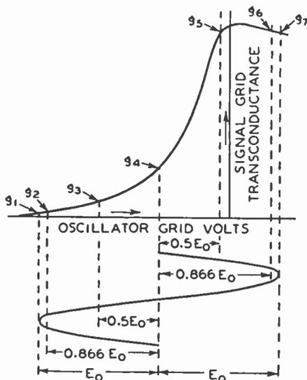
Fig. 2—a. Points used for 30-degree analysis of conversion transconductance.
