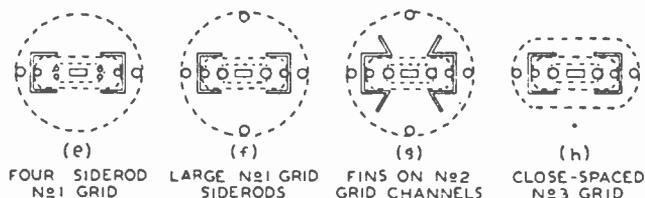
Fig. 20—Cross-sectional views of improved mixers designed for outer-grid injection of oscillator. The views show only the portions of the tube inside of and including the oscillator injection grid.
