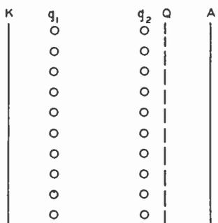
Fig. 8—Determination of amplification factor and inter-electrode capacitance in multigrid structures by use of the Q plane.
