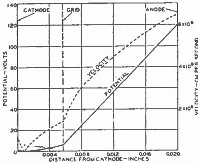
Fig. 1—Potentials and velocities in a parallel-plane triode.
