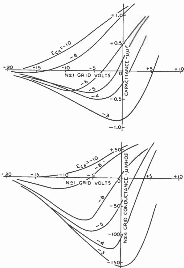
Fig. 10—Signal-grid (grid No. 4) admittance of a typical mixer designed for inner-grid injection of oscillator at 31.5 megacycles. Curves taken with no oscillator voltage applied. Data represents electronic admittance only (i.e., "cold" values were subtracted from measured values before plotting).
