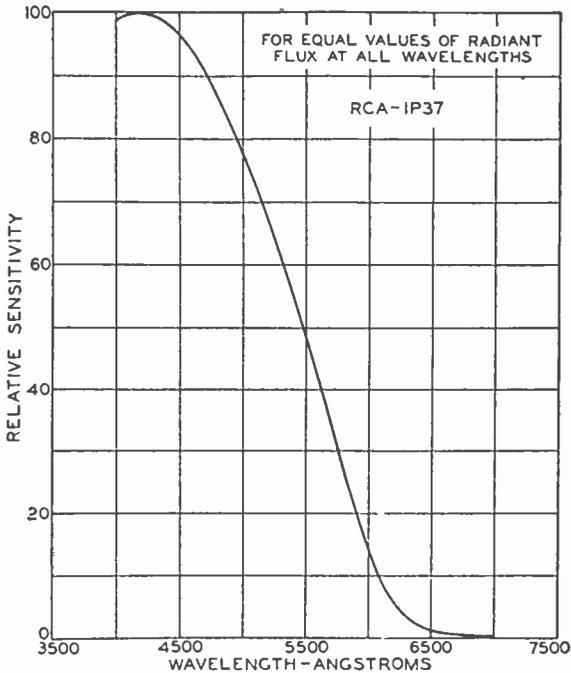
FIG. 1. Spectral sensitivity of phototube having *S-4* response.
