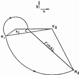
Fig. 5—The graphical construction giving the circular motion produced by the transverse field of Fig. 3. The radius vector  $CR_2$  indicates the phase and magnitude of the motion at the instant the electric field ceases to act.
