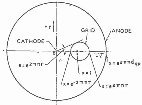
Fig. 4—Cross section of the triode of Fig. 3 transformed from the  $w$  plane to the  $z$  plane.
