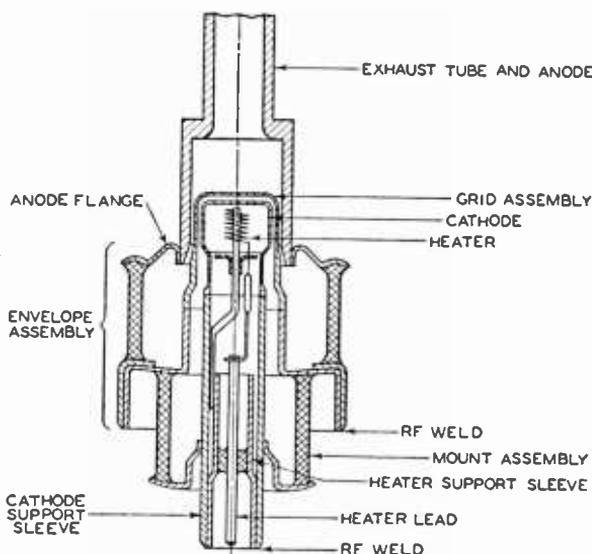
Fig. 1—Cross-sectional view of the 5588.
