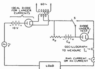
Fig. 10—Circuit for measuring equivalent diode resistance values.
