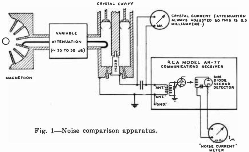
Fig. 1—Noise comparison apparatus.
