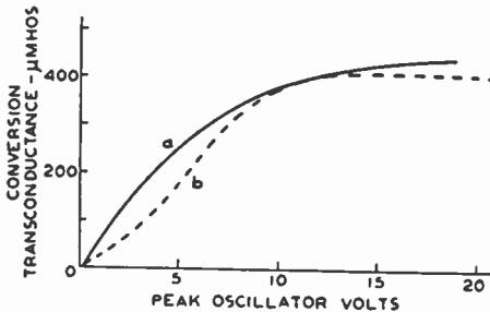
Fig. 14—Conversion transconductance of a typical mixer designed for outer-grid injection of oscillator. Signal-grid bias,  $E_{c1} = -3$  volts. Curve *a* corresponds to fixed No. 3 grid bias,  $E_{c2} = -8$  volts. Curve *b* corresponds to bias obtained through a 50,000-ohm grid leak.
