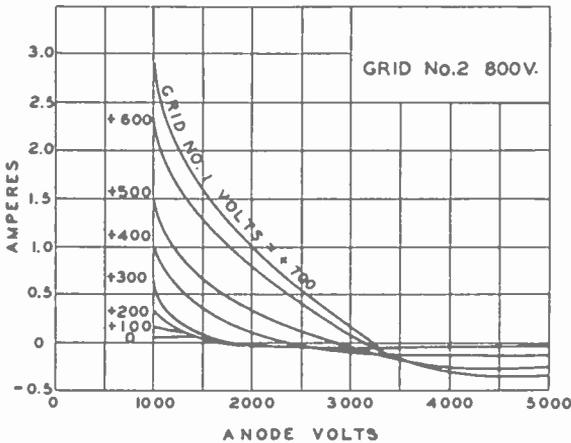
Fig. 10—No. 2 grid characteristics for each unit.
