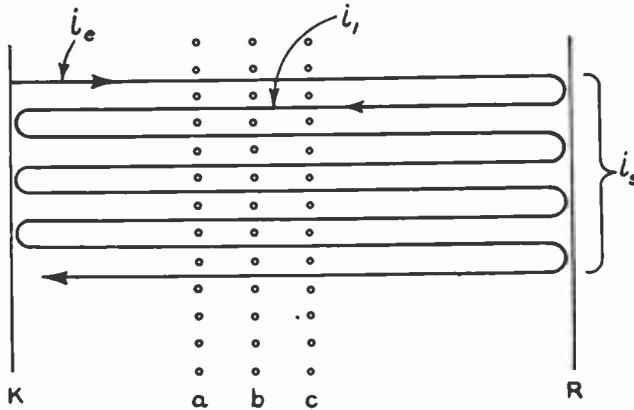
Fig. 2—Schematic electron paths in a triple-grid reflex oscillator, showing the effective current  $i_e$  and the built-up space current  $i_s$ , due to multiple transits, between cathode  $K$  and reflector  $R$ .
