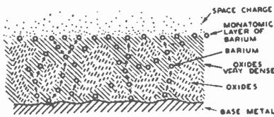
Fig. 11—Representation of cathode coating.
