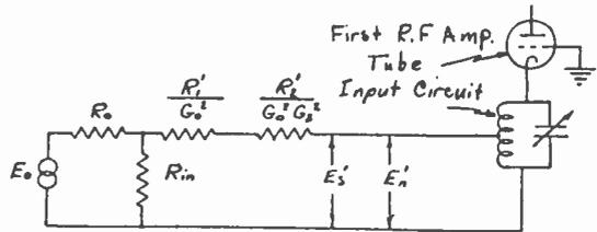
and the noise-equivalent resistances of the first and second radio-frequency amplifier tubes.
