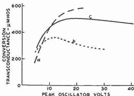
Fig. 9—Conversion transconductance of a typical mixer designed for inner-grid injection of oscillator. Signal-grid bias = -3 volts. *a*, fixed-bias operation of oscillator grid; *b*, oscillator-grid bias obtained through high-resistance grid leak; *c*, oscillator-grid bias obtained through a 50,000-ohm grid leak.
