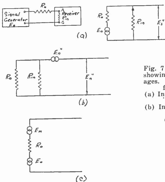
Fig. 7 — Receiver input circuit showing noise and signal voltages. 4KT method of noise-factor measurement.
