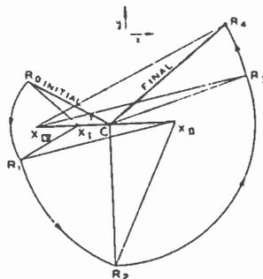
Fig. 7—The graphical construction for the transverse field of Fig. 6. The radius vector representing the initial circular motion is  $CR_1$ , its magnitude being drawn proportional to the actual radius in centimeters, determined by
