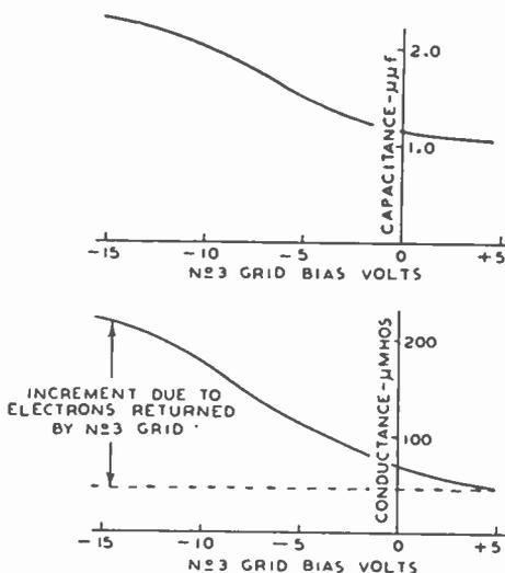
Fig. 16—Signal-grid (grid No. 1) admittance of typical mixer designed for outer-grid injection of oscillator. Data taken at 31.5 megacycles with no oscillator voltage applied.  $E_{c1} = -3$  volts,  $E_{c2 \text{ and } c3} = 100$  volts,  $E_k = 250$  volts.
