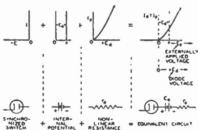
Fig. 1—Characteristics and equivalent circuit for high-vacuum diodes.
