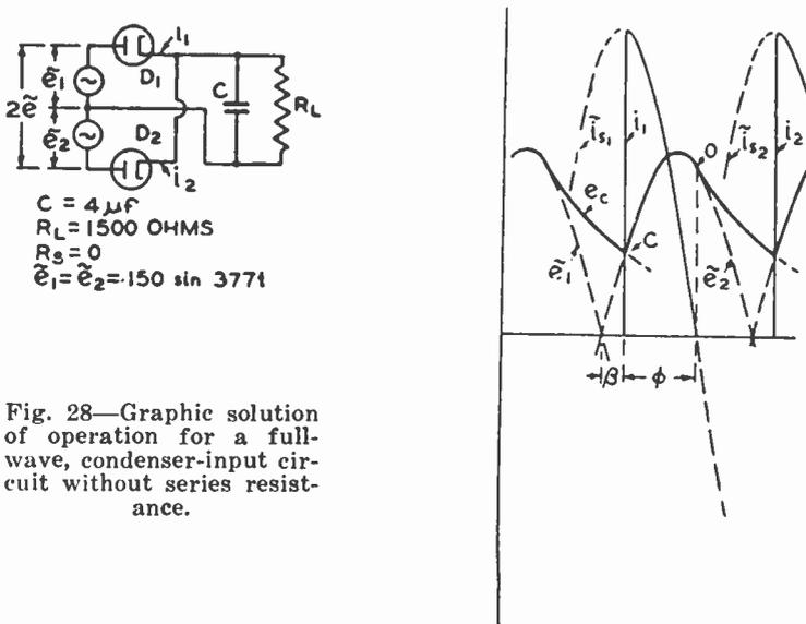
Fig. 28—Graphic solution of operation for a full-wave, condenser-input circuit without series resistance.
