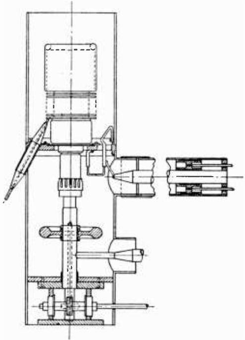
Fig. 4—Cross section of the “half-wave” oscillator circuit.
