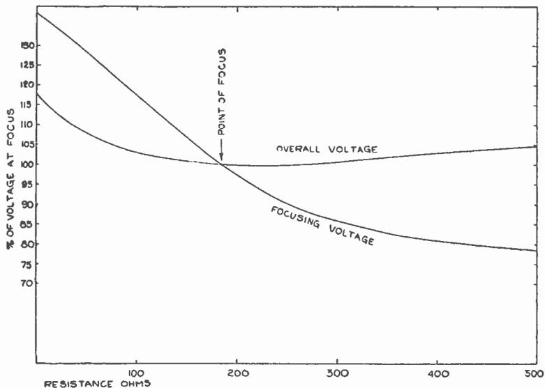
Fig. 20—Voltage control of type S-2 Power Supply.
