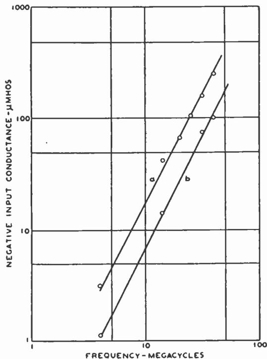
Fig. 11—Signal-grid (grid No. 4) conductance of a typical mixer designed for inner-grid injection of oscillator. Lines are drawn with slope of 2. Curve *a* taken with  $E_{c1} = 0$ ,  $E_{c4} = -3$  volts. Curve *b* taken with  $E_{c1} = -6$ ,  $E_{c4} = -6$  volts.
