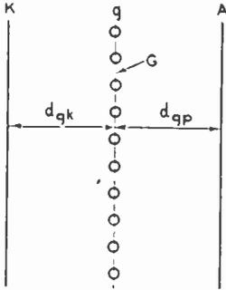
Fig. 5—Triode with equivalent plane G at grid.
