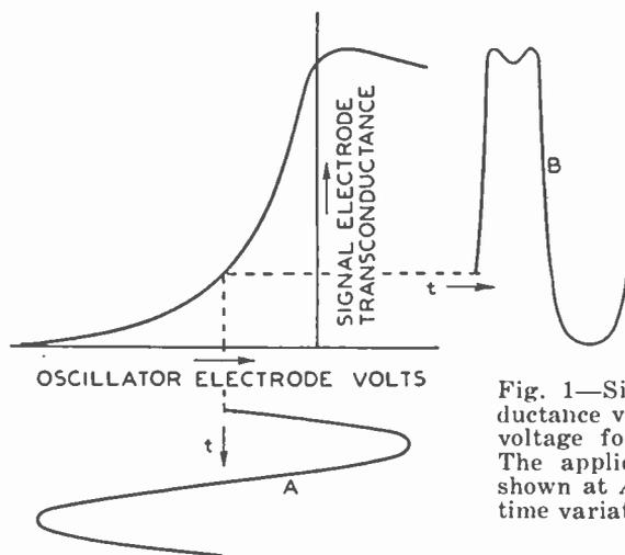
Fig. 1—Signal-electrode transconductance versus oscillator-electrode voltage for a typical mixer tube. The applied oscillator voltage as shown at A and B is the resulting time variation of transconductance.
