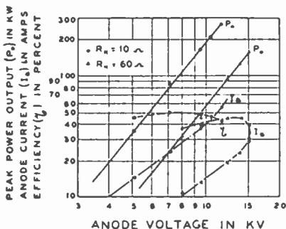
Fig. 5—Typical pulse operating data at 600 Mc.
