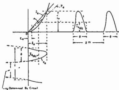
Fig. 2—Graphic evaluation of equivalent diode resistance values.
