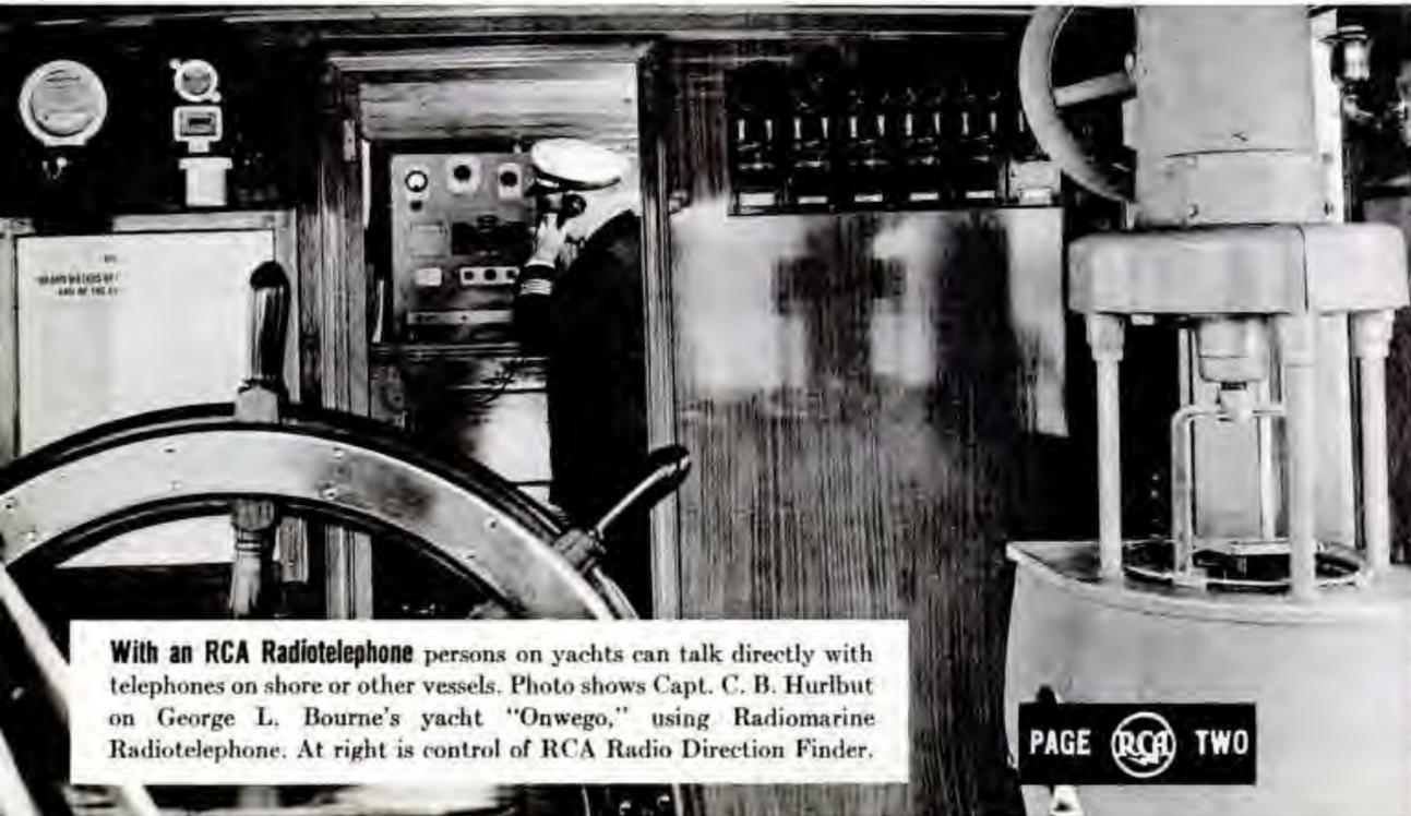
With an RCA Radiotelephone persons on yachts can talk directly with telephones on shore or other vessels. Photo shows Capt. C. B. Hurlbut on George L. Bourne's yacht "Onwego," using Radiomarine Radiotelephone. At right is control of RCA Radio Direction Finder.
