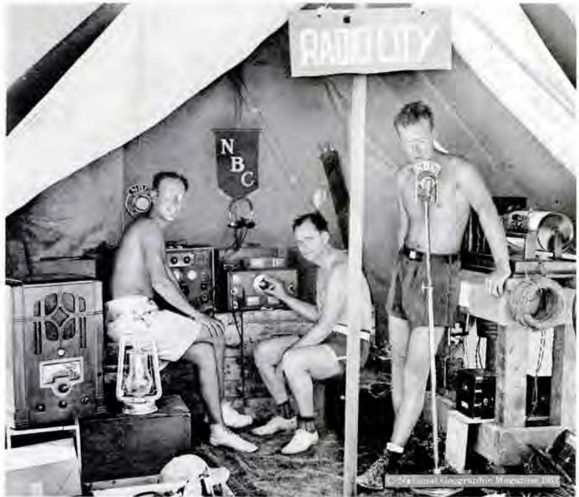
**"Radio City," South Pacific model**—RCA services joined hands to put historic broadcast from Canton Island on NBC network. The speakers' voices were carried by RCA ultra-high frequency transmitter from the Island to the navy vessel Avocet, lying off shore. From there a special RCA transmitter sent them to RCA
