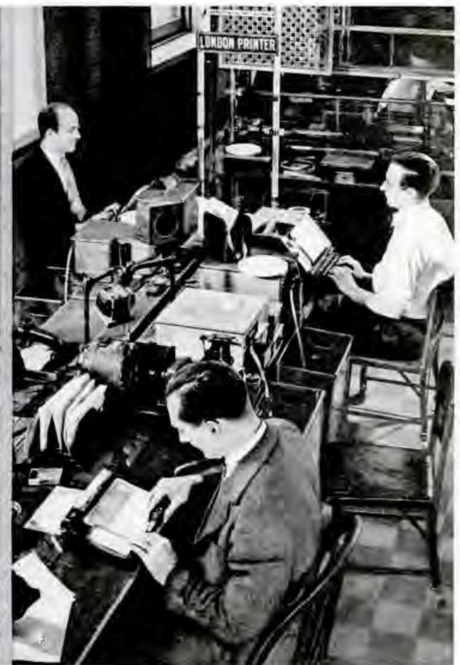
A single radio wave now speeds RCA service by carrying three separate messages. Pictures above show how this is done. (1) Three operators send messages as usual. (2) These messages pass to swiftly rotating device called a "multiplex." This turns so quickly that it picks up the code impulses from each operator in order, even
