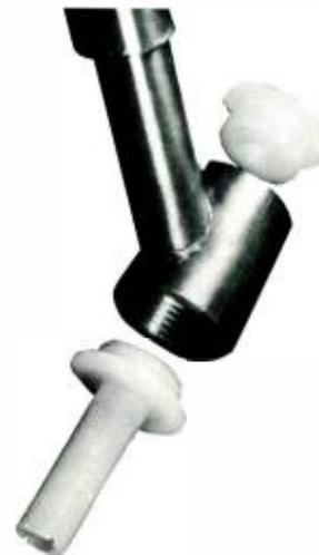
A close-up exploded view of the chip collector, shown in Fig. 2, clearly indicates the simple three-part construction of the tool, which consists of a brass body, a top adaptor, and a bottom adaptor. The adaptors may be fabricated from Delrin, Nylon, Teflon, or other low-friction, abrasive-resistant materials.
