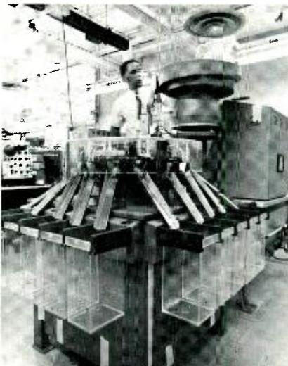
Production equipment sometimes combines functions. In this case one machine tests and sorts silicon rectifiers.
