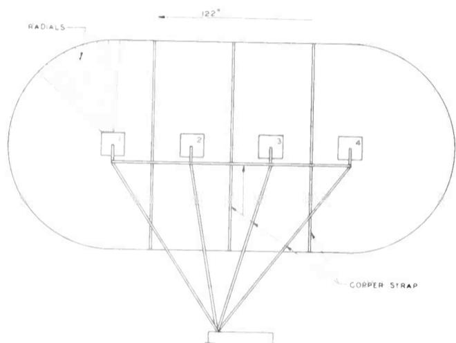
FIG. 5. (Above) Sketch showing approximate layout of antenna and ground system of WLOS and WLOS-FM.
