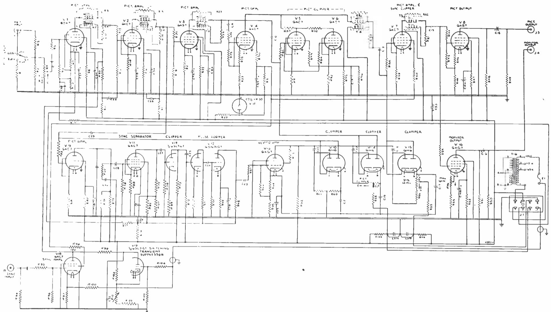
FIG. 6. Schematic diagram of the Type TA-5B Stabilizing Amplifier.
