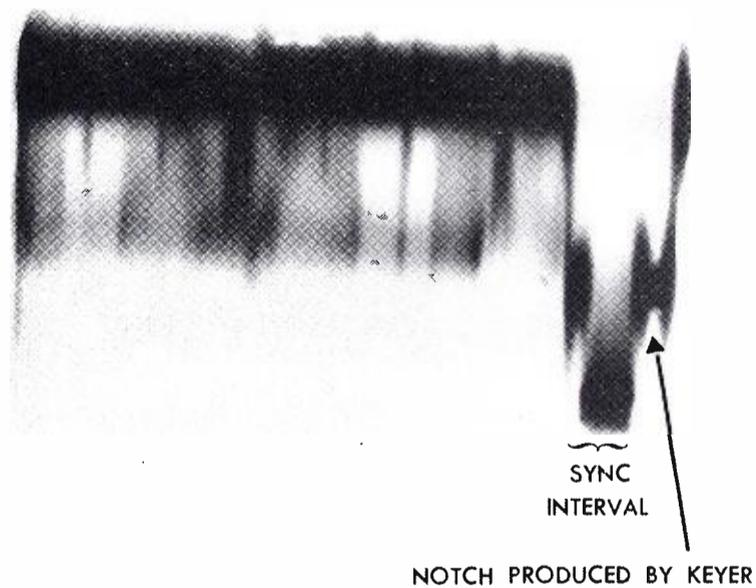
**FIG. 13.** An oscillogram of the output signal shown in Figure 12 except that a saw-tooth sweep frequency of 15750 cycles was used. The horizontal blanking interval appears at the right. The notch in this interval is caused by the clamp circuit effecting a low-impedance path between grid and ground in the amplifier and thus suppressing the hiss signal.
