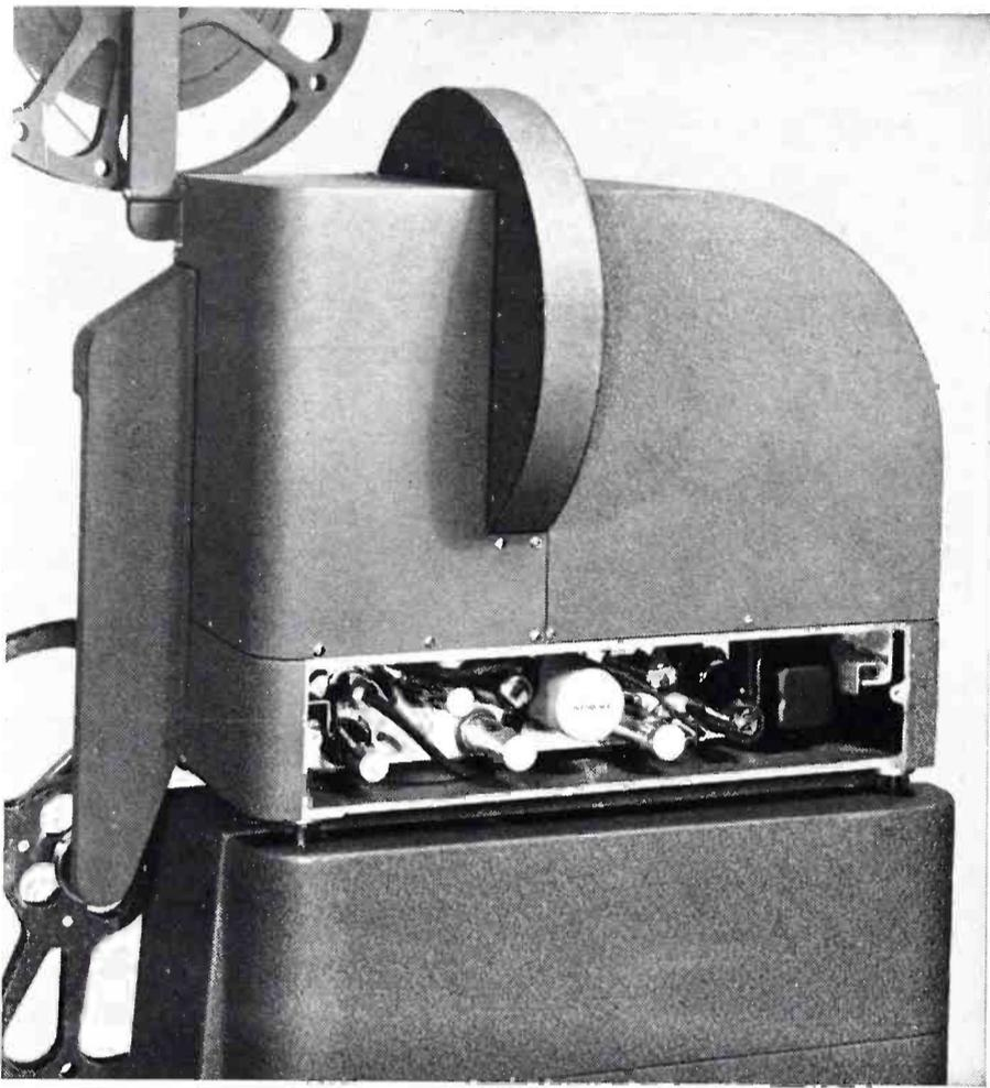
**FIG. 7.** The amplifier, a self-contained unit, is shock-mounted in a recess in the base casting. Cover of the amplifier compartment, held in place by thumbscrews, is easily removed for servicing.
