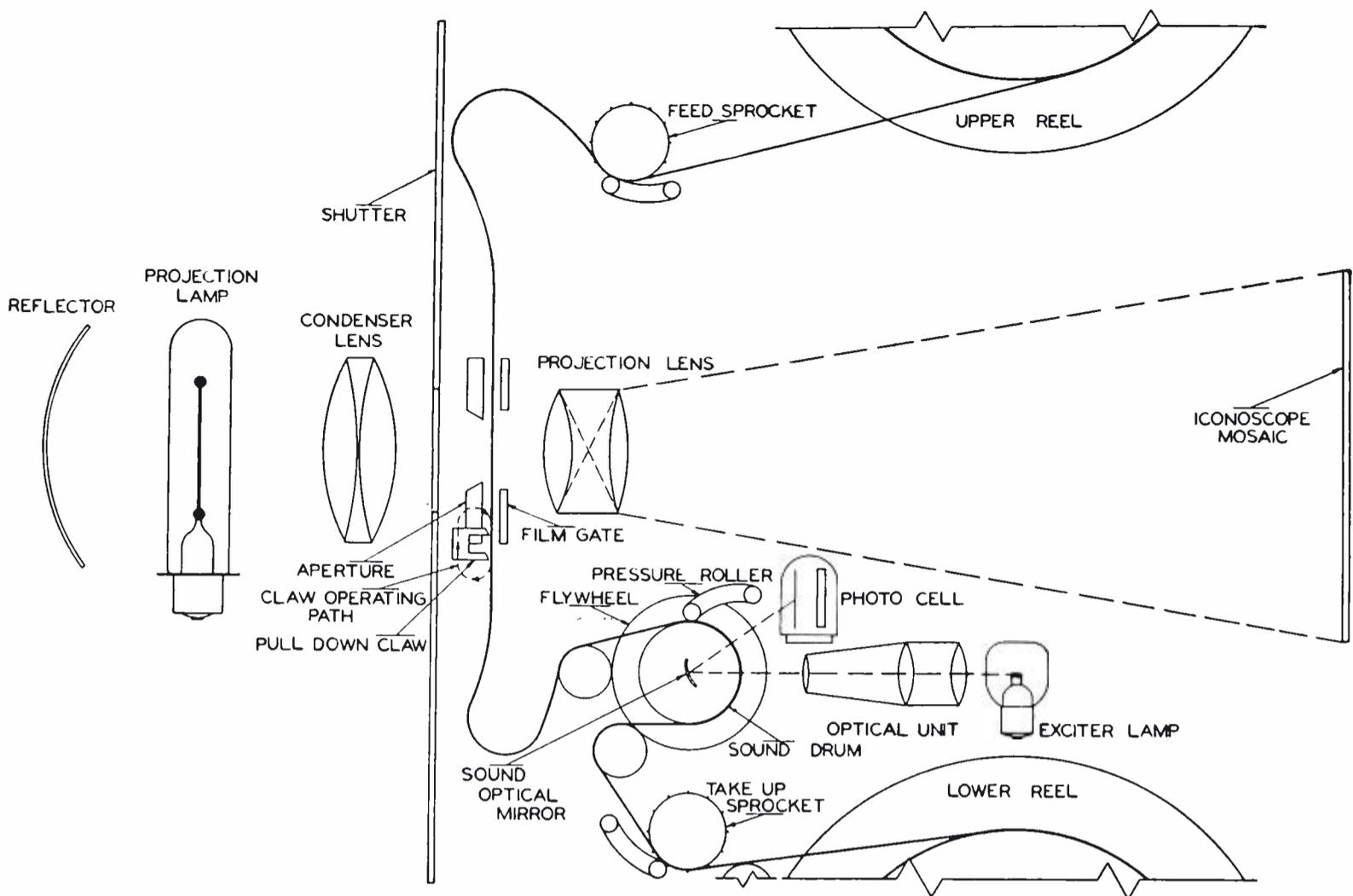
FIG. 3. Diagram of the optical and film feed systems of the TP-16A Projector.
