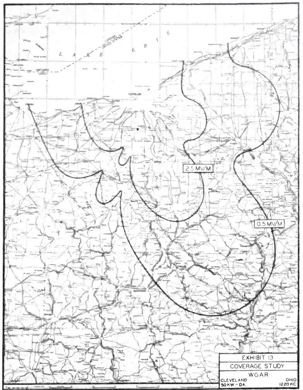
FIG. 22. Computed coverage of new WGAR 50 KW transmitter and directional system described in accompanying article.
