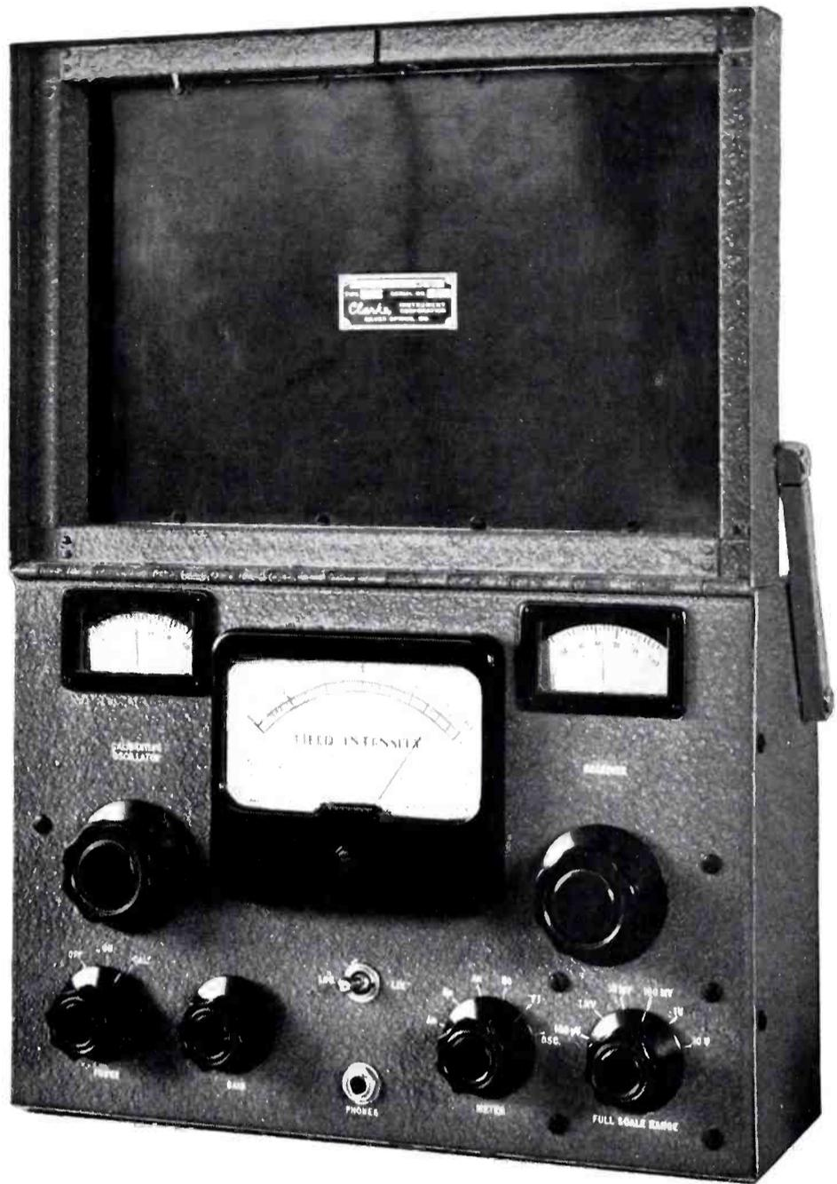
**FIG. 1.** (above) *The WX-2A Field Intensity Meter is an extremely convenient, entirely self-contained instrument providing direct readings with high accuracy at frequencies in the AM broadcast band.*
