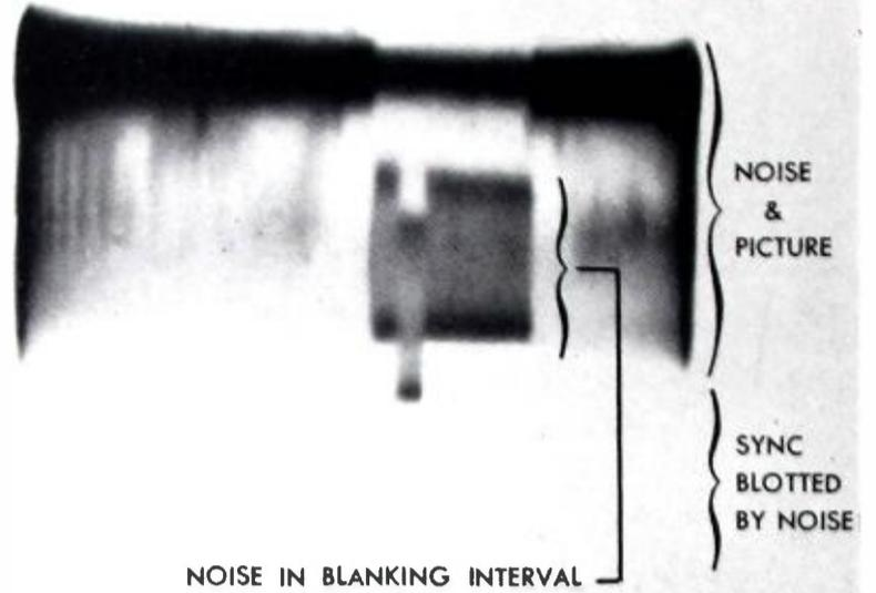
FIG. 9. An oscillogram of a typical noise-free signal generated by a Monoscope camera. The sweep frequency is 30 cycles, therefore, the gap in the center is a vertical blanking interval.
