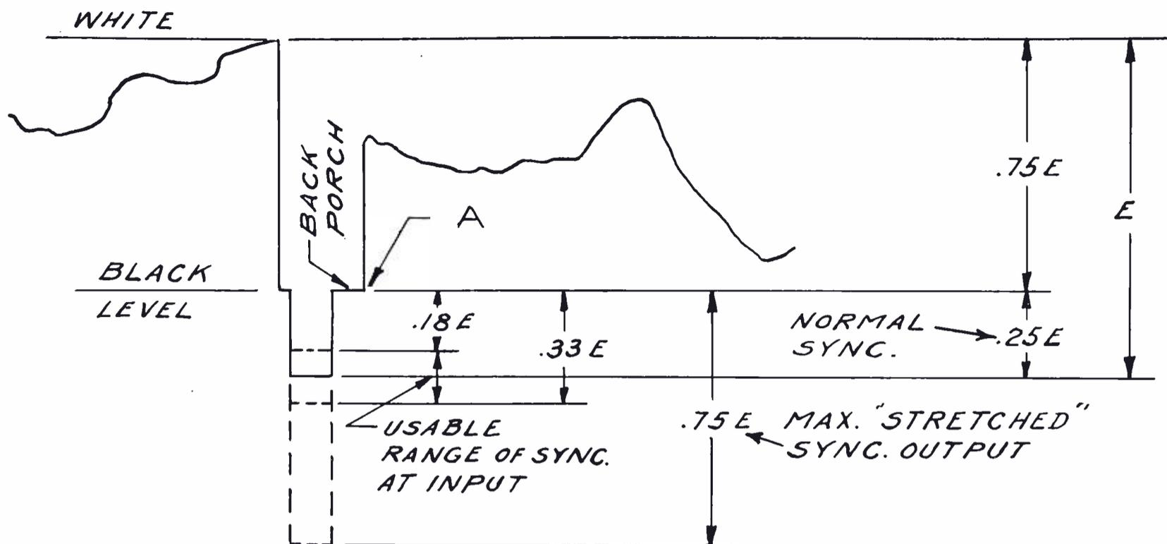
FIG. 5. The drawing above shows the possible sync-to-picture voltage ratios in the stabilizing amplifier. Also shown is the "back porch" interval of the blanking pulse, during which the clamping action takes place.
