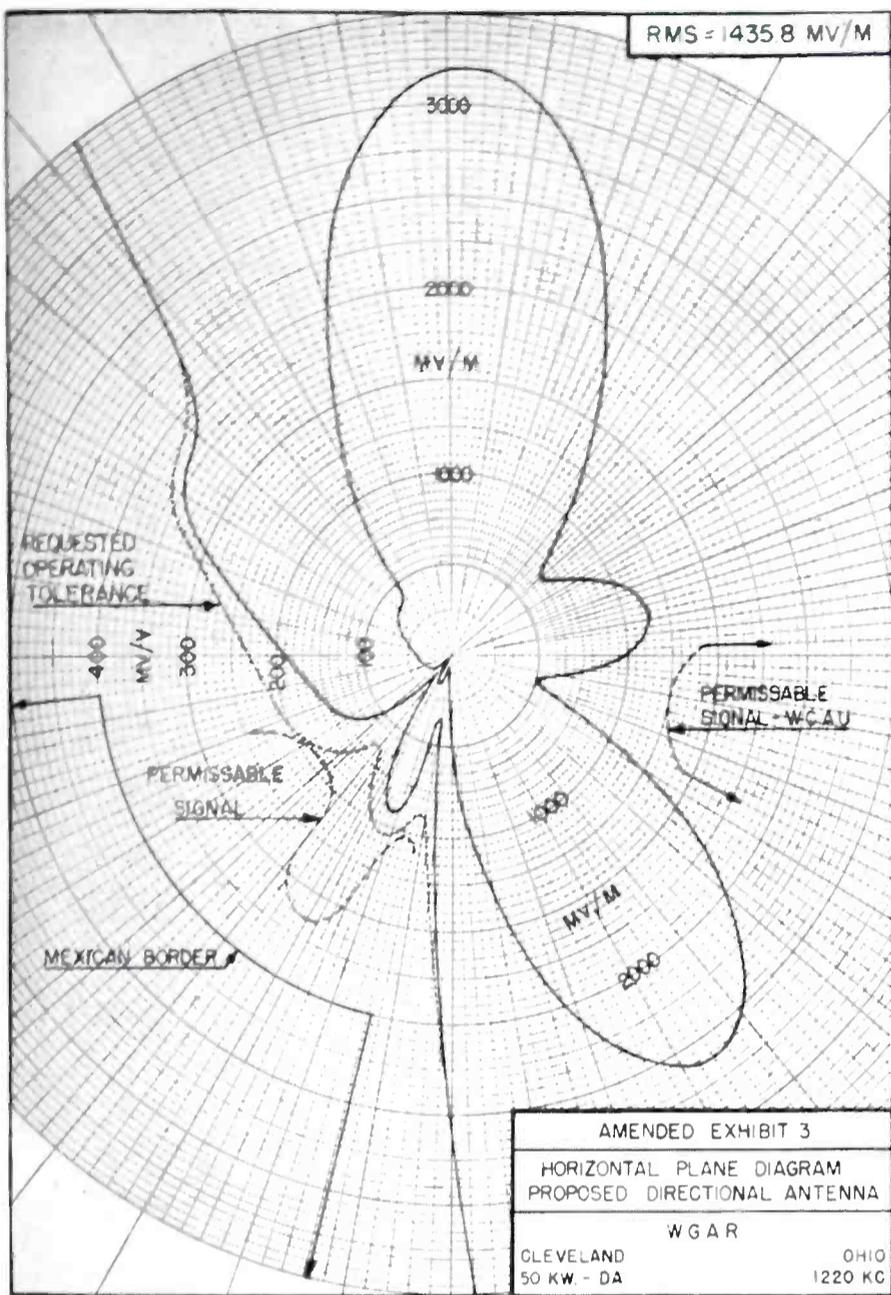
FIG. 21. Computed horizontal polar diagram of the unattenuated field at one mile for the five-tower WGAR array.
