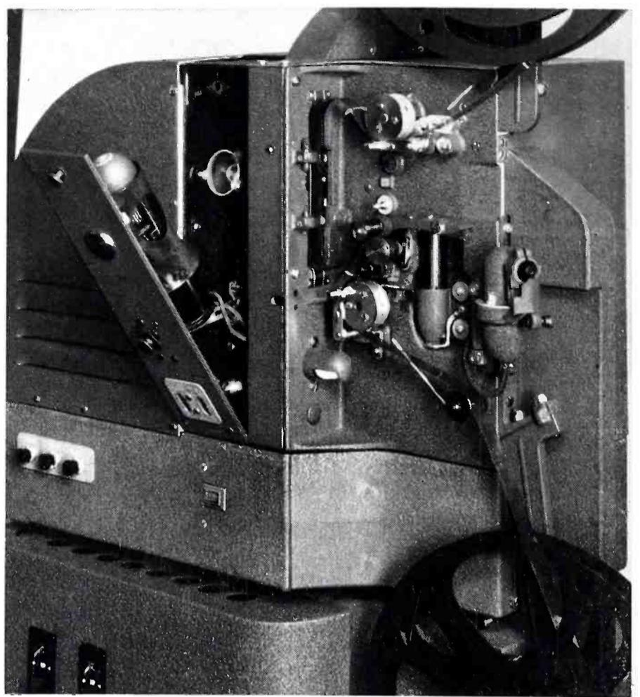
**FIG. 8.** Another feature which contributes to maintenance operation is the fact that reflector, condenser lens and projector lamp are instantly accessible for inspection and cleaning.
