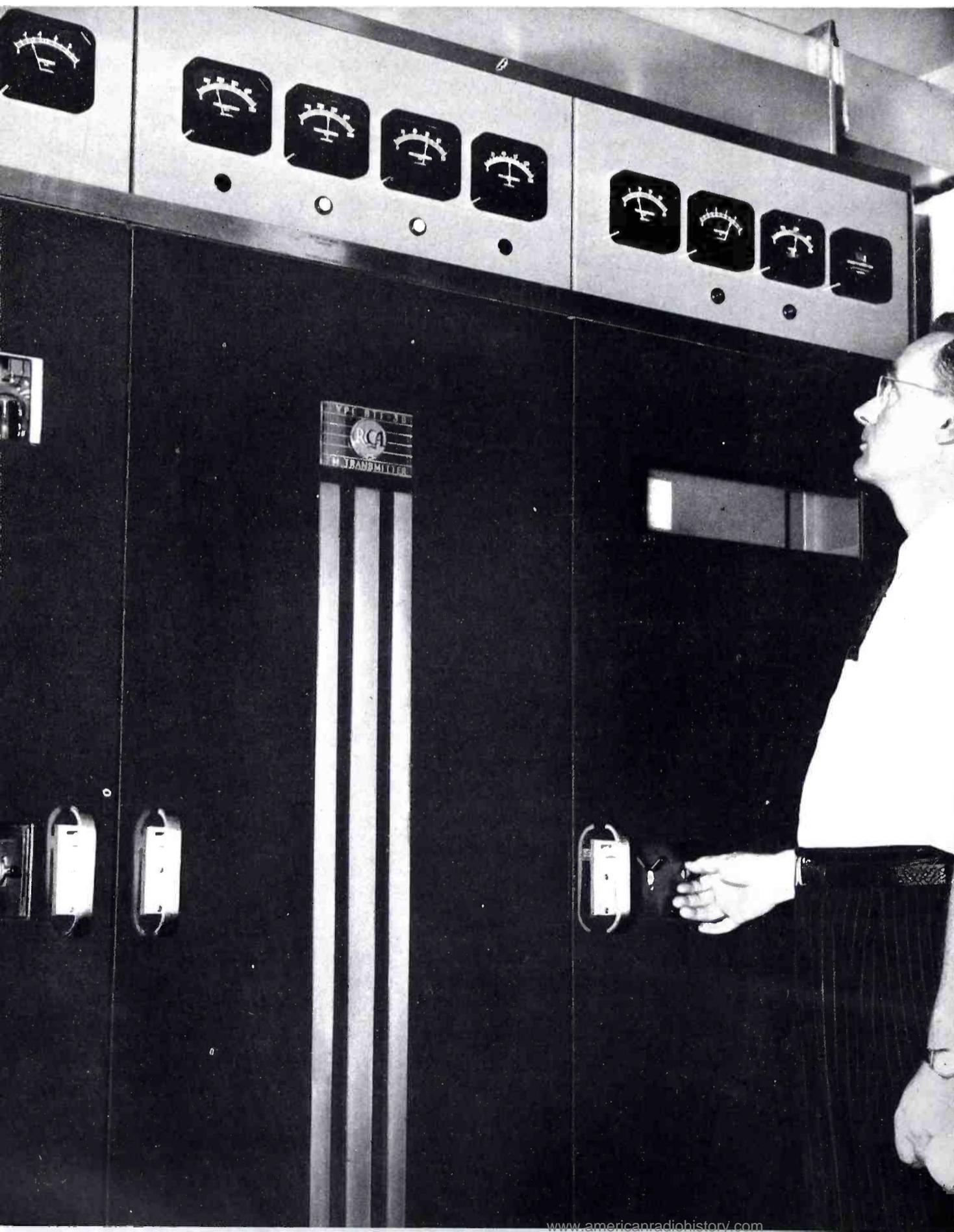
**FIG. 1.** (Left) KRON's 3 kilowatt FM transmitter, RCA type BTF-3B, which is setting the standard for FM quality in San Francisco. The clean carrier and absence of noise has enabled FM dealers to demonstrate the superiority of FM. The transmitter is now located in the Chronicle building, a temporary site.
