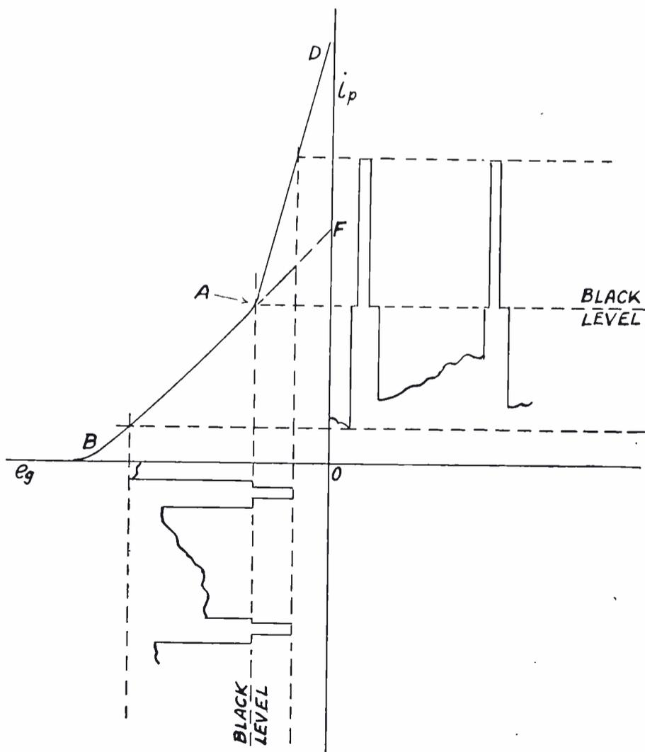
FIG. 4. Characteristic curve showing operation of the sync stretching stages of the amplifier. Tubes V5 and V6 amplify only the sync portion of the video signal as indicated by portion AD of the curve.
