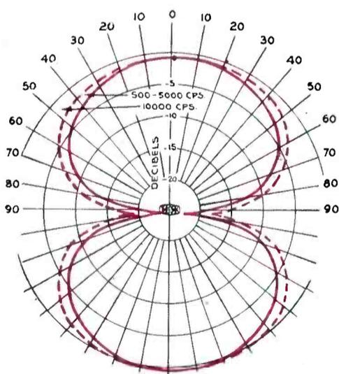
**Directional characteristics of a typical KB-2C microphone.**
