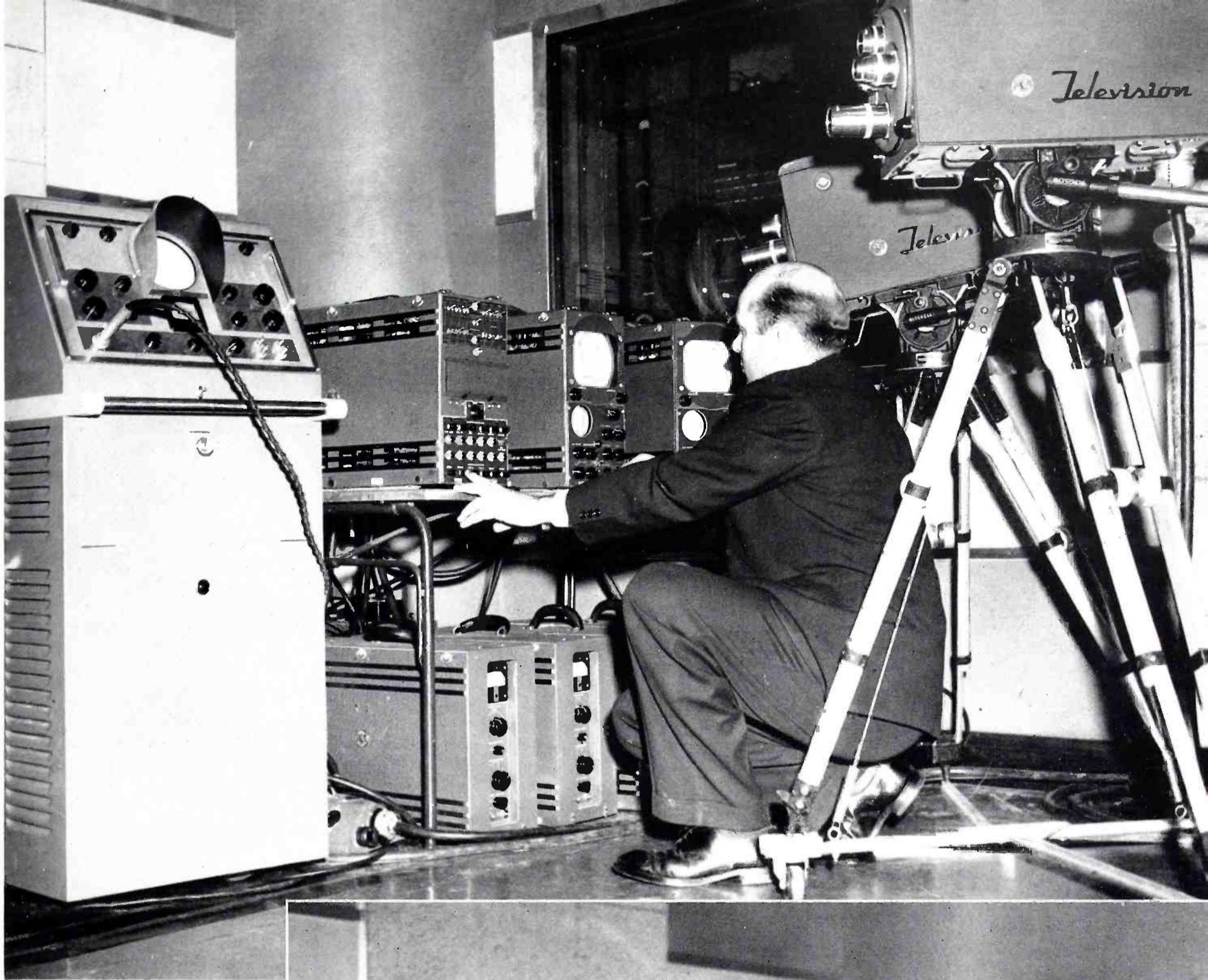
**FIG. 2.** (above) In December 1946, WOW purchased the two RCA Image-Orthicon Camera Chains shown above in the WOW studio. Unit at left is an RCA 715-B Oscilloscope which is especially designed for television testing.
