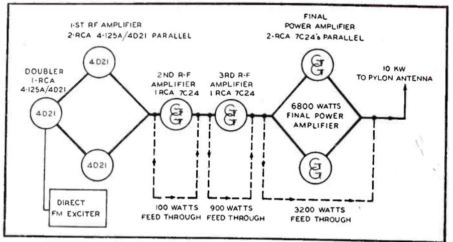
FIG. 4. (above) Because RCA Grounded-Grid circuits put tube input and output voltages in series . . . and in phase, power output is additive. The grounded-grid drivers contribute nearly 3200 watts to the total power output. This allows the use of smaller, less expensive tubes in the final P. A.
