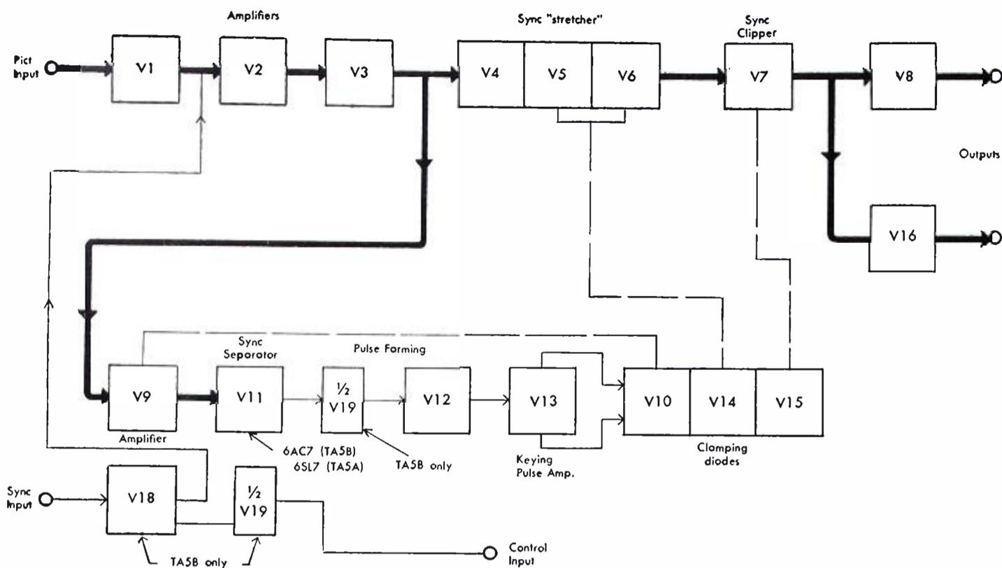
FIG. 3. Circuits of the Stabilizing Amplifier are shown here in block diagram form. Video circuits are indicated by the heavy lines; pulse-forming and clamping circuits are shown by the broken lines.
