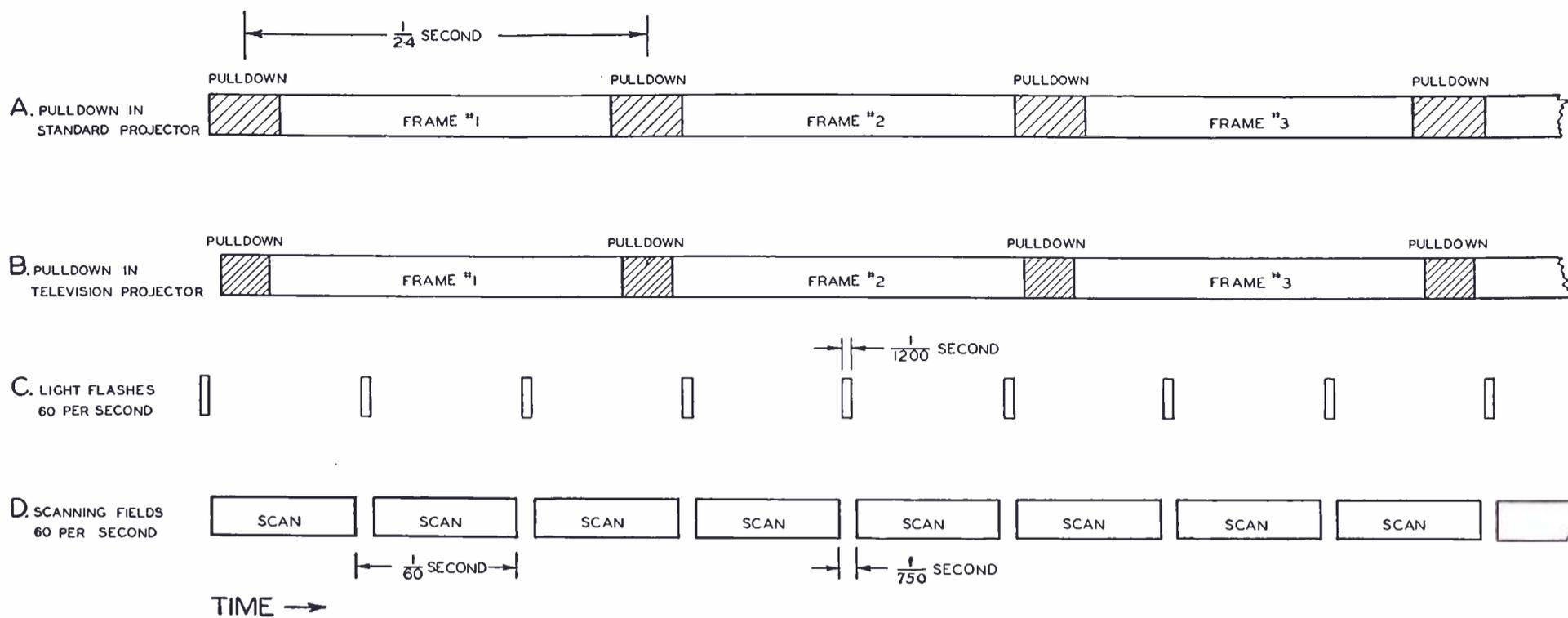
**FIG. 4.** This diagram illustrates the time relationship of the framing, light and scanning sequences employed in the RCA type TP-16A 16mm Television Film Projector. Line A shows the "pull-down" interval in a standard 16mm film projector (Type PG-201). The "pull-down" interval is about one-sixth of the total frame cycle. Line B illustrates the effect of speeding up the "pull-down" in the TP-16A Projector. The "pull-
