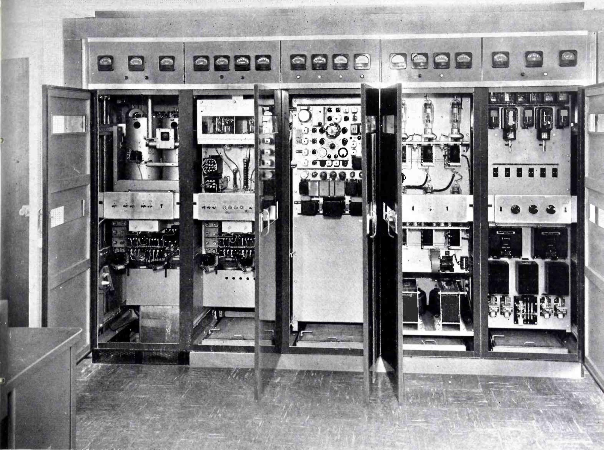
**FIG. 2.** (above) *Front view of the 10 KW FM Transmitter in which access doors are opened to show (cabinets from left to right): Final 10 KW amplifier, Low Power R-F (250 watt, 1 and 3 KW), Direct FM Exciter, H-V Rectifier and Power and Control sections. All controls and switches, necessary for normal operation, are conveniently located at hand level.*
