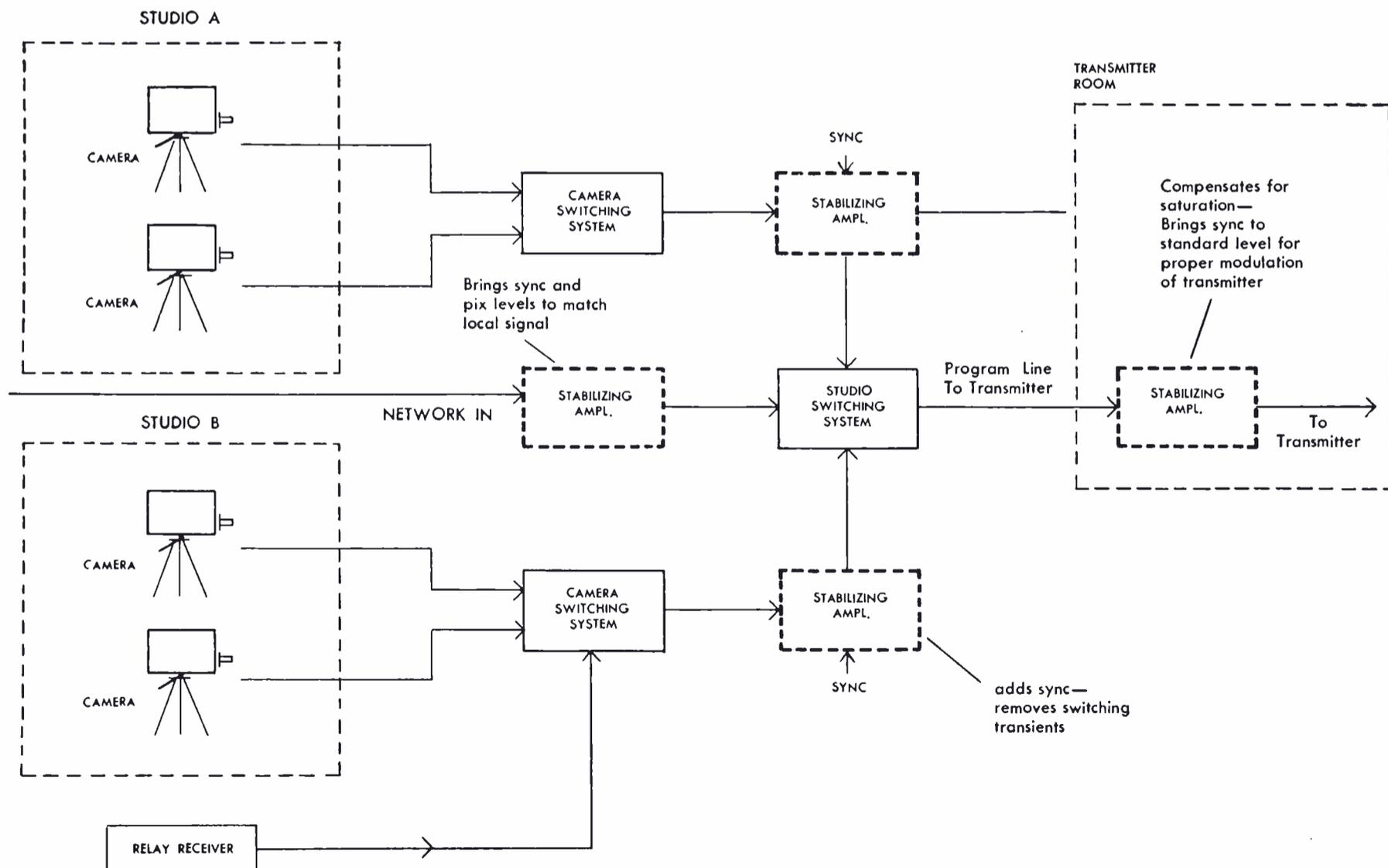
FIG. 1. Block Diagram (above) shows a few typical applications of the Stabilizing Amplifier in the television studio and in the transmitter room.
