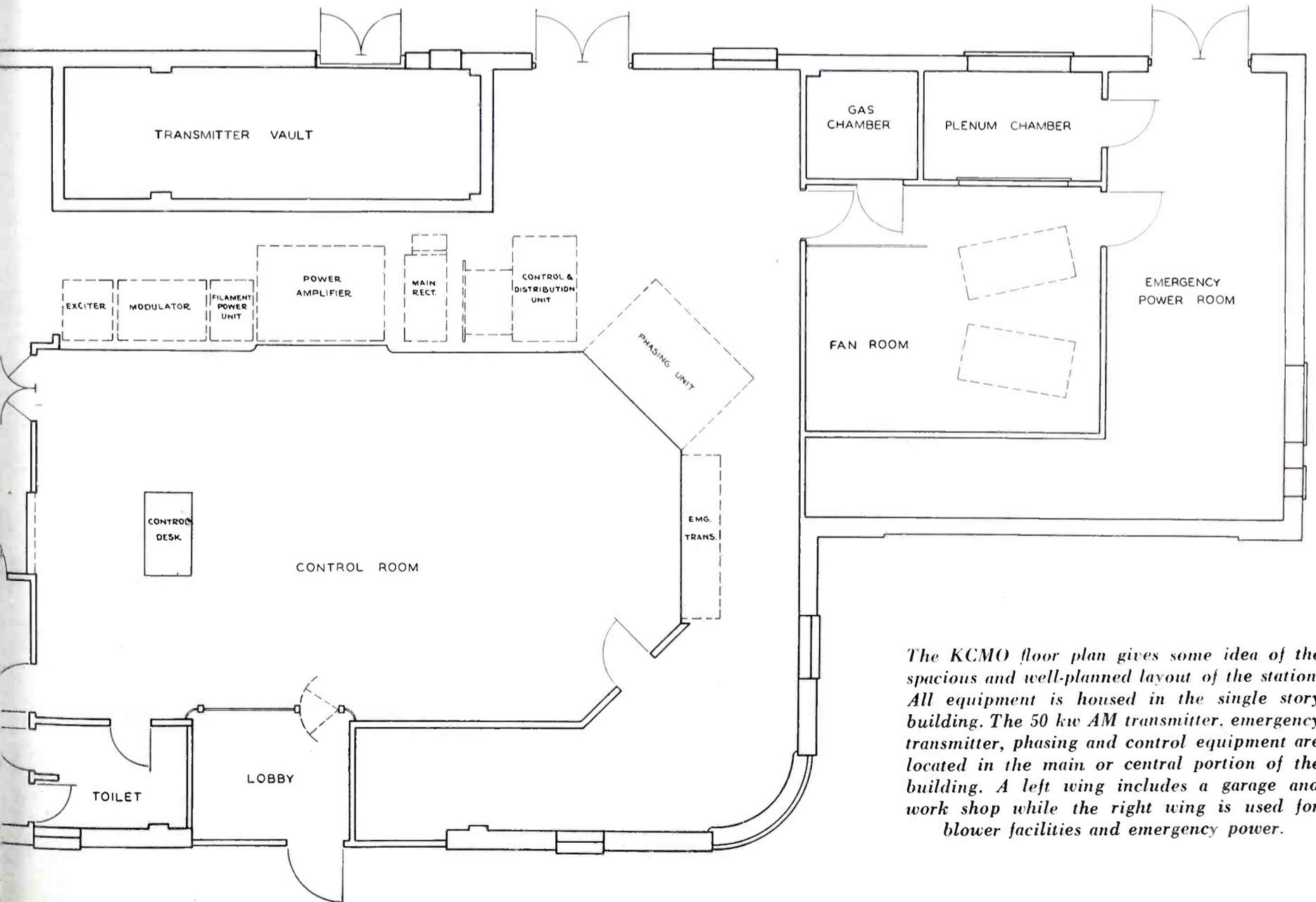
*The KCMO floor plan gives some idea of the spacious and well-planned layout of the station. All equipment is housed in the single story building. The 50 kw AM transmitter, emergency transmitter, phasing and control equipment are located in the main or central portion of the building. A left wing includes a garage and work shop while the right wing is used for blower facilities and emergency power.*
