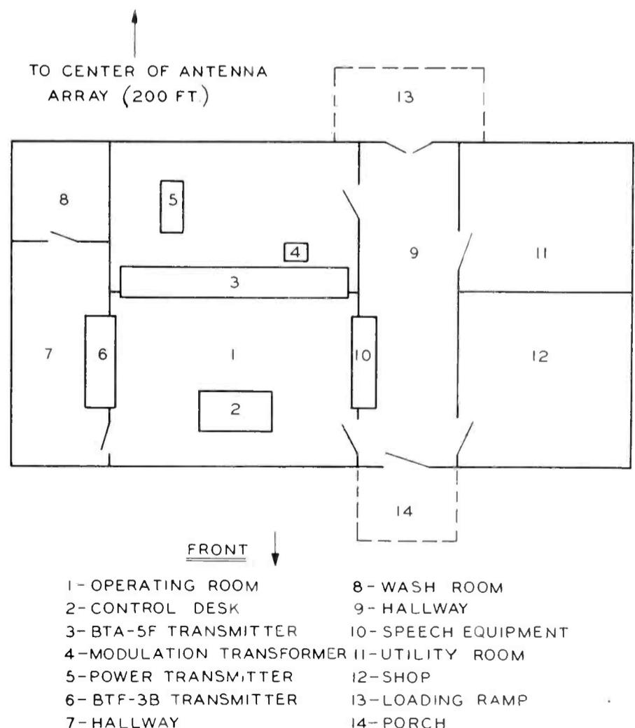
**FIG 3.** Floor Plan diagram of WLOS and WLOS-FM. The control console for the AM and FM transmitters is located so that the operator has full vision of and access to all equipment required for normal operation.
