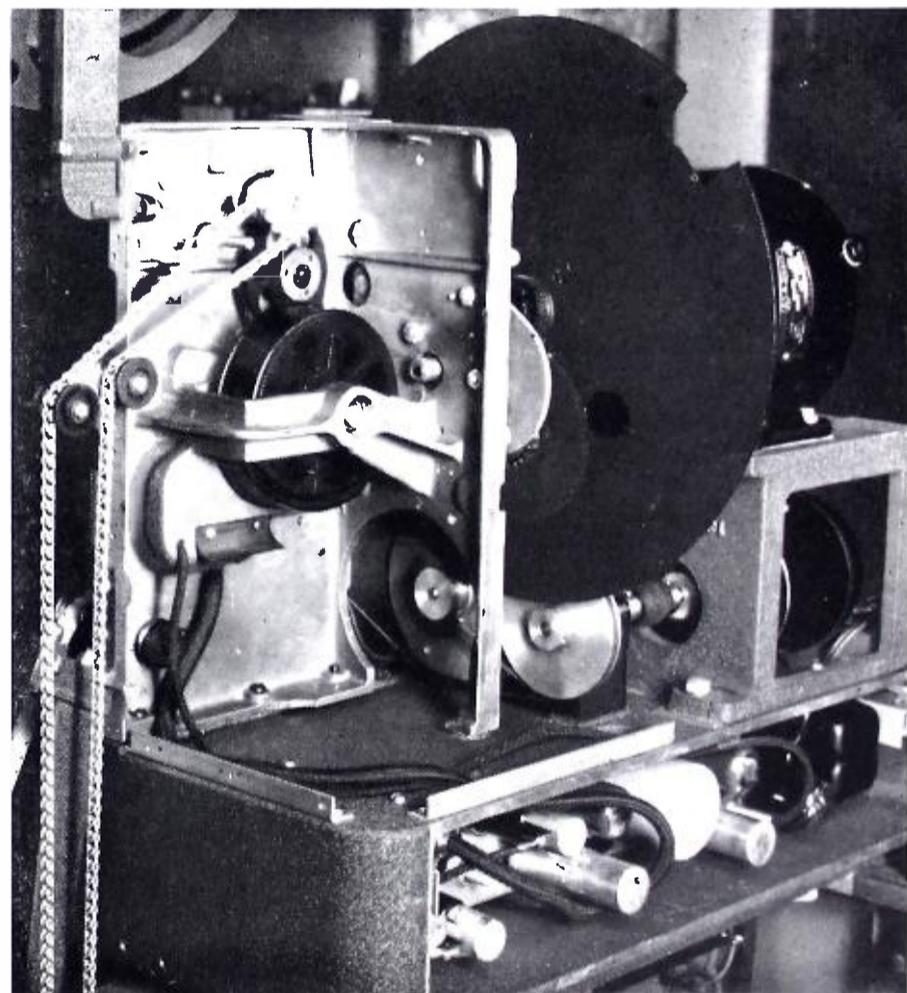
**FIG. 5.** This photograph, with projector cover removed, shows details of shutter and drive. The small motor beneath the main drive motor operates a blower which ventilates the lamp house. The RCA-developed rotary stabilizer used on the sound take-off drum is in the foreground.
