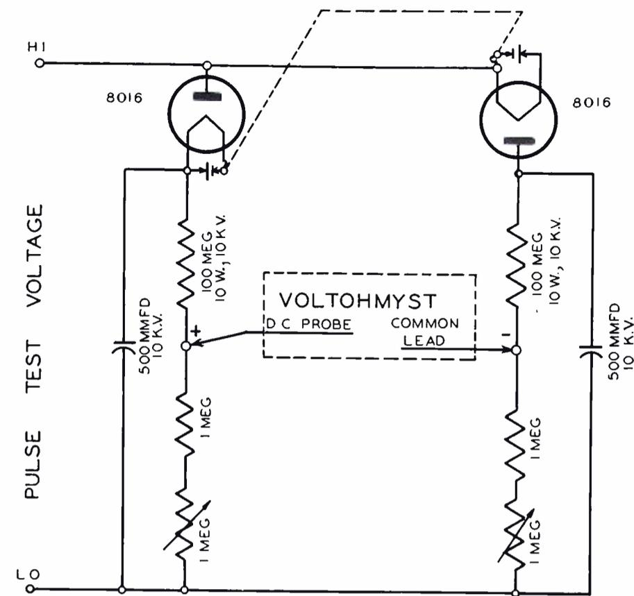
*Schematic diagram of Adapter showing hookup with Model 195-A VoltOhmyst.*
