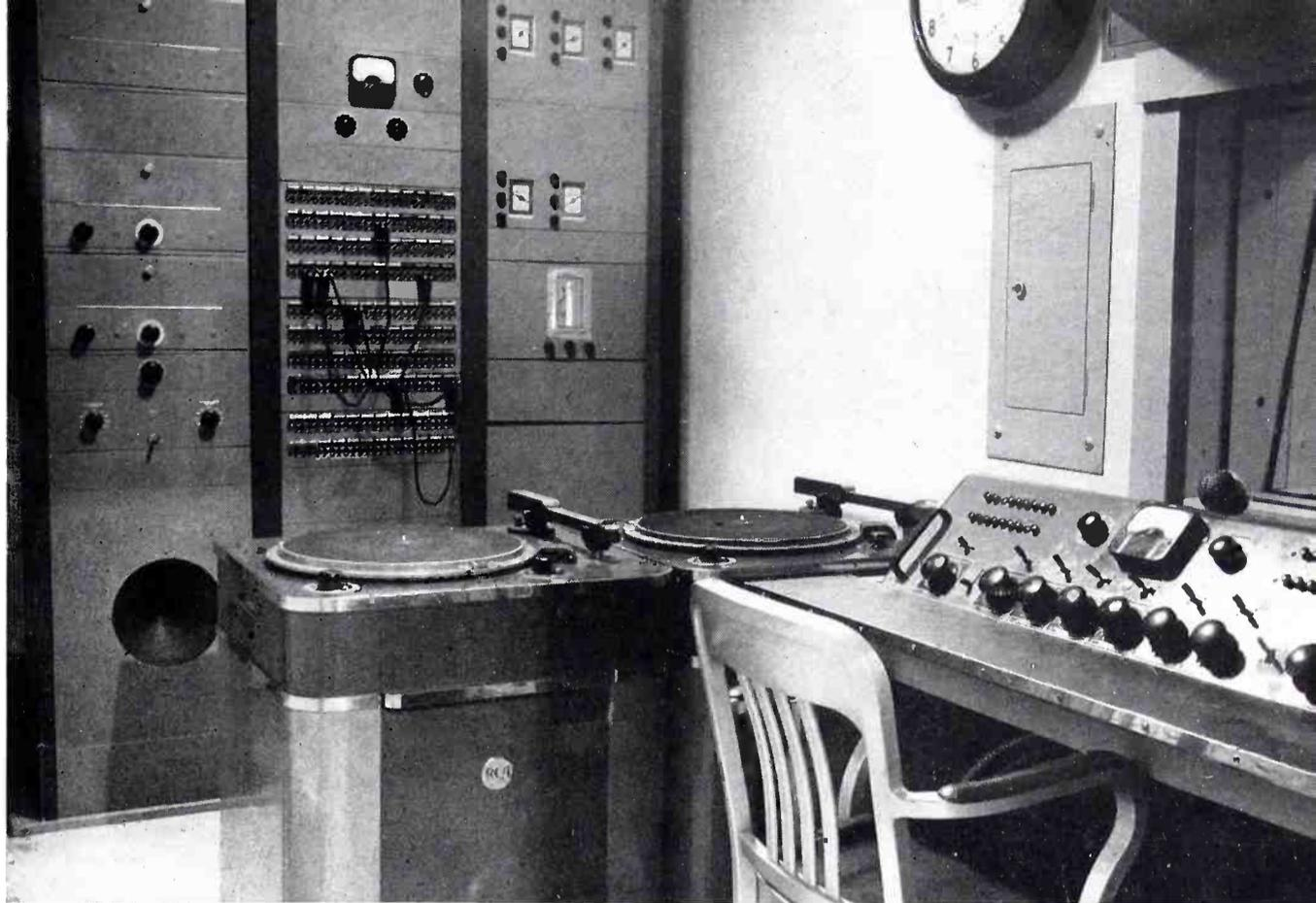
solettes were modified so that positions #3 and #4 accommodate both turntables and microphones. With either of the keys in the left position the turntables are connected. With the keys in the right position the studio microphones are connected. This increases the usefulness of the consolettes immeasurably.
