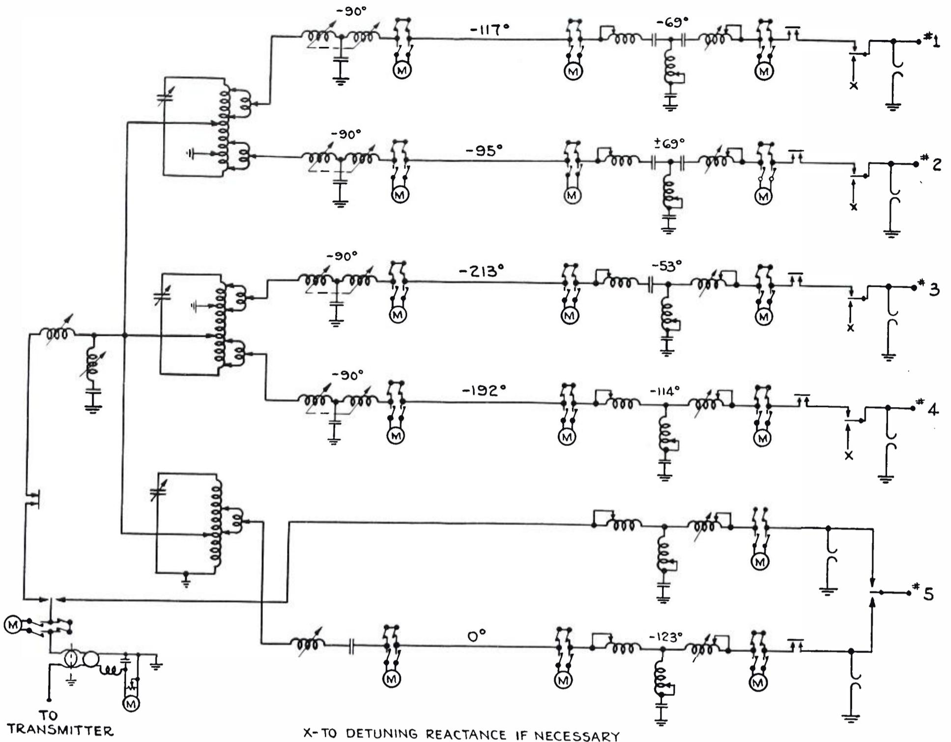
**FIG. 15.** Schematic diagram of the five-tower Phasing and Power Dividing networks which are located in the center tuning house of the new WGAR installation. For daytime non-directional operation, the center (No. 5) tower only is used. Switching of power circuits, as well as monitor circuits, is accomplished from the main transmitter building by means of remote control circuits which, for simplicity, are not shown here.
