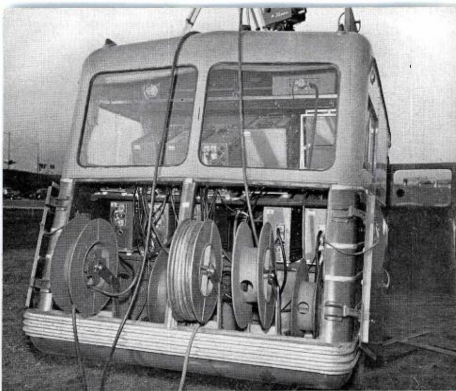
**FIG. 7.** (left) Rear view of unit showing how cable reels can be pulled out to facilitate unreeling. Inner end of cable extends through hole in reel to receptacle on camera control units on the operating table just above.
