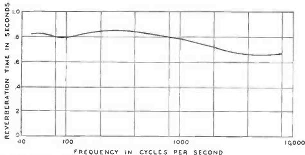
FIG. 2. Reverberation time-frequency characteristic of the test room.
