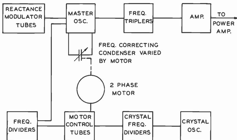
FIG. 9. This is a block diagram of the exciter unit in the BTF-250A Transmitter at WSHS. Operation and adjustment are described in the text.
