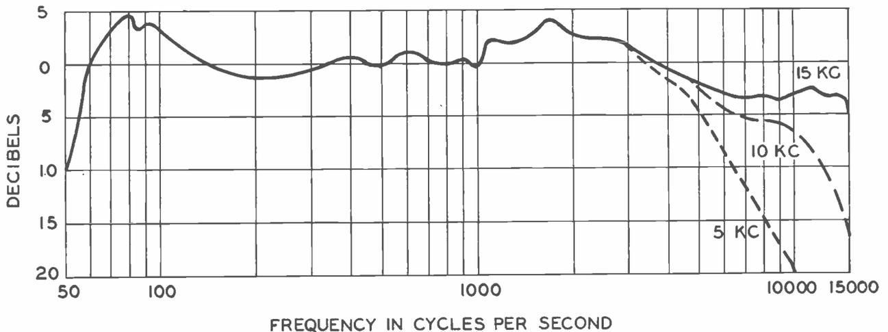
FIG. 7. Frequency response of the LC-1A Speaker (mounted in cabinet) for the three settings of the H-F Attenuator.
