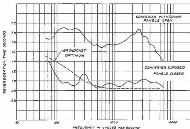
FIG. 4. Reverberation time-frequency characteristics.
