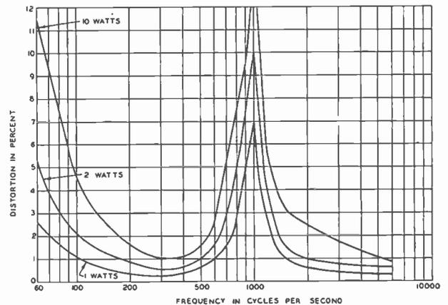
FIG. 6(b). Shown here are distortion curves for a typical "coaxial" type speaker of conventional design. Use of a cross-over filter causes high distortion in the cross-over frequency region. In the LC-1A this is avoided by elimination of the filter, a single condenser being used instead.
