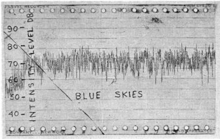
FIG. 9. Instantaneous sound intensity level diagram for a portion of "Blue Skies," which was one of the numbers used.
