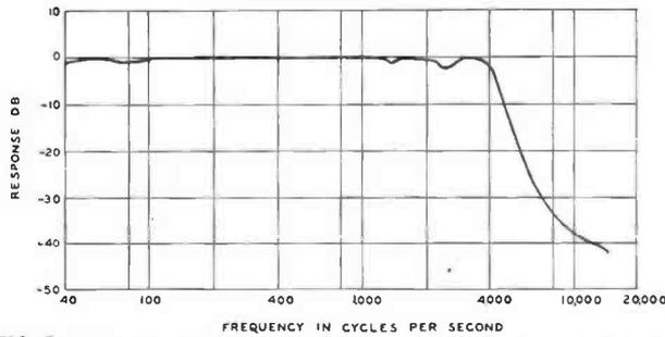
FIG. 6. The response-frequency characteristic of the acoustical filter.
