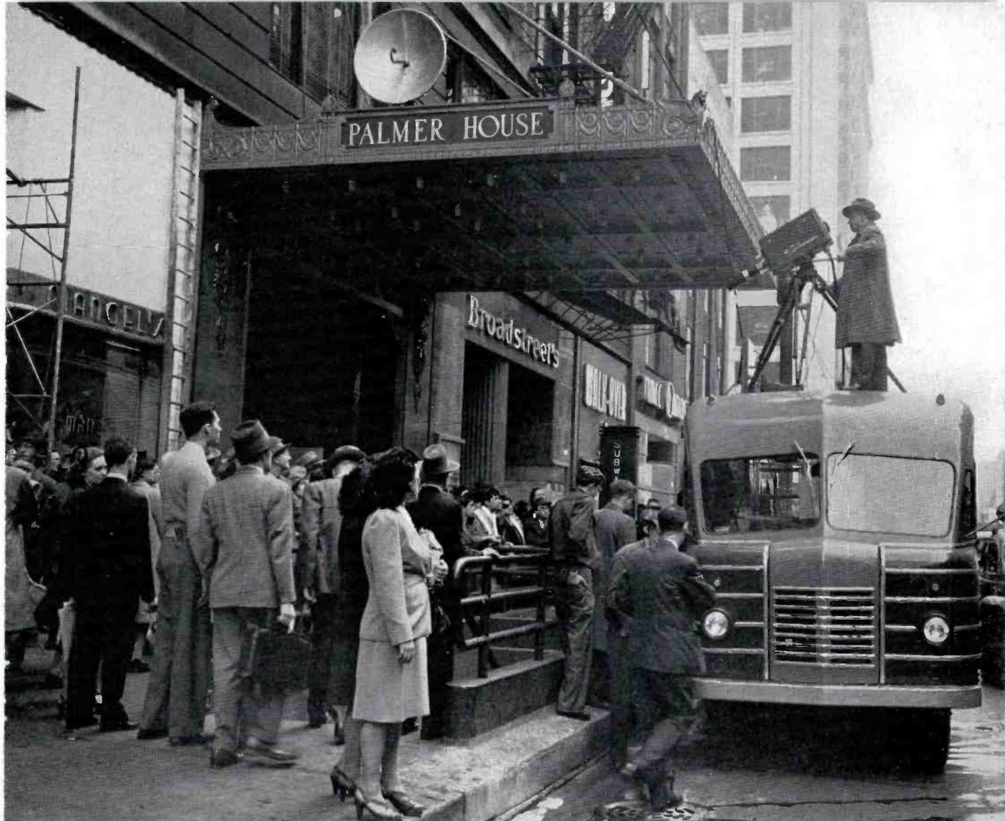
**FIG. 2.** *The TJ-50A Mobile Unit on State Street, Chicago. Standard relay transmitter may be mounted on roof of unit or anywhere within 400 feet. In this view it is placed on hotel marquee for sending video signals to receiver at WBBK on State-Lake Building, three blocks north.*
