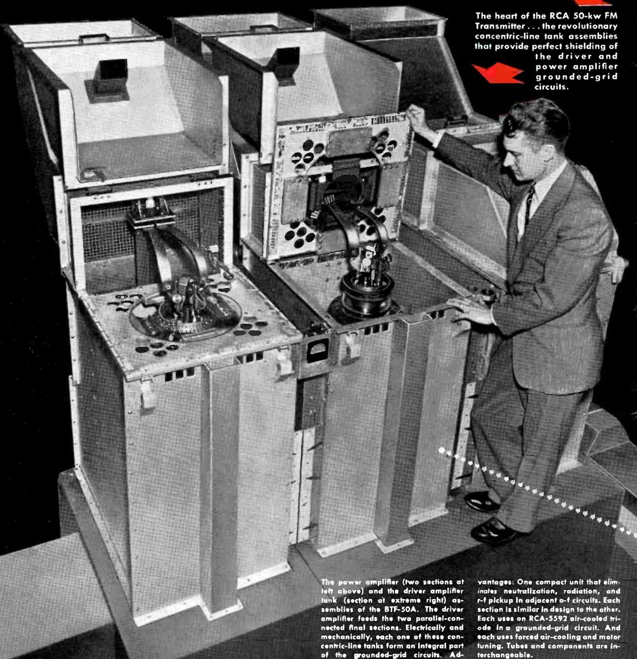
The heart of the RCA 50-kw FM Transmitter... the revolutionary concentric-line tank assemblies that provide perfect shielding of the driver and power amplifier grounded-grid circuits.
