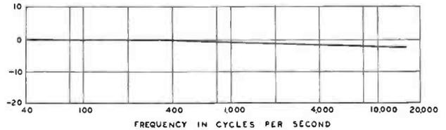
FIG. 8. Response-frequency characteristic of the cloth curtain. Loss introduced by this curtain is negligible.
