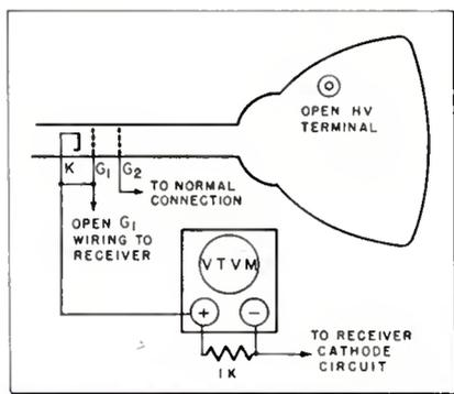
Fig. 2—Connections for CRT emission test.
