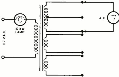
**Fig. 3.** Basic test which you can make to identify power transformer windings using an a.c. voltmeter.
