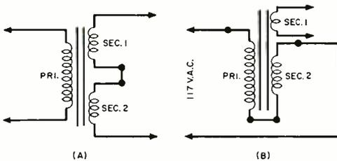
**Fig. 4.** Two tricks to use in making emergency substitutions: (A) two filament windings can be connected in series to supply higher voltages; (B) a filament winding can be connected in series with the primary to lower all secondary voltages.
