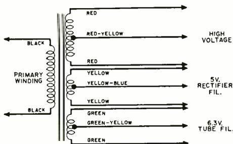
50 ma. This transformer has a standard primary winding and a secondary winding delivering 350 volts *on each side* of its center tap; rated secondary current is 50 milli-amperes. The secondary winding could also be described as 700 volts—CT, 50 ma.
